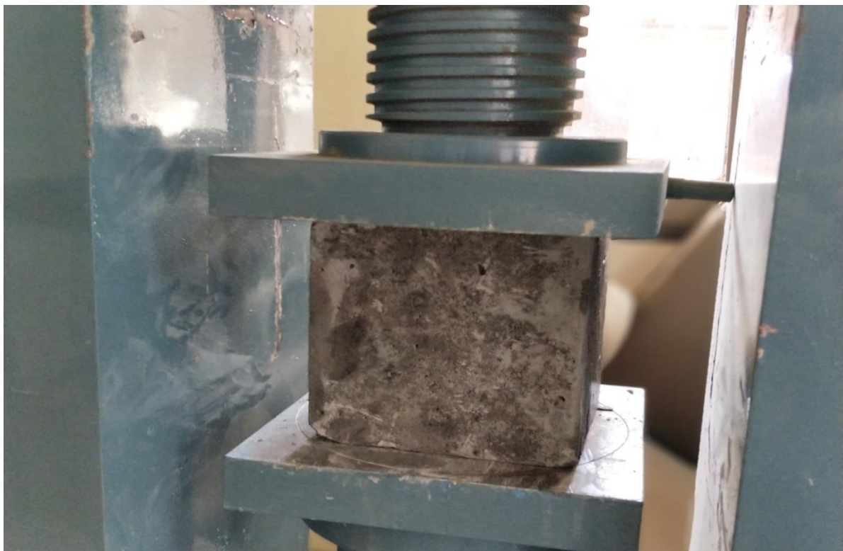
Fig.5.5 Testing of cubes
