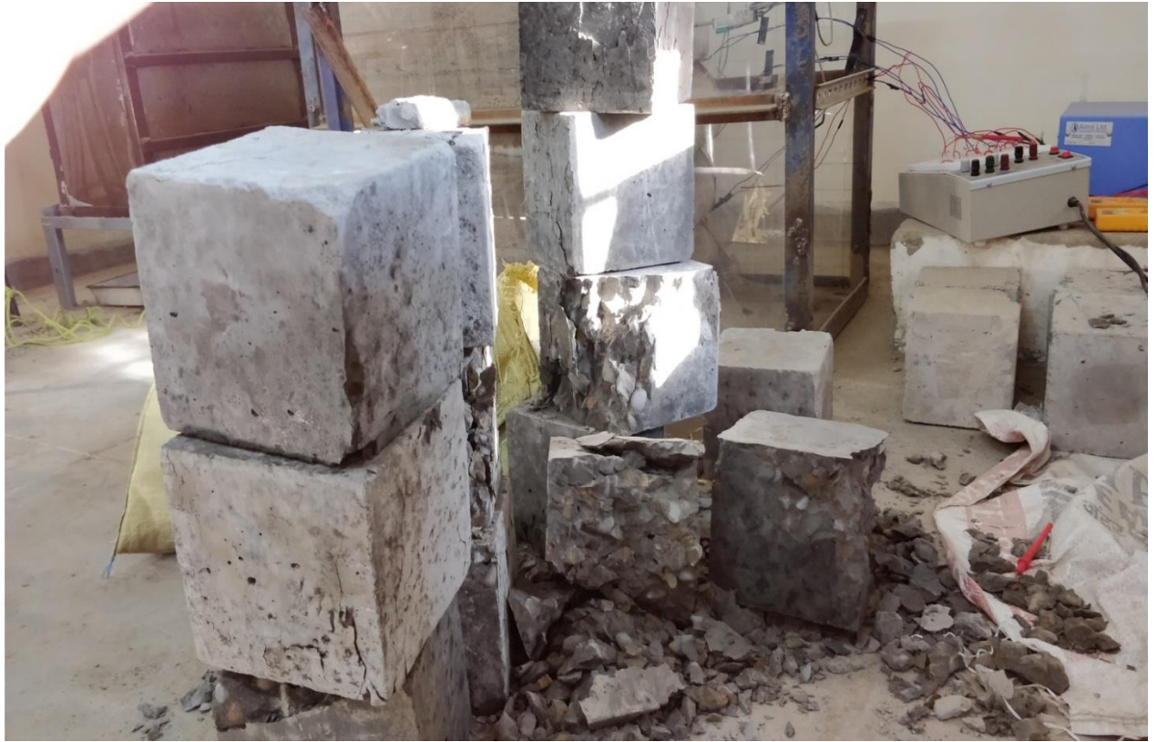
Fig.5.6 Testing of cubes
