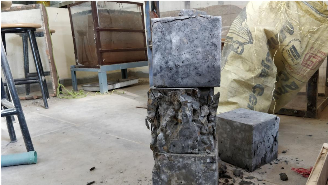
Fig.5.4 Testing of cubes
