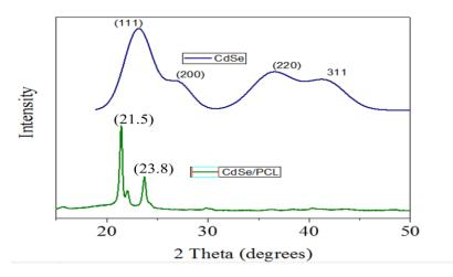
Figure 4.4 XRD results of CdSe4 above one and CdSe4/PCL below one
