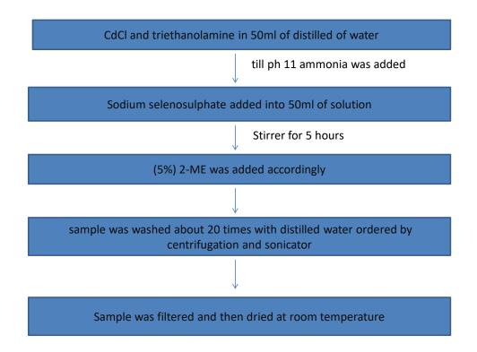
Figure 3.1 Flow chart of synthesis of CdSe4 QDs
