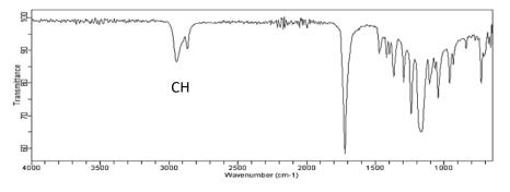
Figure 4.7 Standard peak of PCL polymer C=O results
