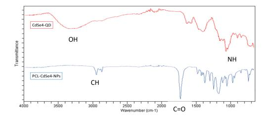
Figure 4.8 FTIR results of CdSe4 in above and CdSe4/PCL below
