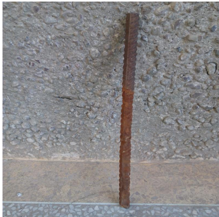
Fig 4.13 Retrieved simple bar dipped in NaCl solution
