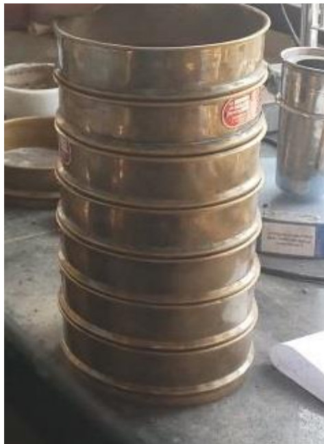
Fig. 3.5 Sieve analysis of sand
