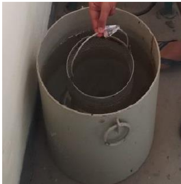
Fig.3.4 Water absorption and specific gravity test of aggregate
