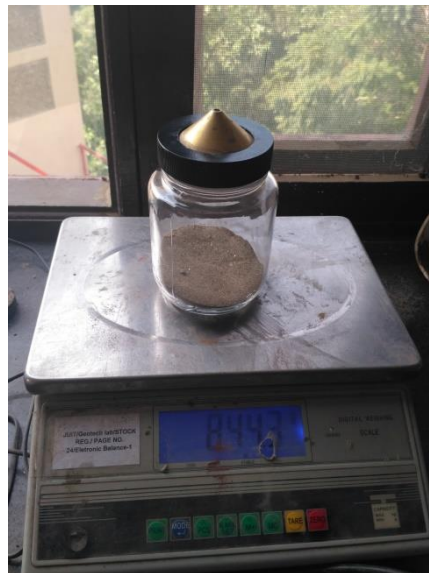
Fig.3.6. specific gravity of sand
