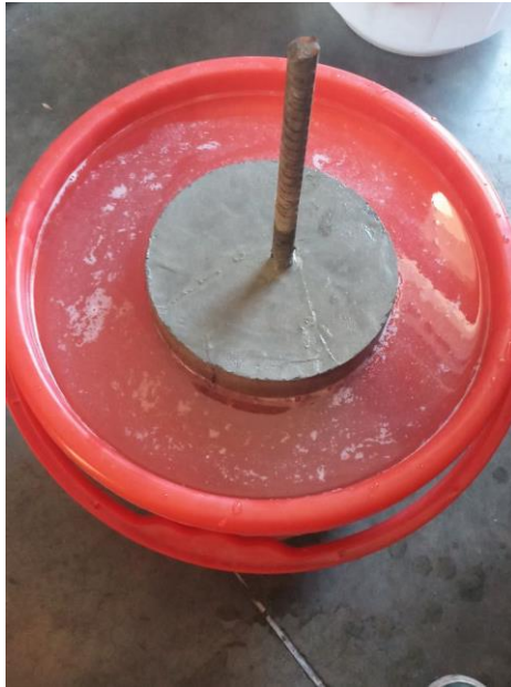
Fig.4.2 Specimen kept in NaCl solution for 24 hours
