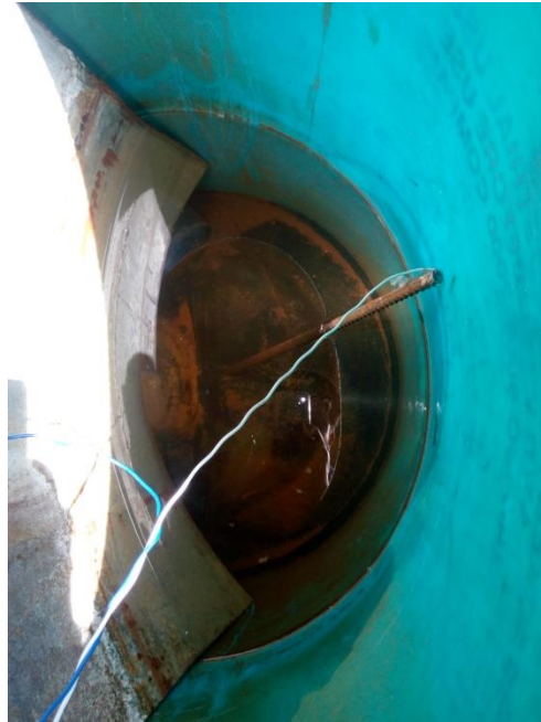
Fig. 4.6 Experimental setup of simple bar dipped in NaCl solution
