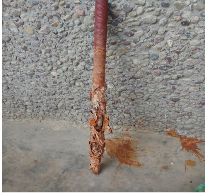
Fig 4.12 Retrieved inhibitor coated bar
