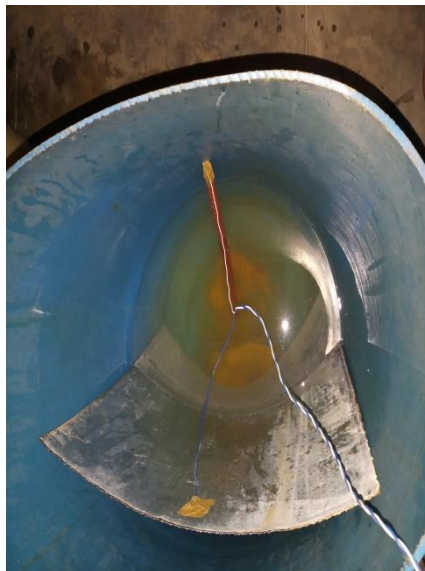
Fig.4.8 Setup for inhibitor coated bar
