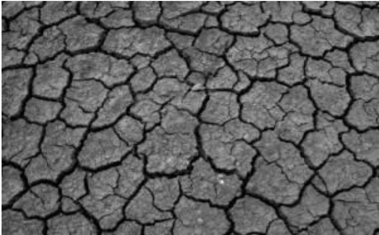
Fig 1 Cracking in black cotton soil
