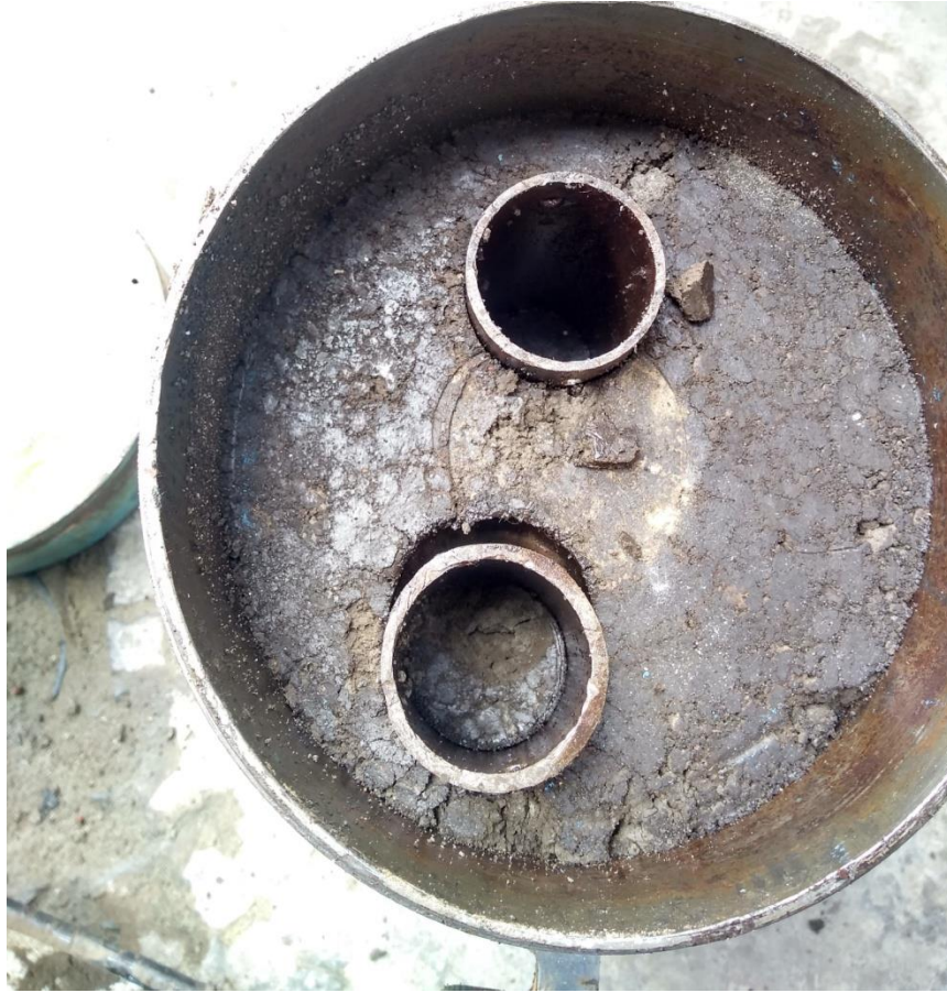
Fig 9 Extraction of UCS sample from Standard proctor
