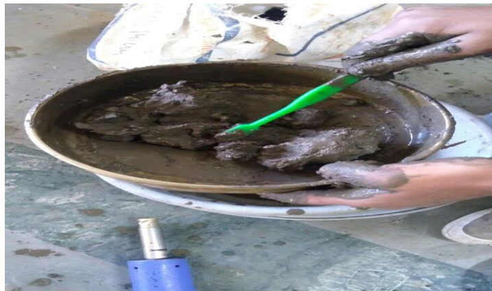
Fig 12 Preparation of sample for hydrometer analysis
