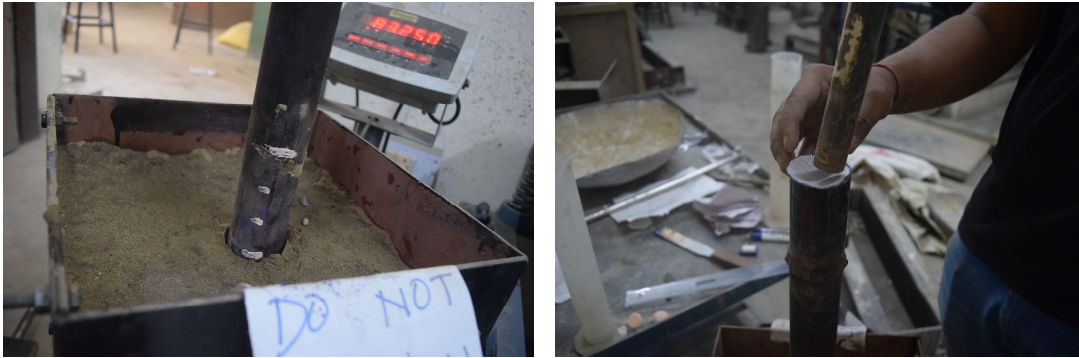
Fig 3.14 (a) Casting the column while inserting the discs and simultaneously pulling out the pipe
