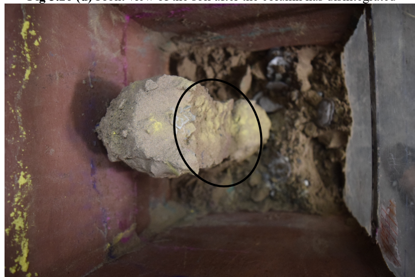
Fig 3.20 (e) Top view of the soil after the column has disintegrated
