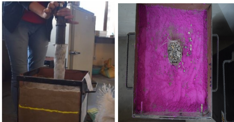
Fig 3.11 (b) Tamping the aggregates
