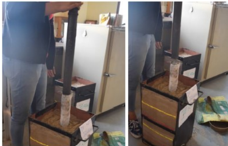
Fig 3.11 (a) simultaneously withdrawing the pipe while filling in the aggregates
