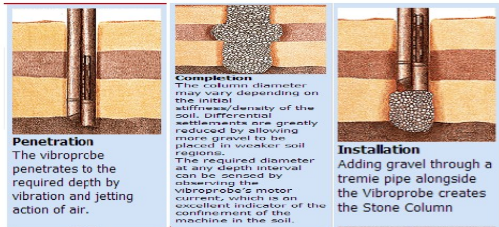
Fig. 1.2 Displacement Method for stone column installation ( Naik, 2013)
