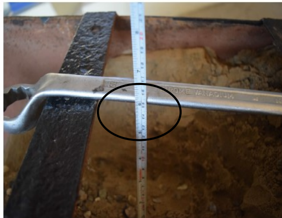
Fig 3.18 (b) Perpendicular distance between the bottom of the column and the wall of the model tank
