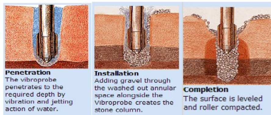
Fig. 1.1 Replacement Method for stone column installation ( Naik, 2013)
