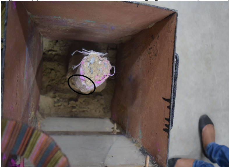
Fig 3.19 (b) Excavated stone column (top view)
