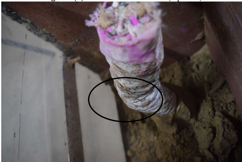
Fig 3.19 (c) Excavated stone column with bulging at the neck (side view)
