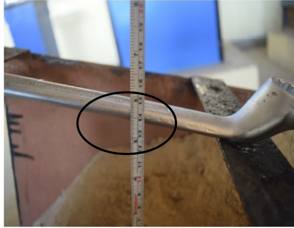
Fig 3.18 (a) Perpendicular distance between the neck of the column and the wall of the model tank
