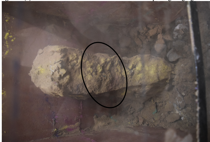
Fig 3.20 (d) Front view of the soil after the column has disintegrated
