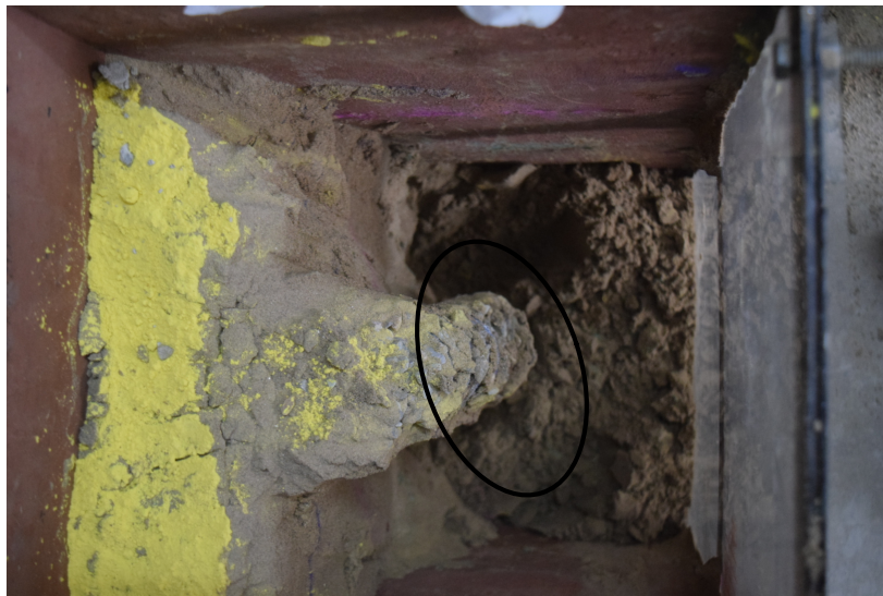
Fig 3.20 (b) Top view of the column after excavation depicting bulging at neck
