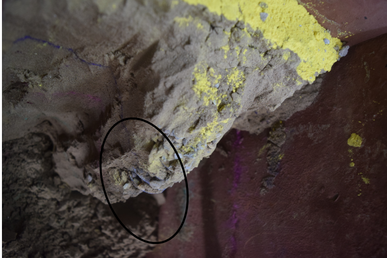
Fig 3.20 (c) Side view of the column after excavation depicting bulging at neck
