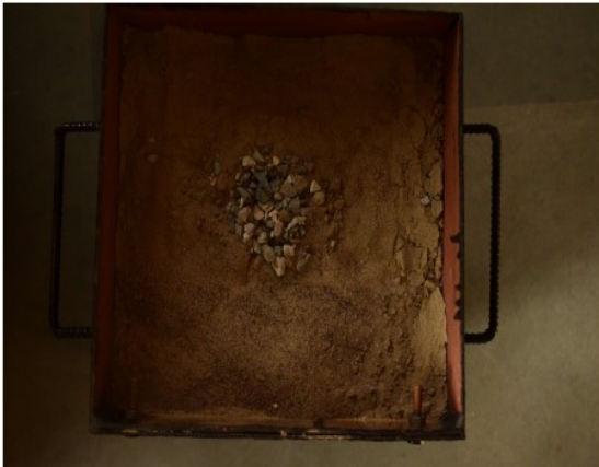
Fig 3.16 (a) Unreinforced column before settlement
