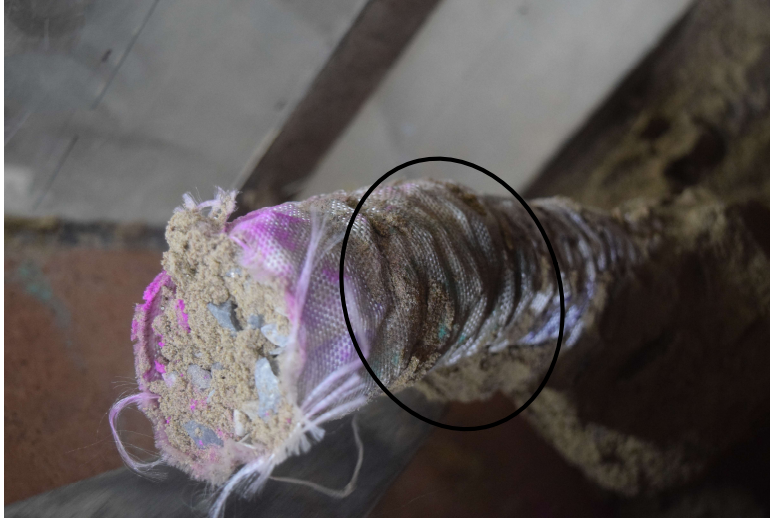
Fig 3.19 (a) Excavated stone column with bulging at the neck (side view)
