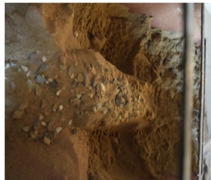
Fig 3.17 Excavated unreinforced stone column
