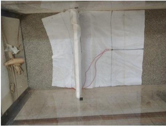
(a) Placement of Geotextile Layer
