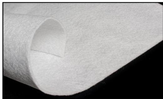
Figure 1.4 (b) Non-Woven Geotextile
