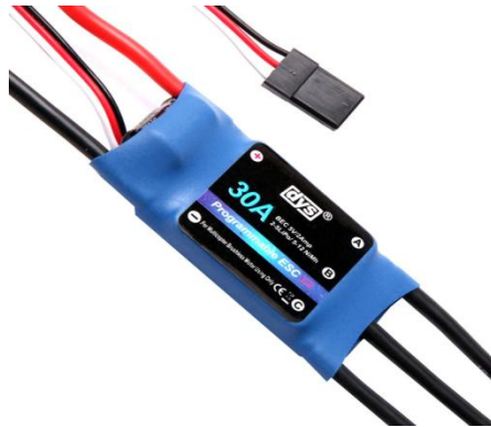
Figure 19: Programmable Electronic Speed Controller (25 Amps)
