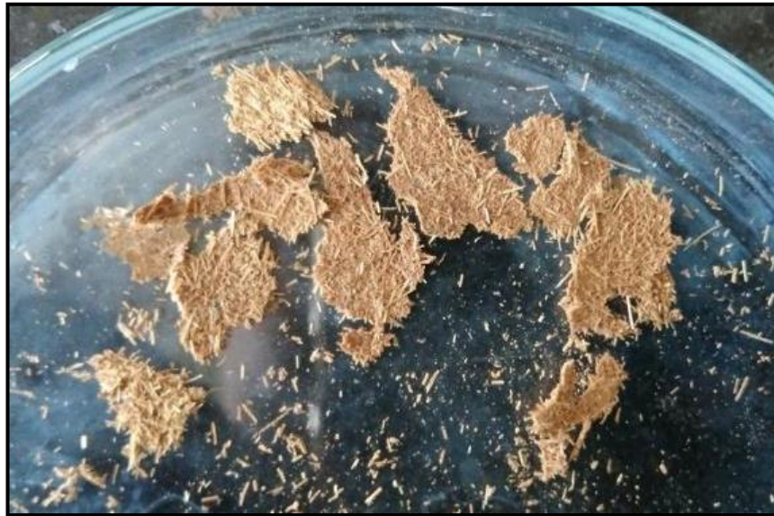
Figure.4.11 – Some level of binding in Pine needle powder with Acacia gum
