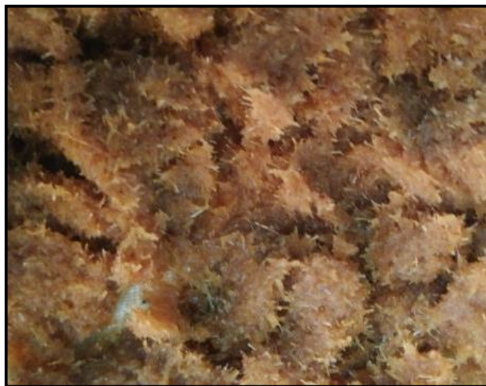
Figure.4.3- Pine needle powder after first NaOH treatment
