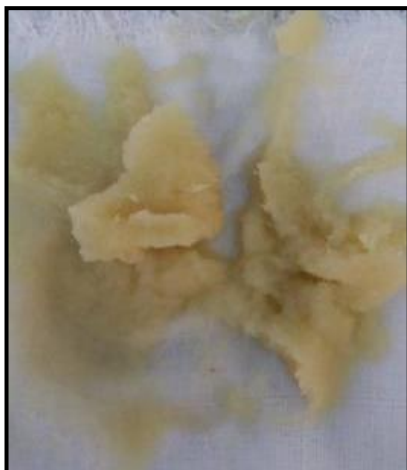
Figure.4.4- Freshly isolated MFC from pine needles after last NaOH treatment
