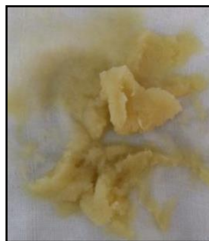
Figure.4.4- Freshly isolated MFC from pine needles after last NaOH treatment
