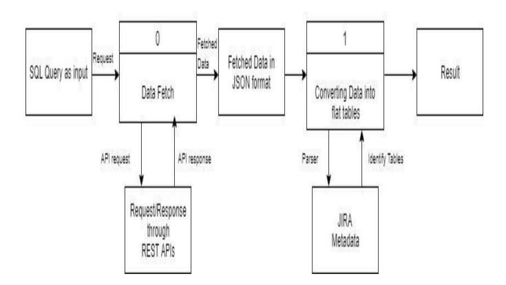
Figure 3.4 Level-0 Data Flow Diagram of the JIRA ODBC Driver
