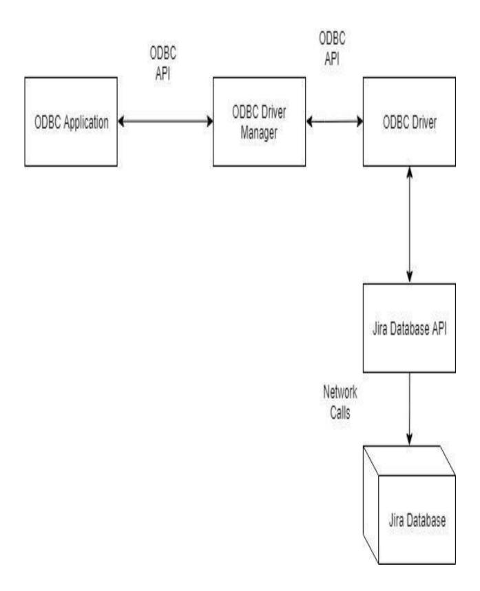
Figure 3.1: shows the system architecture of JIRA ODBC Driver
