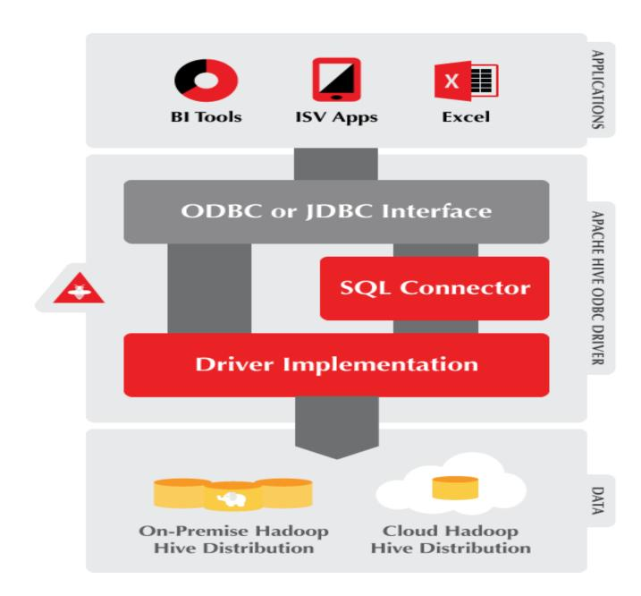
Figure 3.2: shows the High level design of the driver
