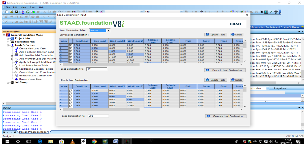
Figure 18-Input window for generation of load combination
