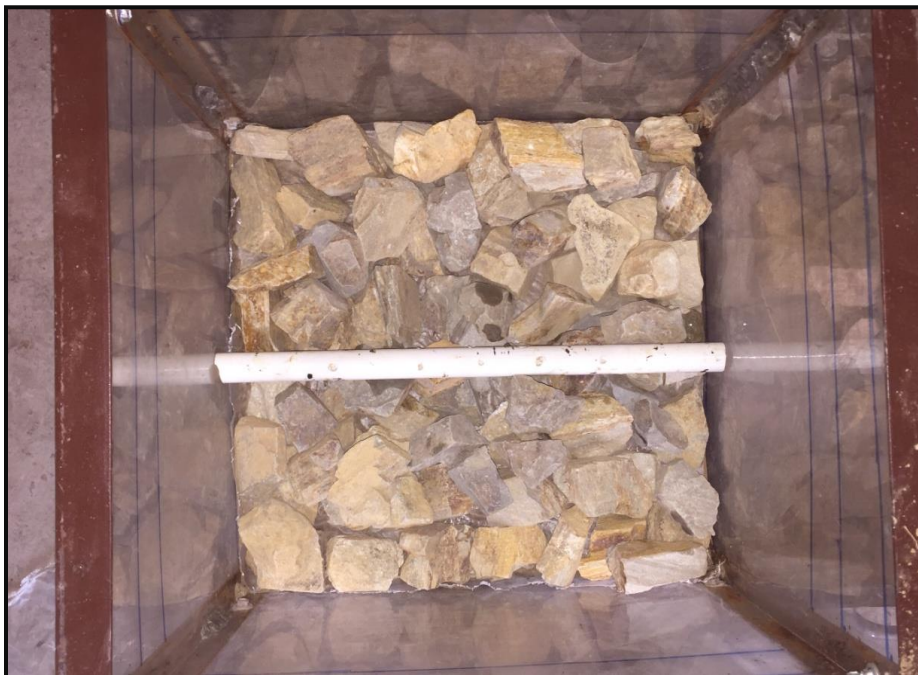
Stone reservoir with water outlet pipe
