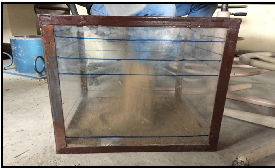
Filling of Uncompact Soil Layer
