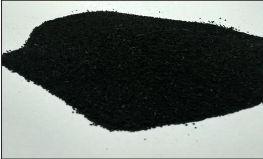
Figure 3.1:- Crumb Rubber mesh - 40
