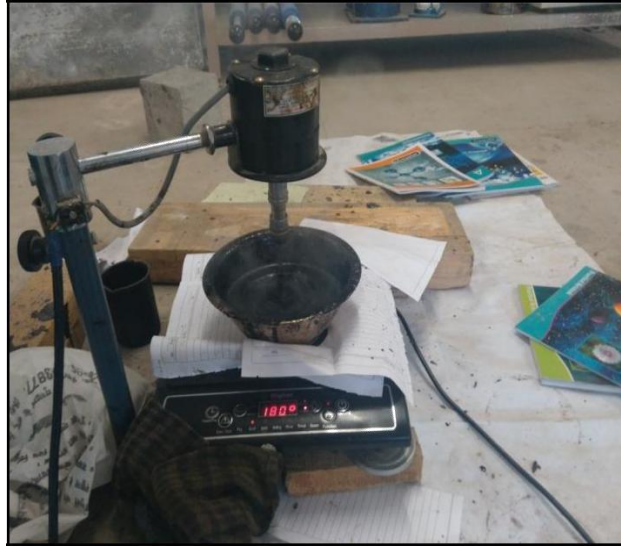
Figure 3.2:- Mixing of crumb rubber with bitumen
