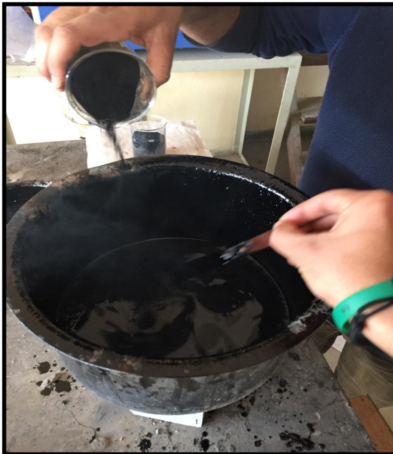
Fig:4.12 Mixing of Crumb Rubber(mesh 40) with bitumen
