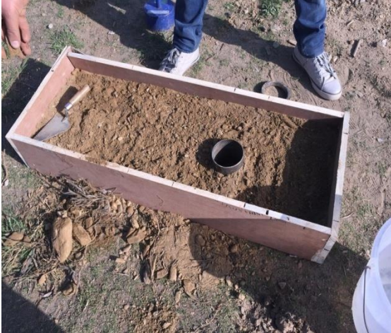
Figure 5.3:- Single Ring Infiltrometer embedded in Test cell.
