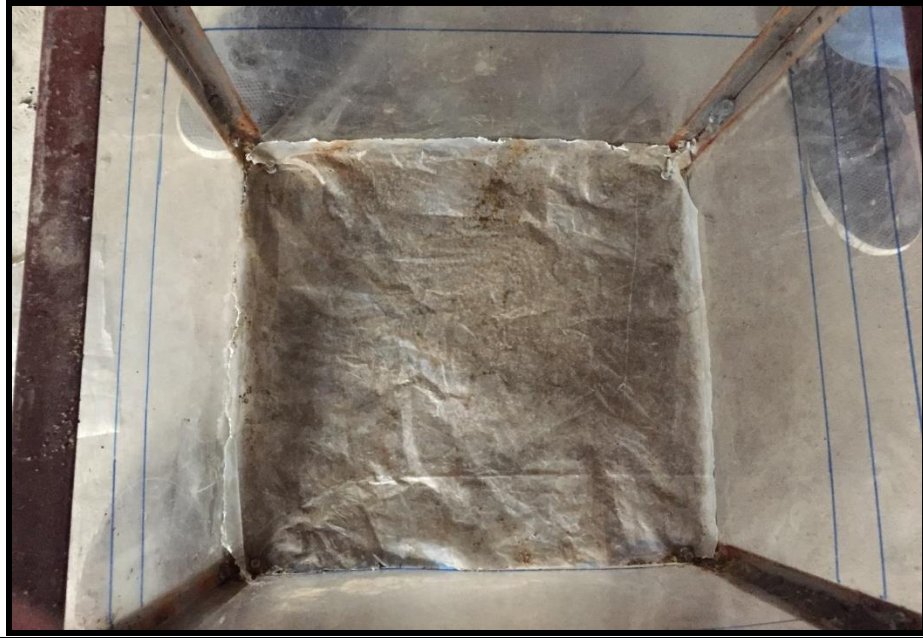
Uncompacted soil layer with water percolating sheet
