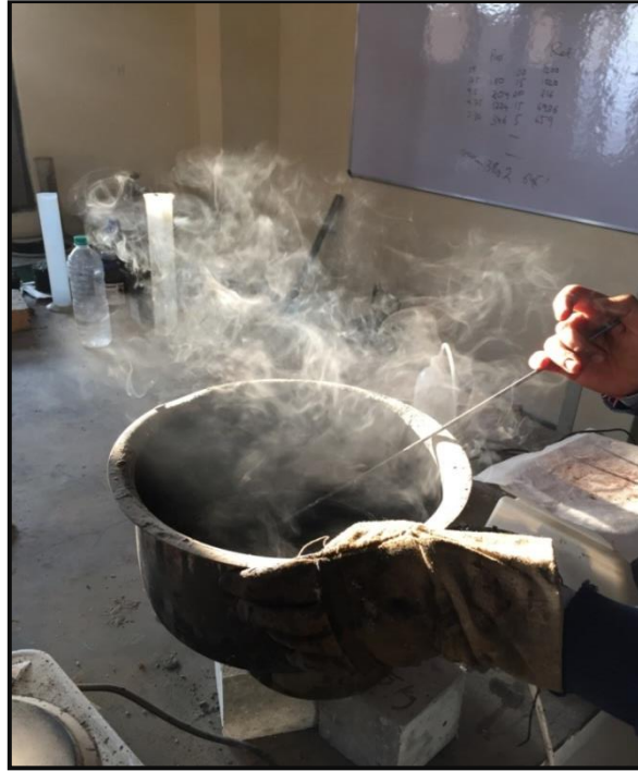
Fig:4.11 Heating of bitumen
