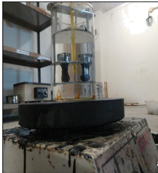
Figure 3.4:- Softening point test
