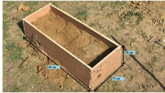
Figure 5.1: Schematic of Test Cell
