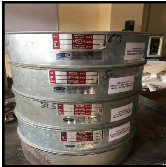
Sieve analysis of aggregates
