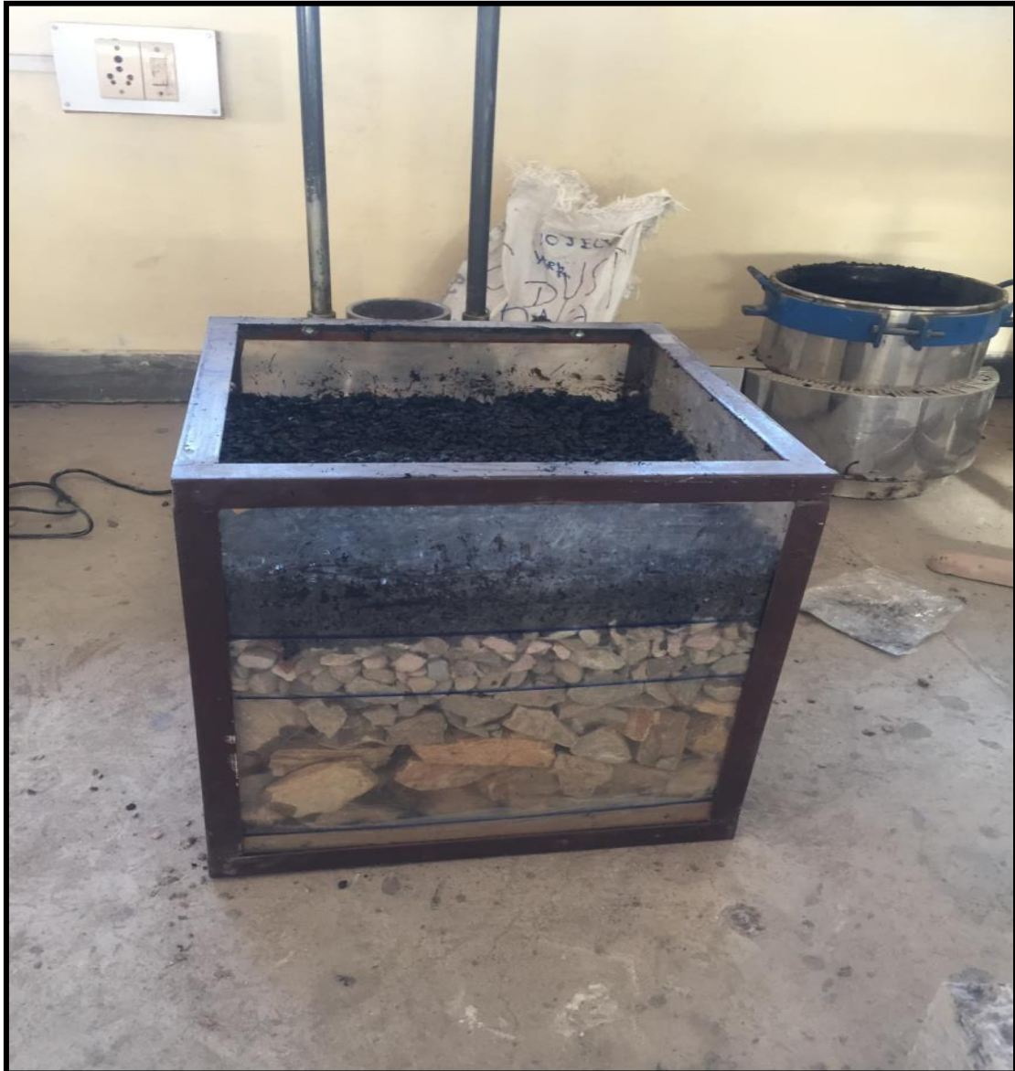
Fig:4.14 Schematic view of Pervious Pavement
