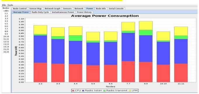
If we analyse both the cases then we can see that the power consumption difference is not too much , it is because of low traffic and low size of packets but still we can see difference at node 4 and node 5. and LPM increases on all the nodes that shows that "Line Per Minute "increases which means now more paths constructed as worst parent attack comes in action because due to attack it takes longest path to transfer the packets .
