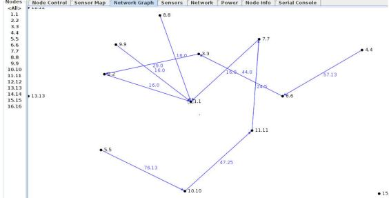
Here in the simulation the sink node is one(1) and the only changes after the attack are in topology path of node 4 and node 5, the numbers on arrow shows the ETX value ,as we can see fromnetwork graph before the attack the ETX VALUE for node 4 and 5 were 29 and 27.65 respectively. But
