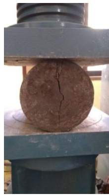
Figure 3.8- Split Tensile testing of Cylinder
