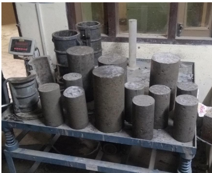
Figure 5.6- Split Tensile Test Samples
