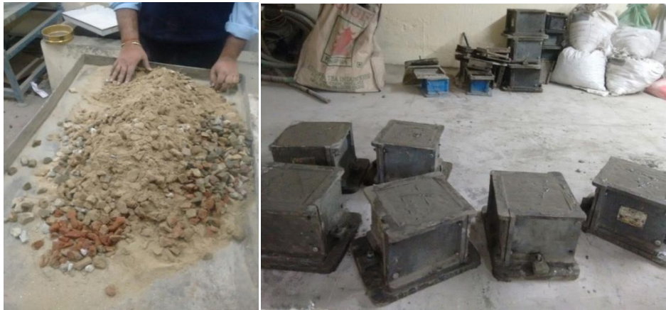
Figure 3.5- Dry mix (left) and concrete mould (right)
