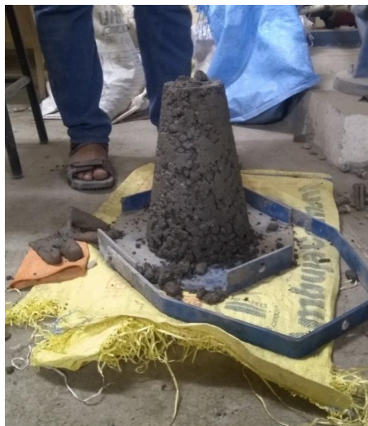
Figure 5.3- Slump cone test
