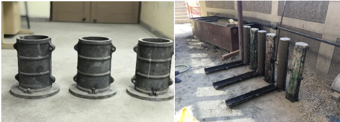
Figure 3.11: mould for casting
