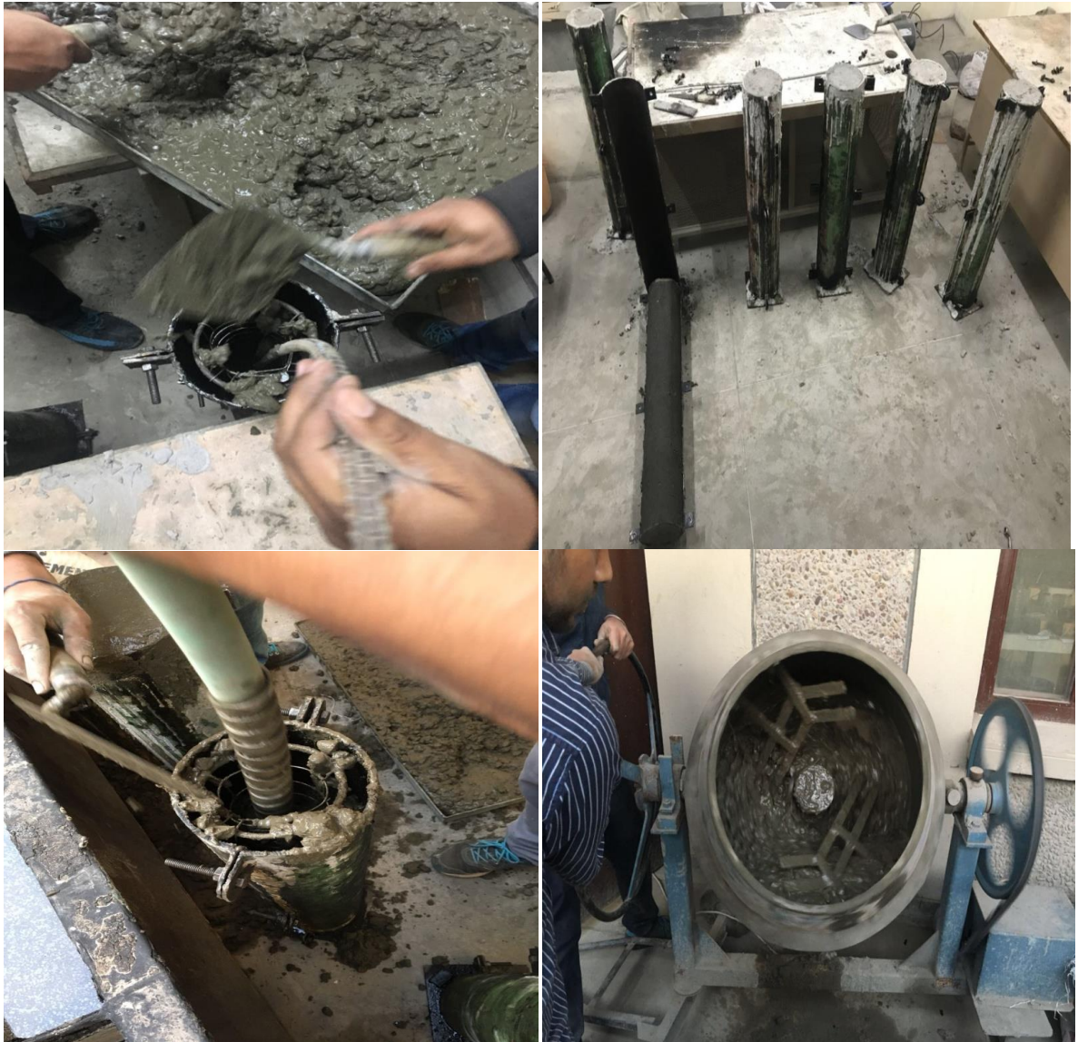
Figure 3.12 Casting of column
