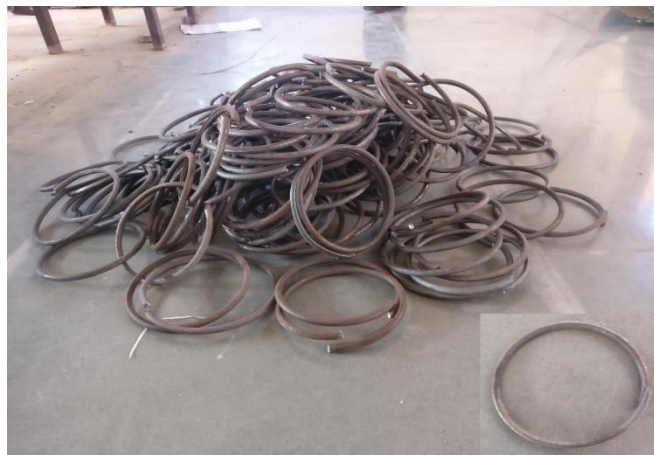
Figure 3.5 Mild Steel Bars Fe 250
