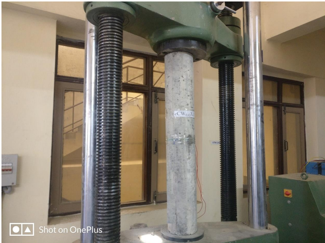
Figure 3.15 testing of column
