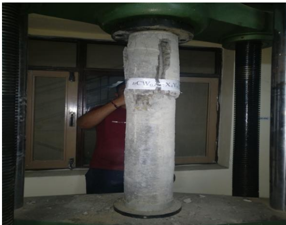
Figure 3.18: Failure of column
