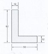
Q.2. Find the collapse load for the given beam.
