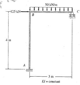
Q.3. Solve the given frame by using approximate method of frame.
