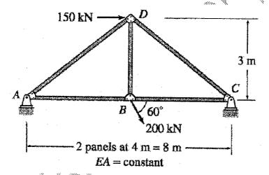
Q.2. Solve the given frame by using Moment Distribution Method.
