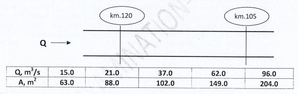
Estimate the travel time through the reach for flows of 17.0m<sup>3</sup>/s and 85m<sup>3</sup>/s
