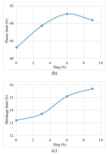
**Fig. 1** Effect of microfine slag on Atterberg limit; (a) on liquid limit, (b) plastic limit, (c) shrinkage limit
