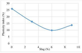
Fig. 2 Change in the plasticity index with microfine slag content
