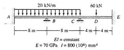
Q.4. Draw the shear force & bending moment diagram and deflection pattern of the given beam.
