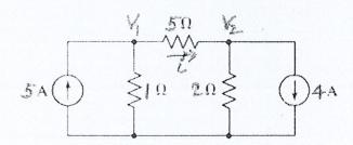
Q.3 Using super position theorem, find the current  $i_x$  in the circuit given below: [(05), CO-1]
