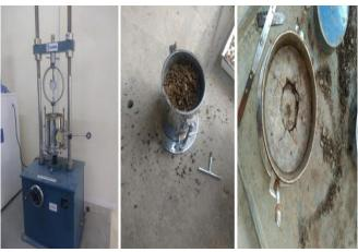
Fig. 5. California Bearing Ratio Test in Laboratory
