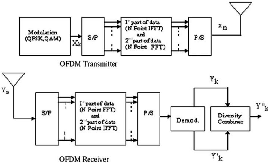
Fig. 1 The system model for the OFDM digital communication systems.
