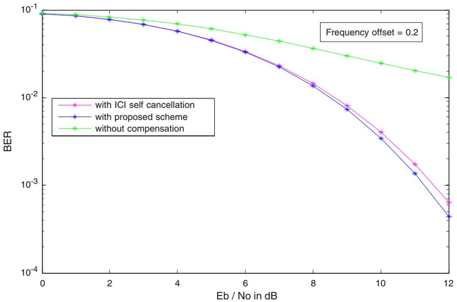
**Fig. 3** Comparison between proposed conjugate ICI cancellation schemes with self cancellation scheme for 16QAM OFDM system.
