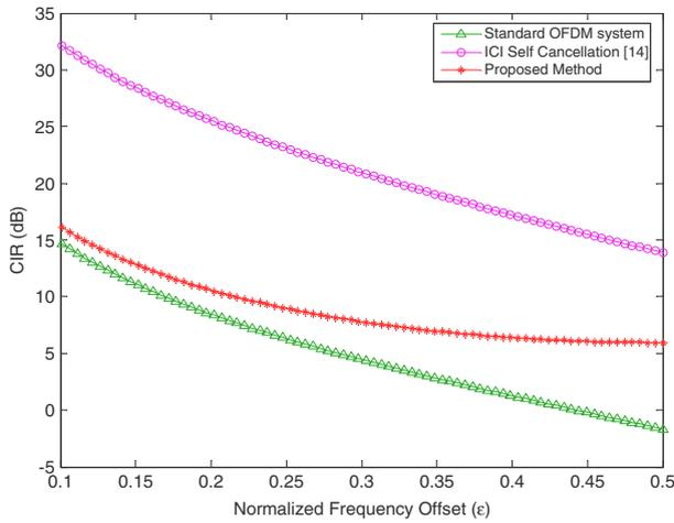
**Fig. 4** Carrier to interference ratio (CIR) versus normalized frequency offset and comparison of the proposed scheme with [14].
