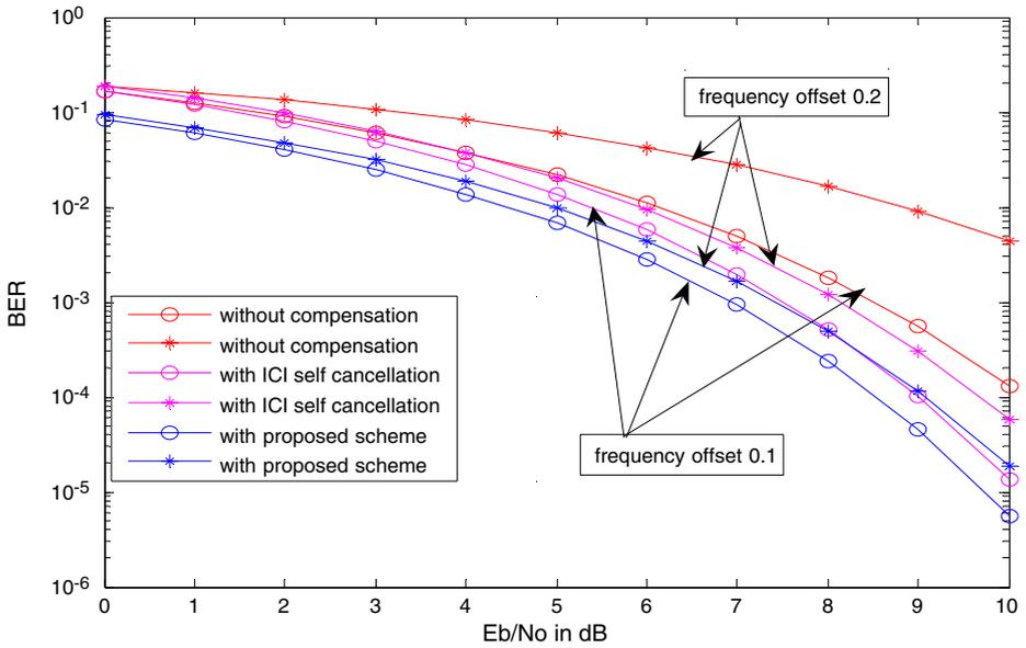
**Fig. 2** Comparison between the proposed improved ICI cancellation schemes with the self-cancellation scheme.
