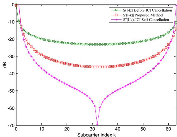
**Fig. 5** Compression of the ICI coefficient before and after cancellation of ICI. It is also compared with [14].
