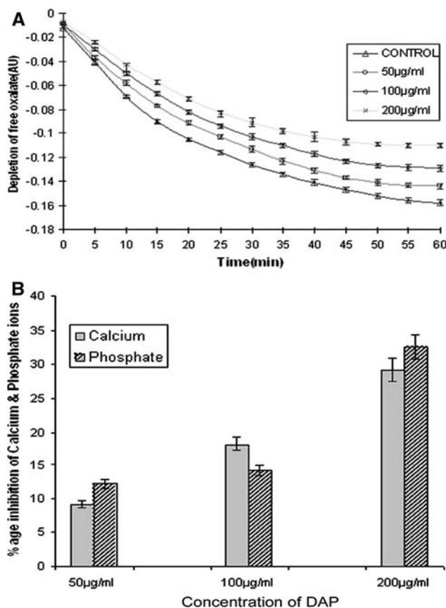
**Fig. 4** **a** The kinetics of the CaOx crystal growth inhibitory activity by DAP at concentrations 50, 100 and 200 μg/ml as compared to control having Millipore water instead of DAP. The inhibitory activity was performed for a longer duration (60 min) to simulate the long term effects of interaction between crystals and DAP (n = 6). **b** Percentage inhibition of calcium and phosphate ions following calcium phosphate crystallization by DAP at concentration 50, 100 and 200 μg/ml (n = 6)
