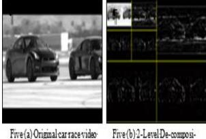
Five(b)2-Level De-composiframe. tion of car race video frame. Fig. 5:Original Car Frames and their Decomposition.
