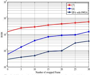
Fig. 9: BER (Log Scale) Under Spatial Attack (Gaussian Noise).
