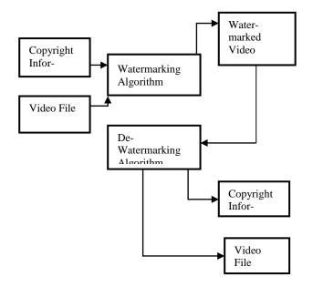
Fig. 1:Block Diagram of Video Watermarking.
