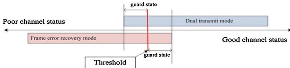
Fig. 5 The mode transition for error adaptive MAC protocol in the distributed cognitive radio network [99]
