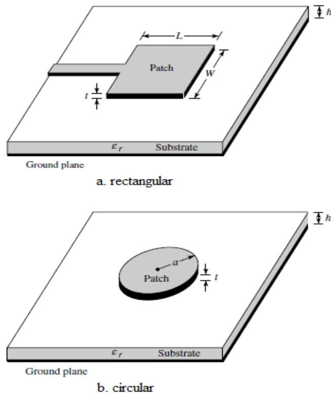
Fig. 1.5 Rectangular and circular microstrip antennas.
