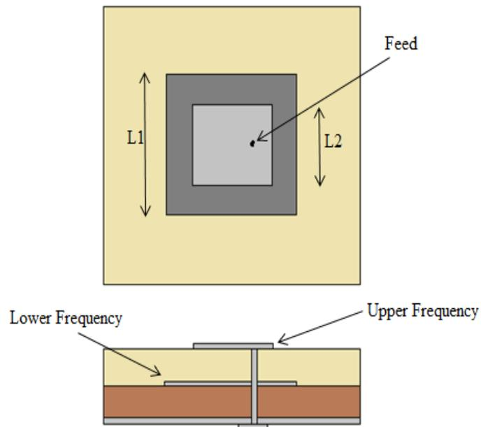
Fig. 3.12. Stacked patches for dual resonance generation.
