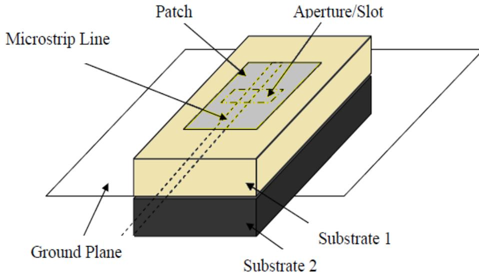
Fig. 2.6. Aperture coupling scheme.
