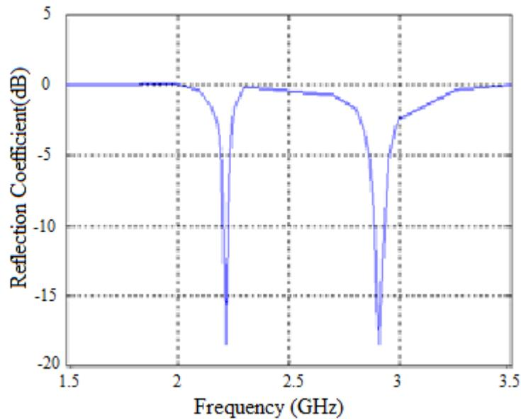
Fig. 4.2. Reflection coefficient of the designed antenna.
