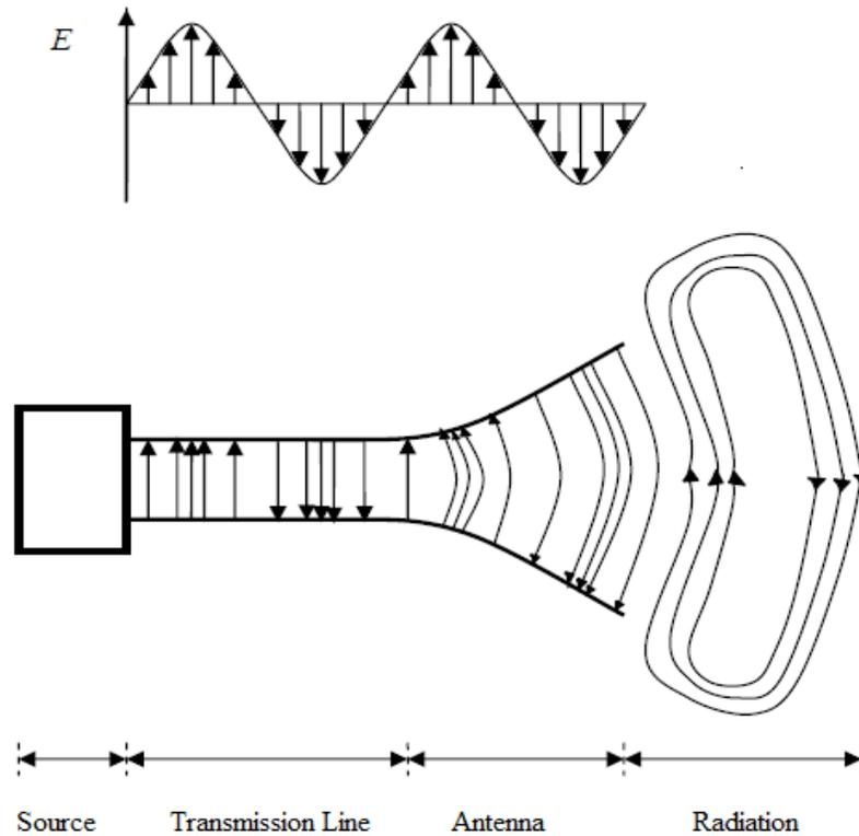
Fig. 1.2 Radiation from an Antenna
