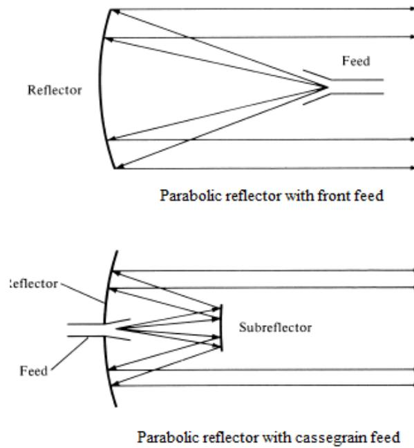
Fig. 1.6. Reflector antenna configurations.
