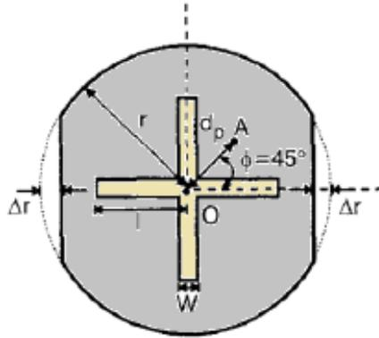
Fig. 3.8. Truncated peripheral edge circular antenna.
