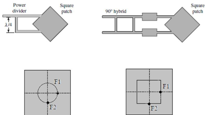
Fig. 3.9. Various dual feed circular polarization generating schemes.
