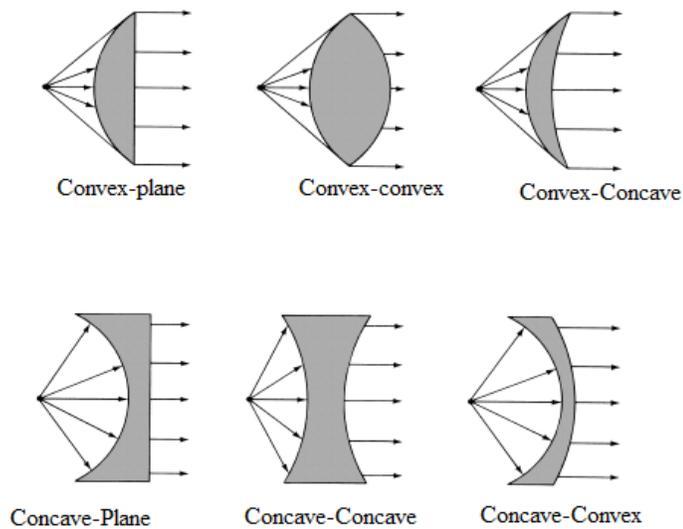
Fig. 1.7 Various lens antenna configurations.
