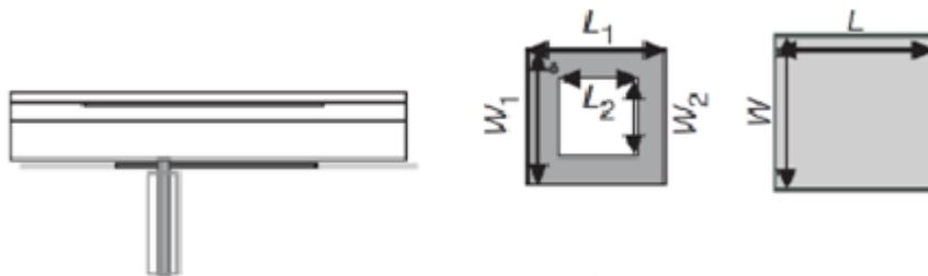
Fig. 3.5 Square ring and square patch stacking.
