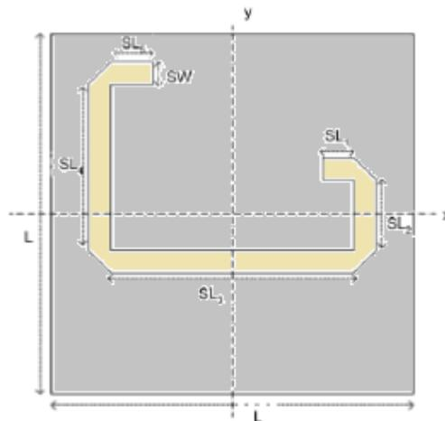
Fig. 3.1. C shaped slot.
