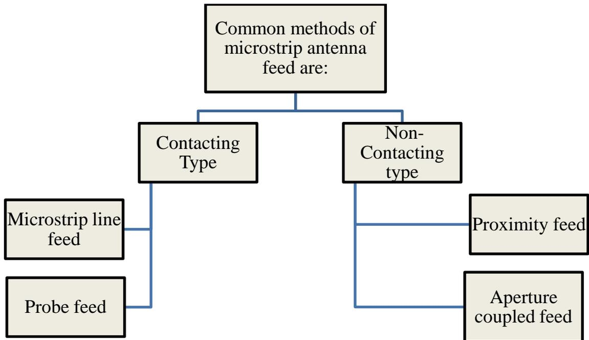
Fig.2.3. Different types of feeding methods.
