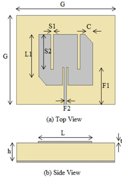
Fig. 5.1 Geometry of the designed antenna.
