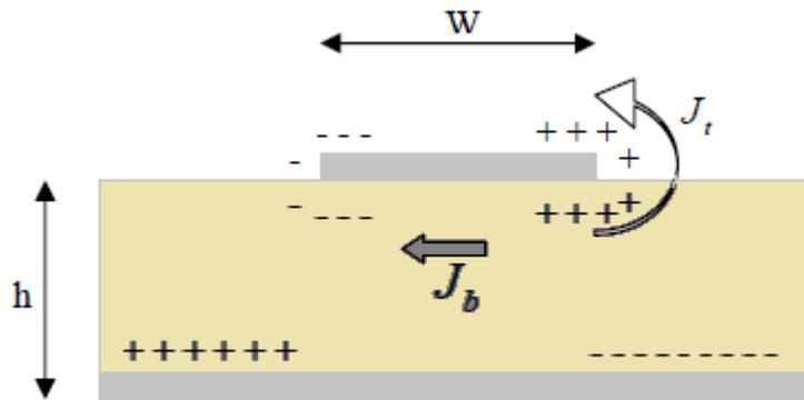
Fig. 2.11. Charge distribution in microstrip antenna.
