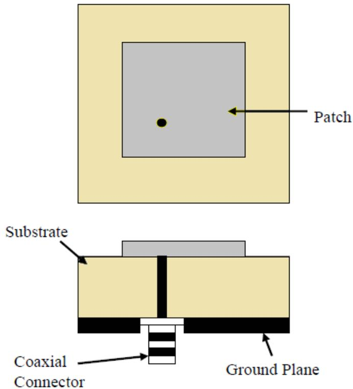
Fig. 2.5. Coaxial feeding method.
