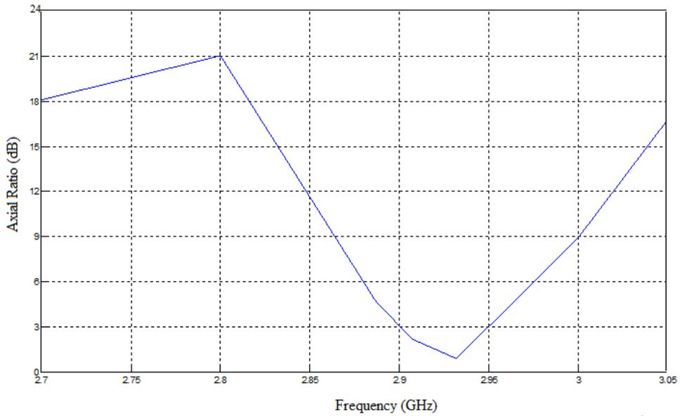
Fig. 4.4. Axial ratio curve for 2.9 GHz resonant frequency.
