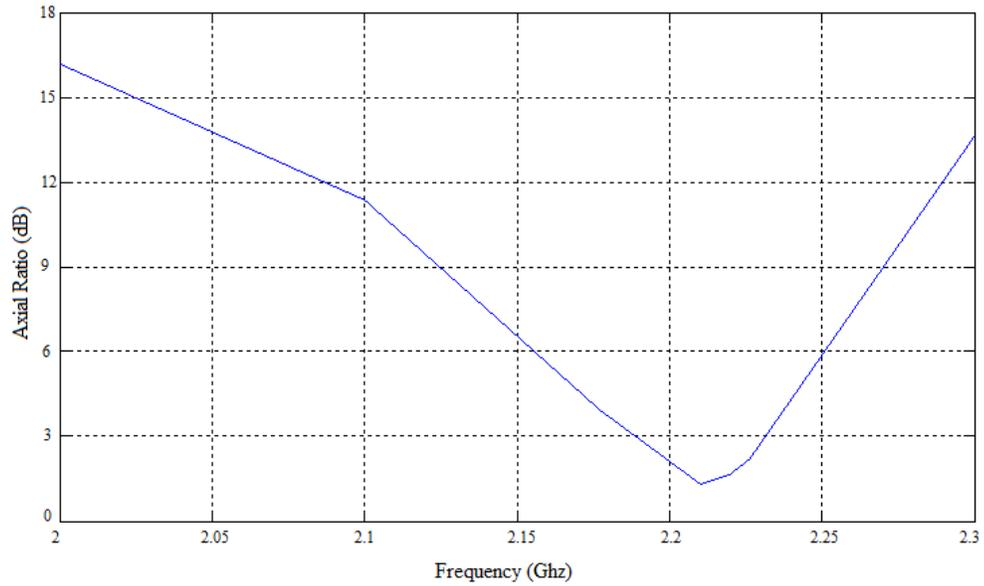
Fig. 4.3. Axial ratio curve for 2.2 GHz resonant frequency.
