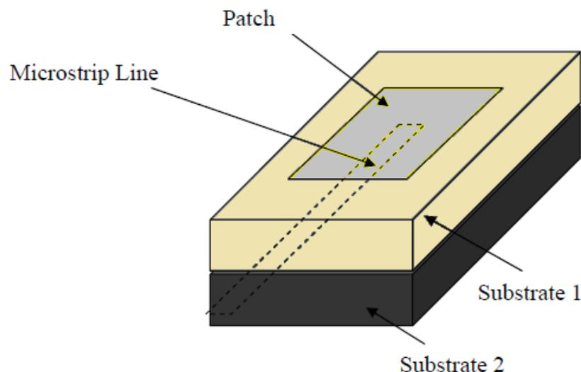
Fig. 2.7. A proximity coupled feeding method.
