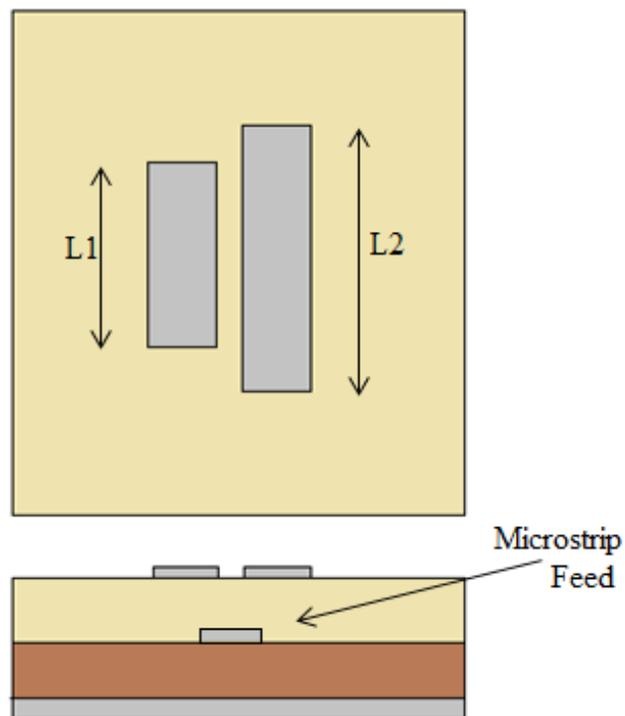
Fig. 3.11. Coupled microstrip dipoles for dual resonance generation.
