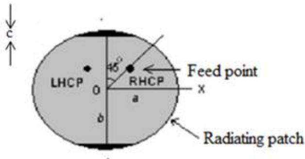
Fig. 3.7. Truncated elliptical patch.
