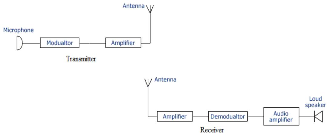
Fig. 1.1 A Basic Wireless Communication System.
