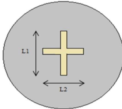
Fig. 3.4. Crossed slot circular patch.
