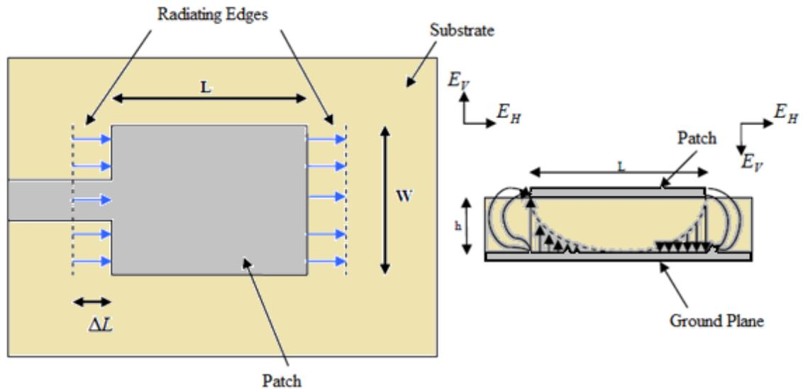
Fig. 2.10. Electric field lines from radiating edges.
