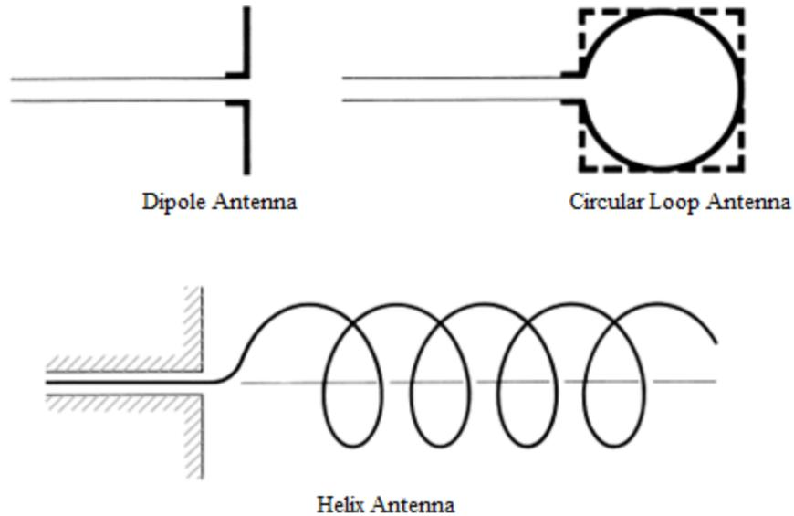
Fig 1.3 Various types of wire antenna configurations.
