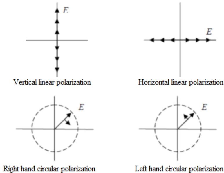
Fig. 1.9. Various polarization schemes.
