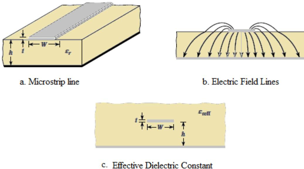
Fig. 2.8. Fringing fields in microstrip antenna.
