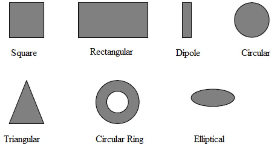
Fig. 2.2. Various shapes of patch element.
