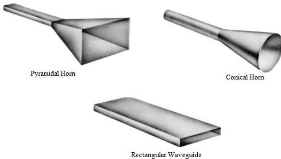
Fig. 1.4 Various aperture antenna configurations.
