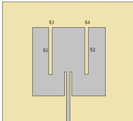
Fig. 3.10. Slots for dual band generation.
