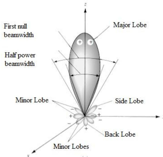
Fig. 1.8. Radiation pattern of a directional antenna.
