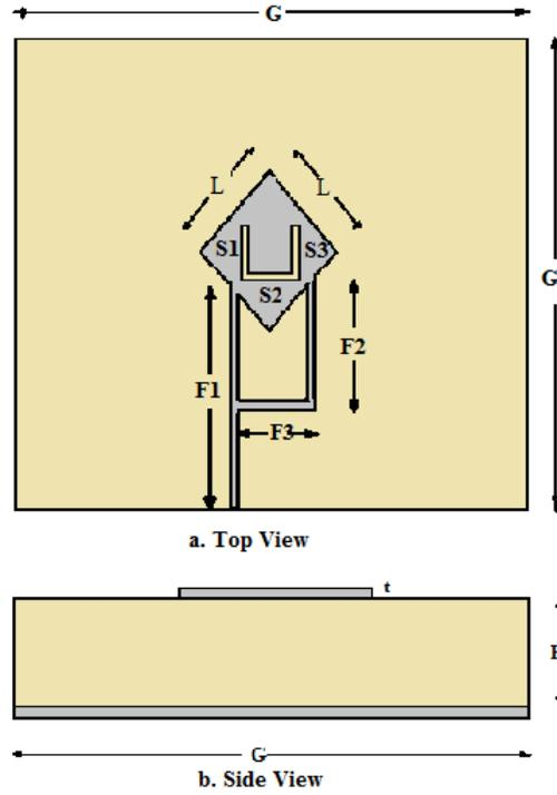
Fig. 4.1. Geometry of the designed antenna.
