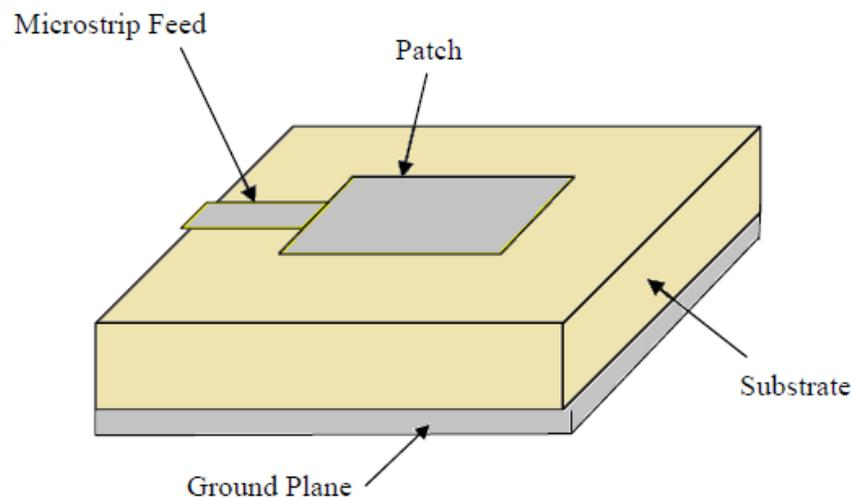
Fig. 2.4. A microstrip line feeding scheme.
