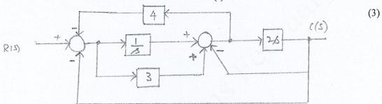
2. Using Mason's rule, find the transfer function  $\frac{C(s)}{R(s)}$  for the system represented below. (4)
