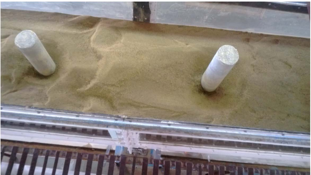
Fig 4.30: Snap shot of the scour hole for both the pier at x/b=9
