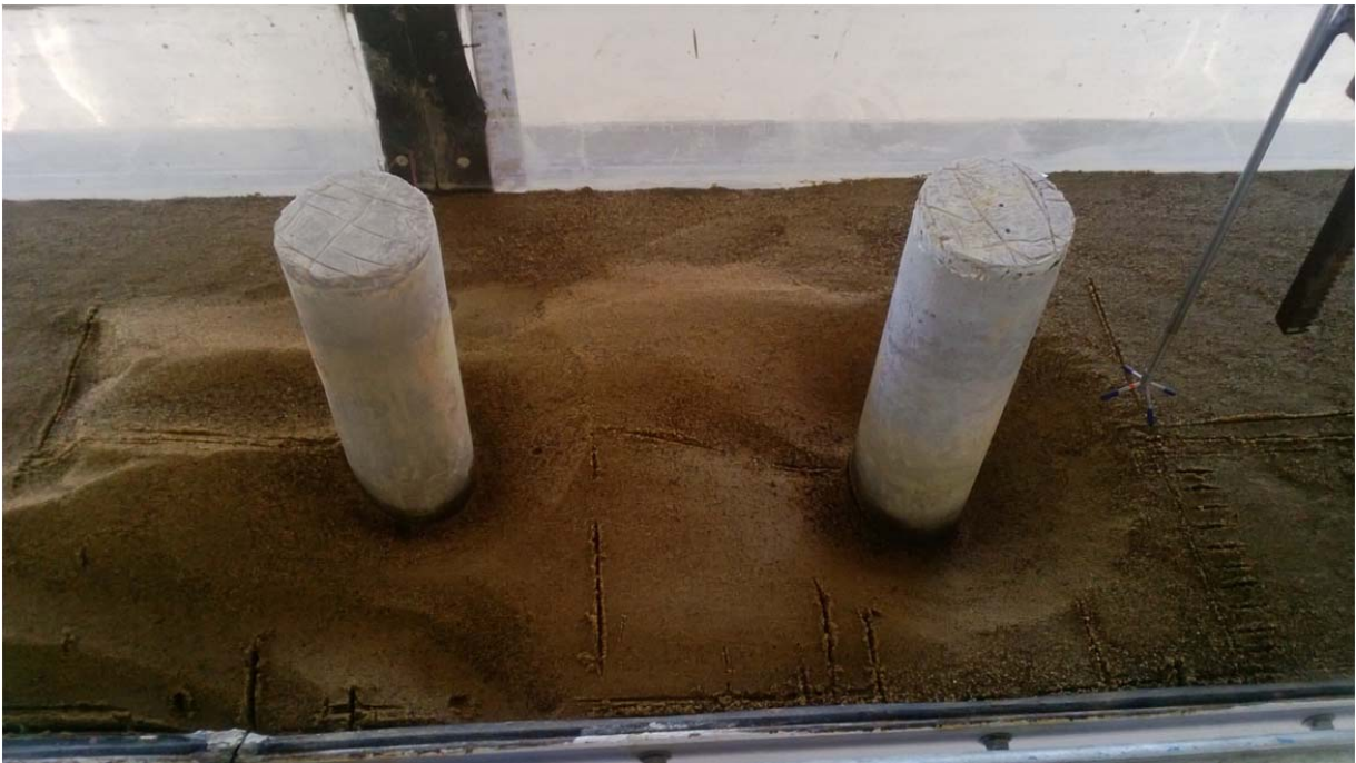
Fig no: 4.27 Snap shot of the scour hole for both the pier at x/b=5
