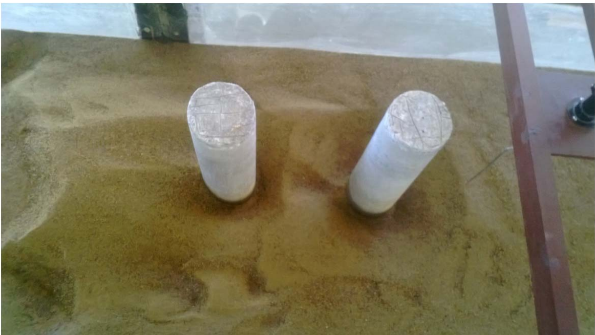
Fig 4.26: Snap shot of scour depth for both piers (upstream and downstream) at a spacing of 3 times the pier diameter
