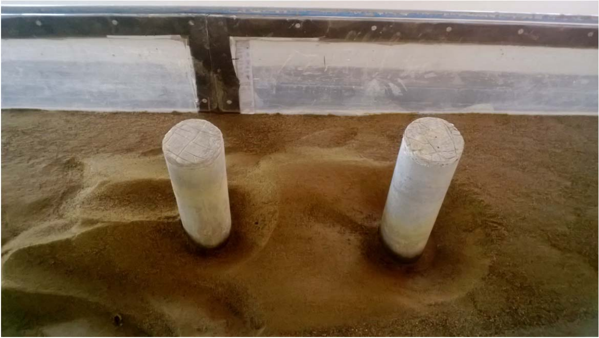
Fig no: 4.27 Snap shot of the scour hole for both the pier at x/b=5
