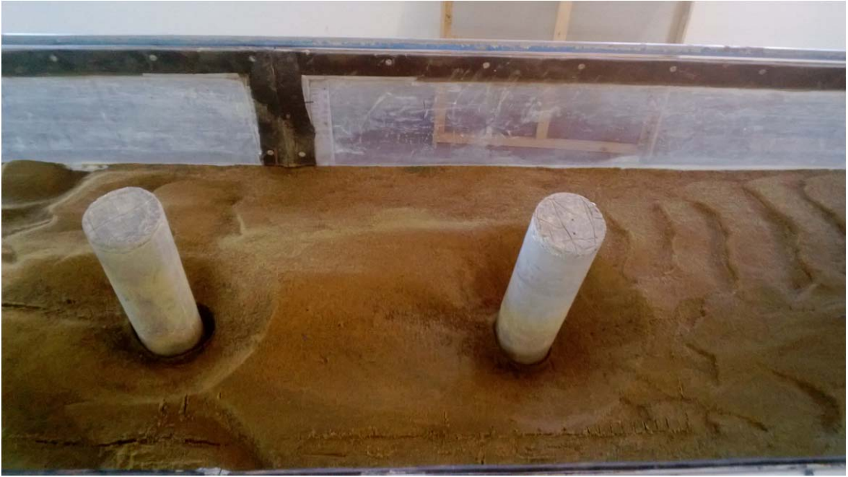
Fig 4.29: Snap shot of the scour hole for both the pier at x/b=12
