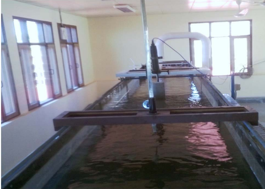
Fig 3.2 pointer gauge used for measuring scour depth
