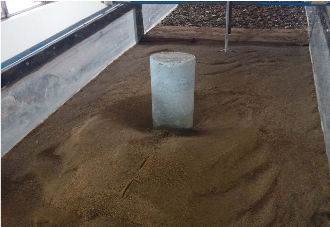
Fig 4.25 Snap of the Scour hole for isolated circular bridge
