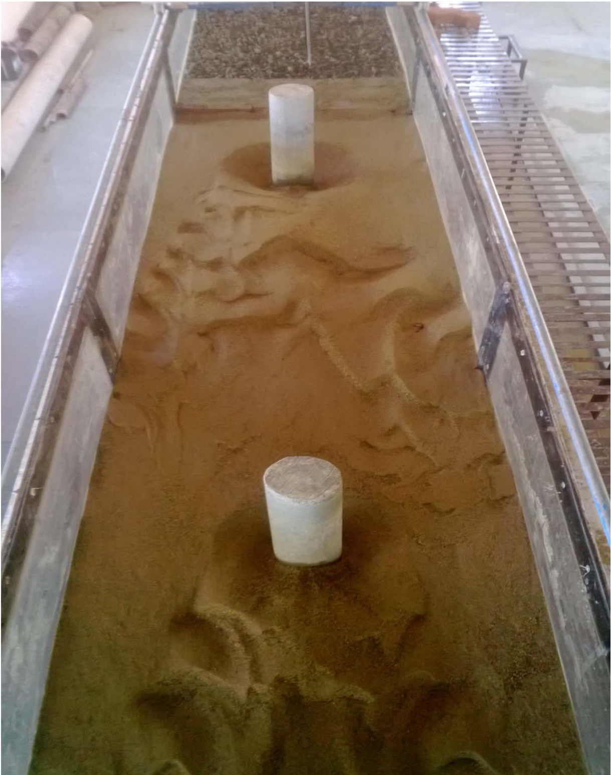
Fig 4.32: Snap shot of the scour hole for both the pier at x/b=14
