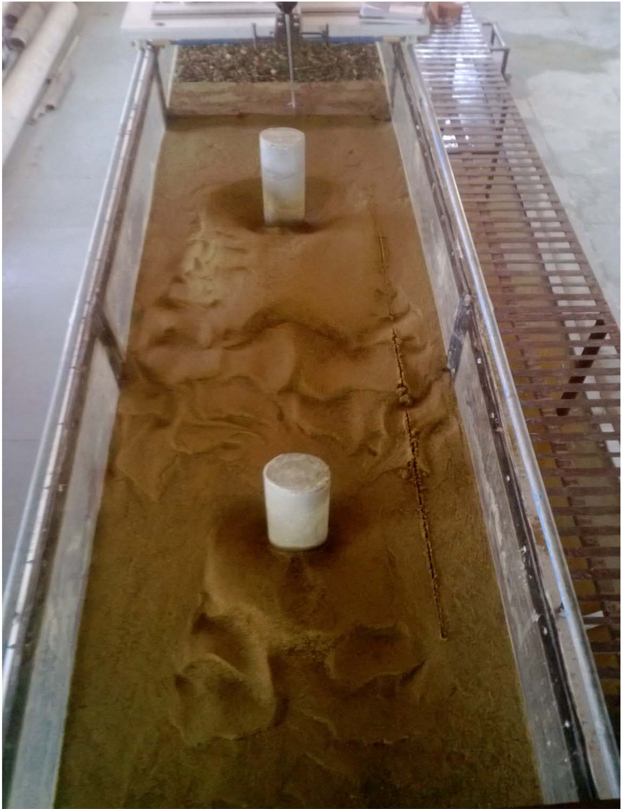
Fig 4.31: Snap shot of the scour hole for both the pier at x/b=12
