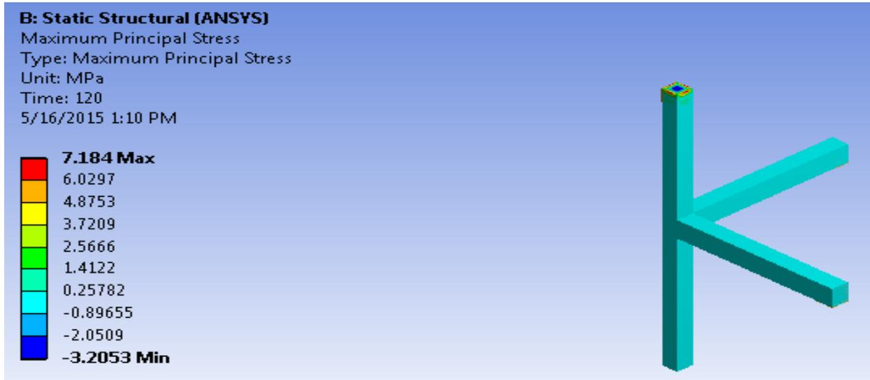
Fig. 5.2.3 Maximum Principal Stress for control specimen with two beams (CS2)
