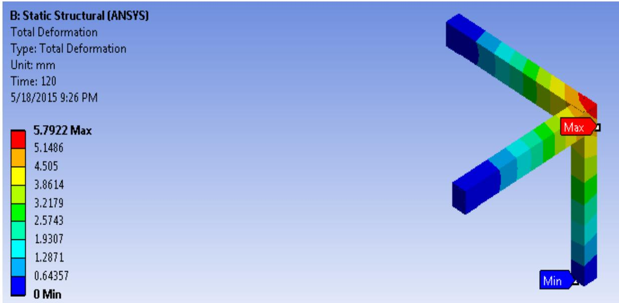
Fig. 5.5.1 Total Deformation of corner joint for Control Specimen (CS5)
