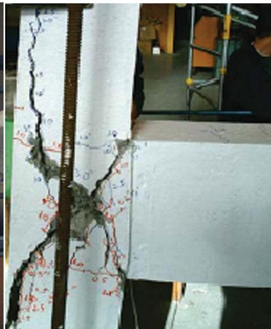
Fig. 2.3.3 Distortion of joint causing diagonal cracks
