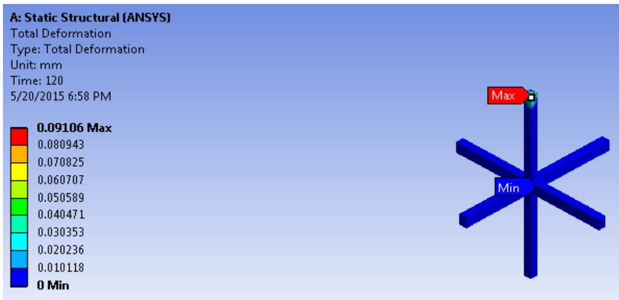
Fig. 5.4.2 Total Deformation for strengthen Specimen with four beams (SS4)
