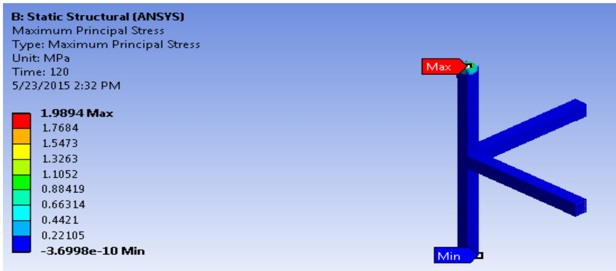
Fig. 5.2.4 Maximum Principal Stress for strengthen specimen with two beams (SS2)
