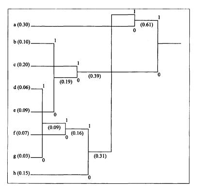
Fig. 3.3 Huffman tree construction for Example 2.
