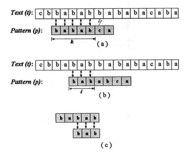
Fig. 4.5 Generation of the Next table. (a) First k characters of p matches with the text, (b) p is shifted by k - i positions right, because (c) first i characters of p is also suffix of the first k matched characters.
