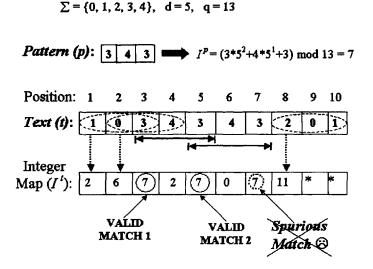
Fig. 4.13 Example of Karp-Rabin string matching algorithm with modulo operation.
