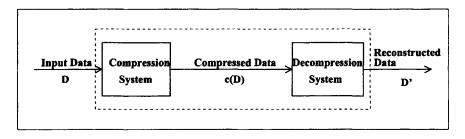
Fig. 3.1 Block diagram of CODEC.
