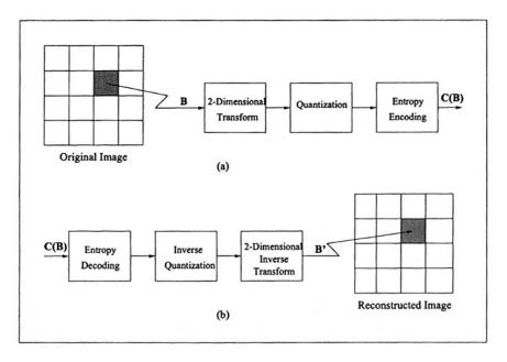
Fig. 3.7 Transform coding-based (a) compression and (b) decompression.
