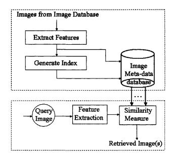
Fig. 9.2 Architecture of a Content Based Image Retrieval System.
