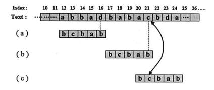
Fig. 4.8 Example of skipping character comparisons in Boyer-Moore algorithm for pattern matching. (a) Current pattern position, (b) pattern completely shifted right because 'd' does not appear in the pattern, (c) pattern is shifted by three positions to align with character 'c'.
