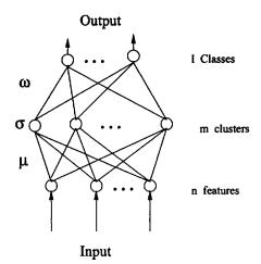
Fig. 2.5 Radial basis function network.
