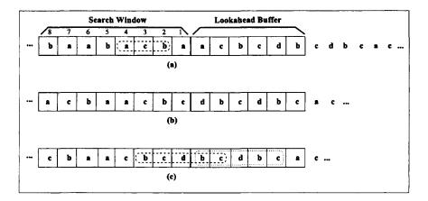
Fig. 3.18 LZ77 coding: An example with sliding window.
