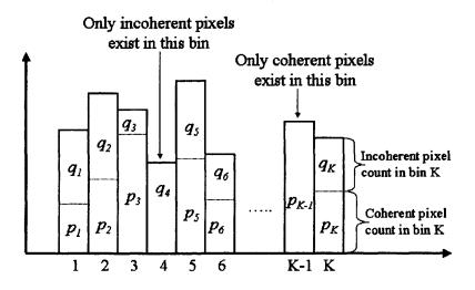
Fig. 9.4 Partitioning the color histogram with coherence and noncoherence pixel counts.
