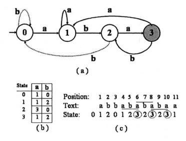
Fig. 4.4 Finite automata: (a) state diagram, (b) state transition table, and (c) pattern matching example.
