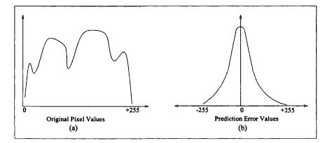
Fig. 3.6 Histogram of (a) a typical image and (b) its prediction error.
