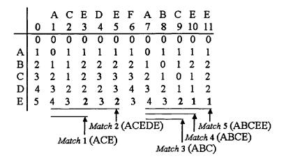
Fig. 4.17 Example of text search with k-mismatches for k = 2.
