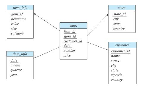
Figure 11.2 Star schema for a data warehouse.
