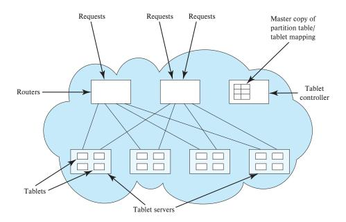
Figure 21.8 Architecture of a cloud data storage system.
