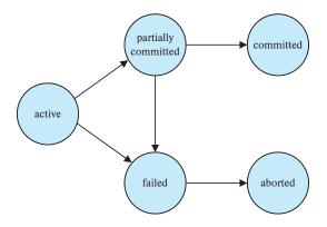
Figure 17.1 State diagram of a transaction.
