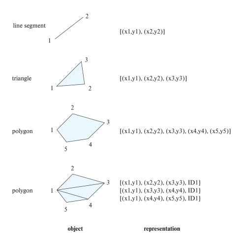
Figure 8.5 Representation of geometric constructs.
