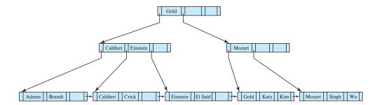
Figure 14.18 Deletion of "Srinivasan" from the B+-tree of Figure 14.14.
