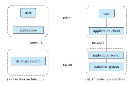
Figure 1.4 Two-tier and three-tier architectures.
