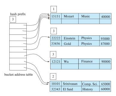
Figure 24.13 Hash structure after six insertions.
