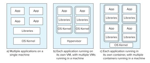
Figure 20.11 Application deployment alternatives.
