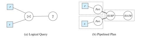
Figure 15.12 Query plan with pipelining.
