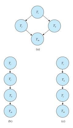
Figure 17.12 Illustration of topological sorting.
