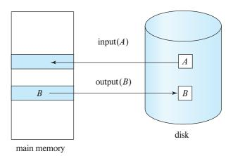
Figure 19.1 Block storage operations.
