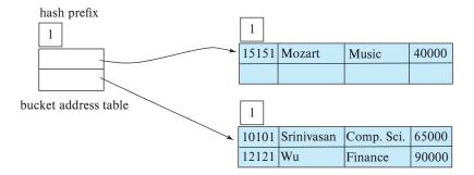
Figure 24.11 Hash structure after three insertions.
