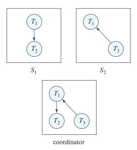
Figure 23.6 False cycles in the global wait-for graph.
