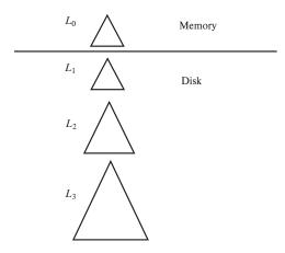
Figure 14.26 Log-structured merge tree with three levels.
