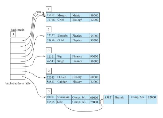
Figure 24.15 Hash structure after 11 insertions.
