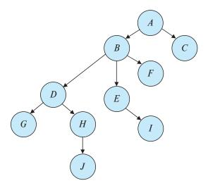
Figure 18.11 Tree-structured database graph.
