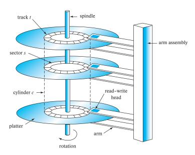
Figure 12.2 Schematic diagram of a magnetic disk.
