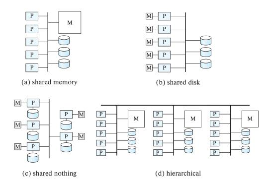
Figure 20.5 Parallel database architectures.
