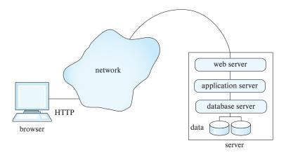
Figure 9.5 Three-layer web application architecture.
