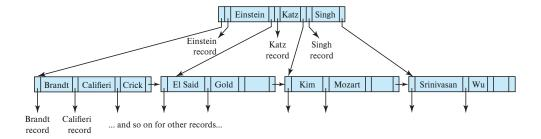
Figure 14.23 B-tree equivalent of B+-tree in Figure 14.9.
