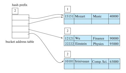
Figure 24.12 Hash structure after four insertions.
