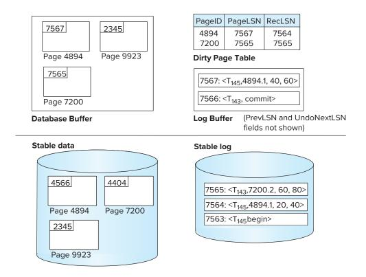
Figure 19.9 Data structures used in ARIES.
