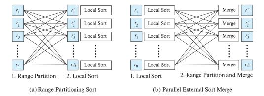
Figure 22.1 Parallel sorting algorithms.
