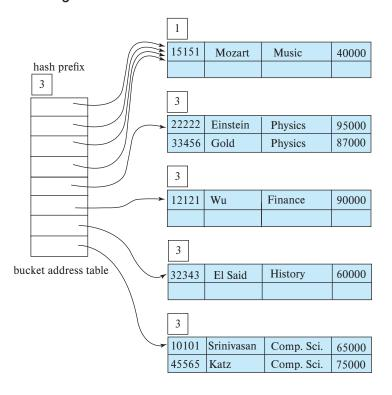
Figure 24.14 Hash structure after seven insertions.
