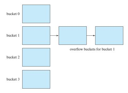
Figure 14.25 Overflow chaining in a disk-based hash structure.
