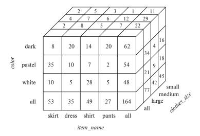
Figure 11.5 Three-dimensional data cube.
