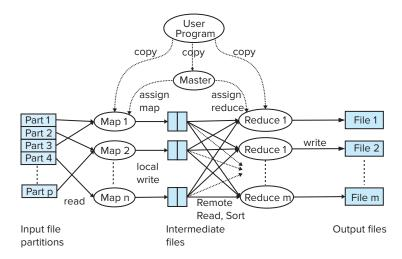
Figure 22.4 Parallel processing of MapReduce job.
