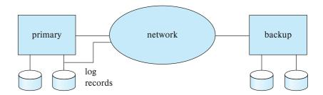
Figure 19.6 Architecture of remote backup system.
