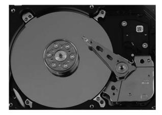
Figure 12.3 Internals of an actual magnetic disk.
