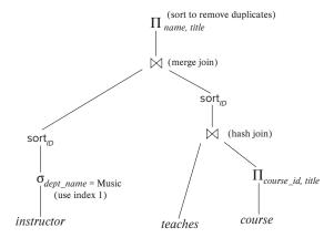
Figure 16.2 An evaluation plan.
