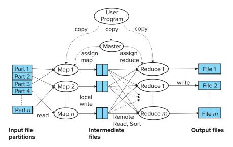
Figure 10.8 Parallel processing of MapReduce job.
