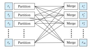
Figure 22.6 The exchange operator used for repartitioning.
