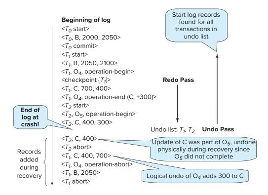
Figure 19.8 Failure recovery actions with logical undo operations.
