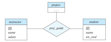
**Figure 6.6** E-R diagram with a ternary relationship *proj-guide*.
