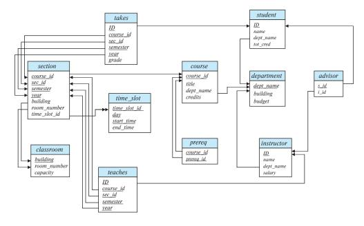
Figure 2.9 Schema diagram for the university database.
