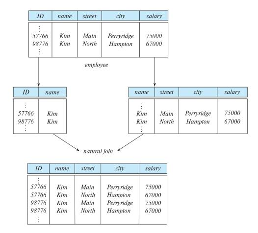
Figure 7.3 Loss of information via a bad decomposition.
