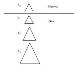
Figure 24.1 Log-structured merge tree with three levels.
