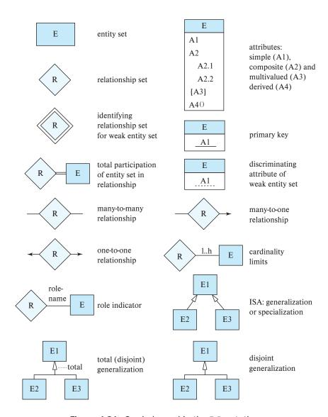
Figure 6.26 Symbols used in the E-R notation.
