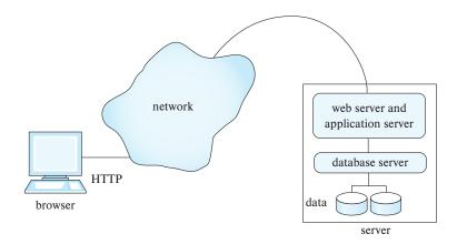
Figure 9.6 Two-layer web application architecture.
