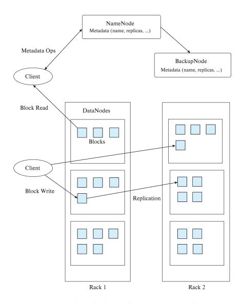
Figure 21.7 Hadoop Distributed File System (HDFS) architecture
