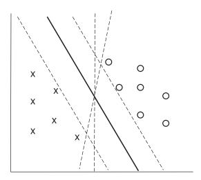
Figure 11.12 Example of a Support Vector Machine classifier.
