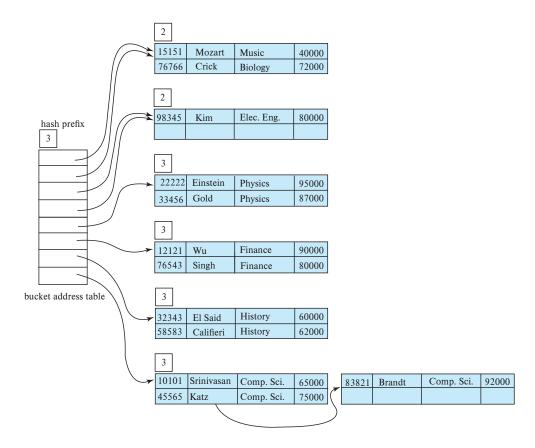
Figure 24.16 Extendable hash structure for the *instructor* file.
