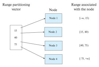
Figure 21.1 Example of range partitioning vector.
