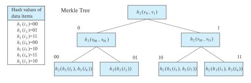
Node identifier shown above node, and has value shown inside node,  $v_i$  denotes stored hash value in node i
