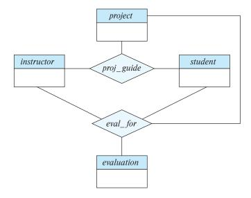
Figure 6.19 E-R diagram with redundant relationships.
