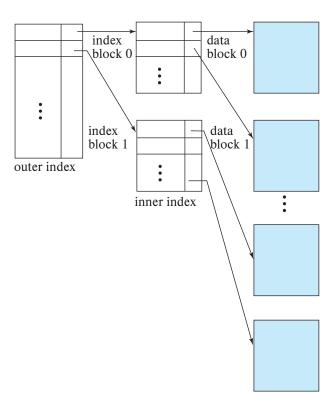
Figure 14.5 Two-level sparse index.
