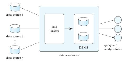
Figure 11.1 Data-warehouse architecture.
