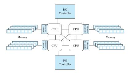
**Figure 20.6** Architecture of a modern shared-memory system.
