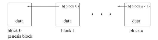
Figure 26.1 Blockchain data structure.
