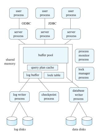
Figure 20.1 Shared memory and process structure.
