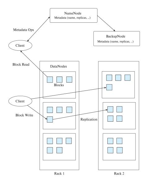
Figure 10.1 Hadoop Distributed File System (HDFS) architecture.
