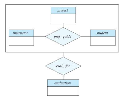
Figure 6.20 E-R diagram with aggregation.
