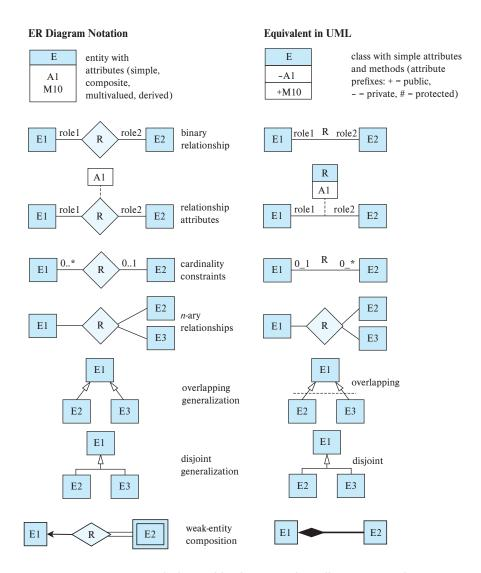
Figure 6.28 Symbols used in the UML class diagram notation.
