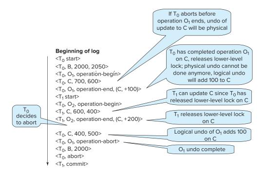
Figure 19.7 Transaction rollback with logical undo operations.
