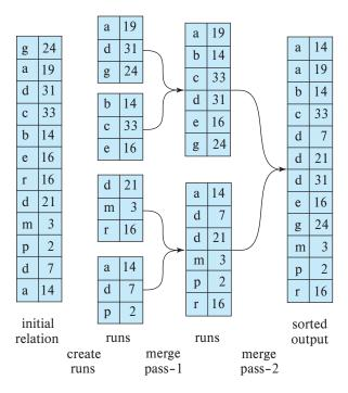
Figure 15.4 External sorting using sort-merge.
