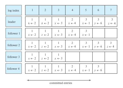
Figure 23.9 Example of Raft logs.
