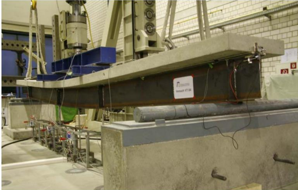
Figure 9 Composite Beam During Test
