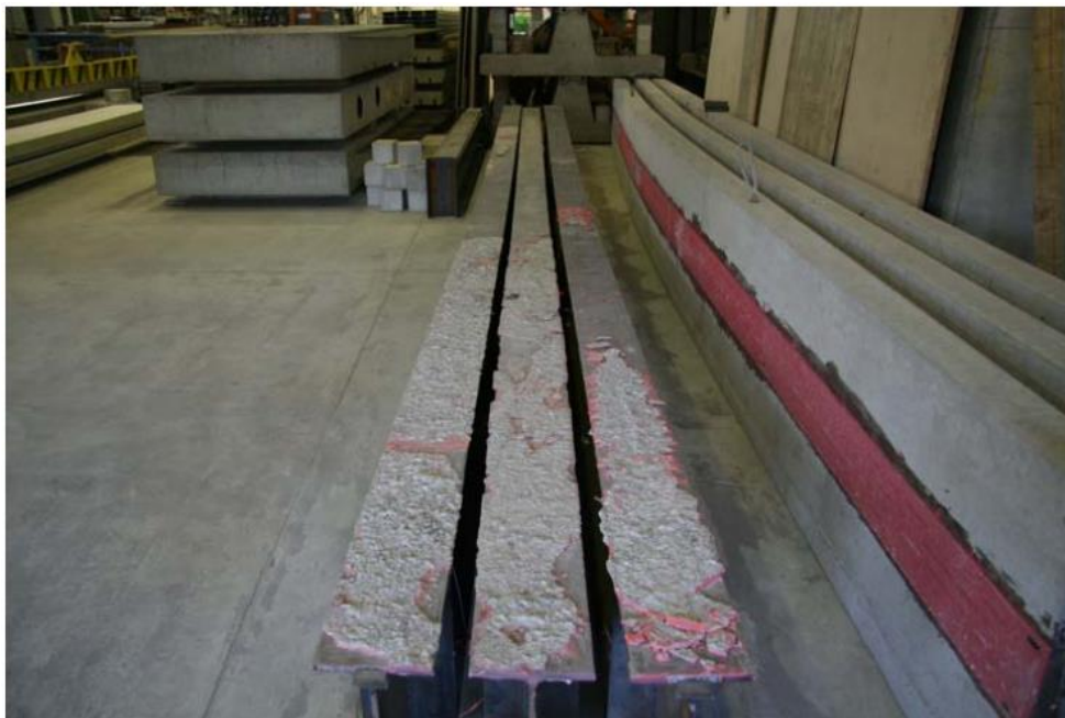
Figure 10 Failure Pattern Of Composite Beams
