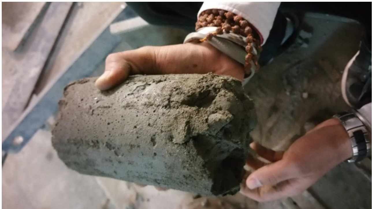
Fig 3.10 Failed Sample at the time of demoulding
