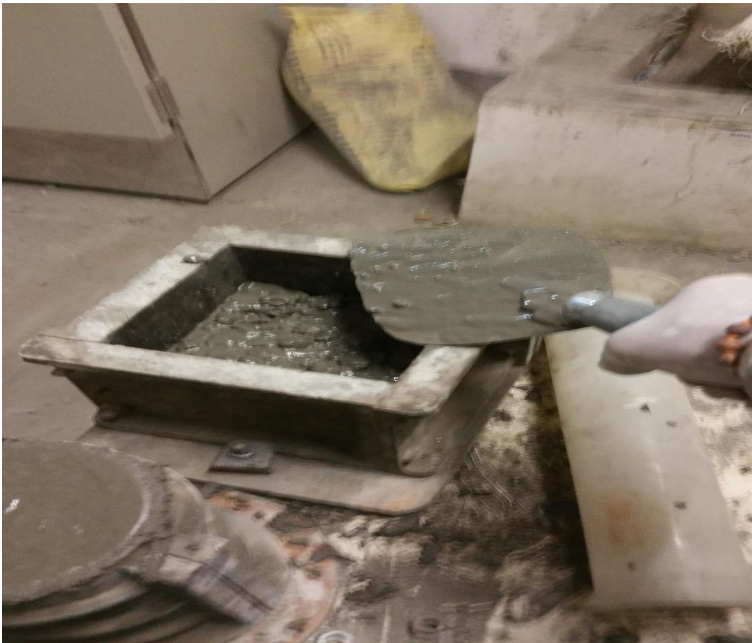
Fig 1.4 – Self Compacting Concrete
