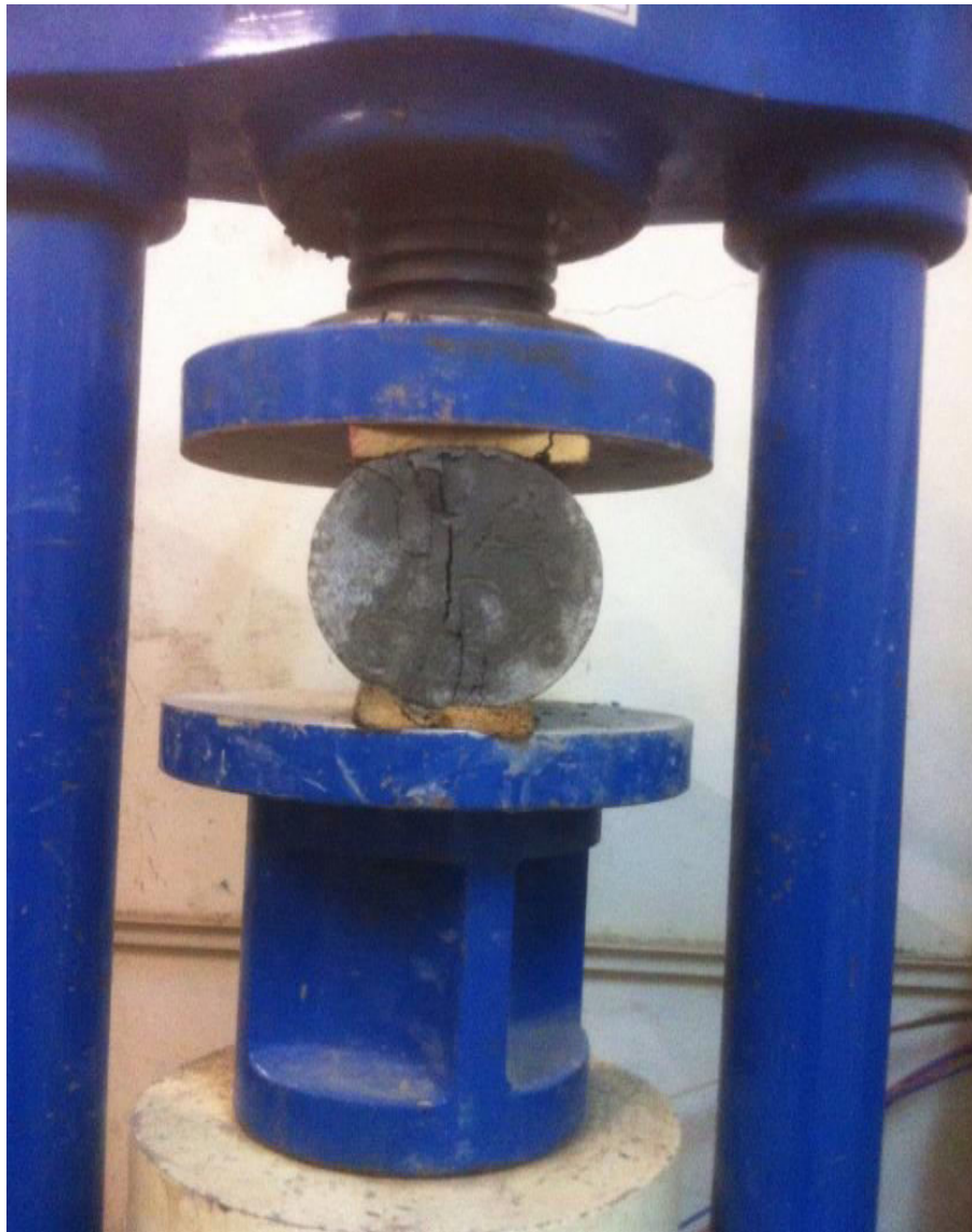
Figure 4.4 Wooden planks being used while calculating the Tensile strength
