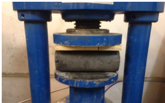
Fig 27- Split tensile testing
