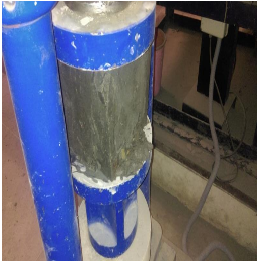
Fig7 – Compressive strength testing
