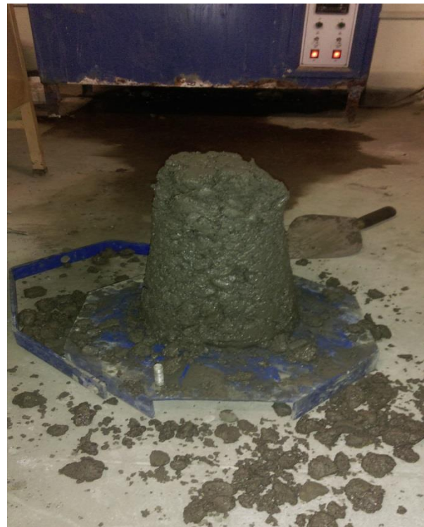
Fig 23 (a)– Slump test for different proportions
