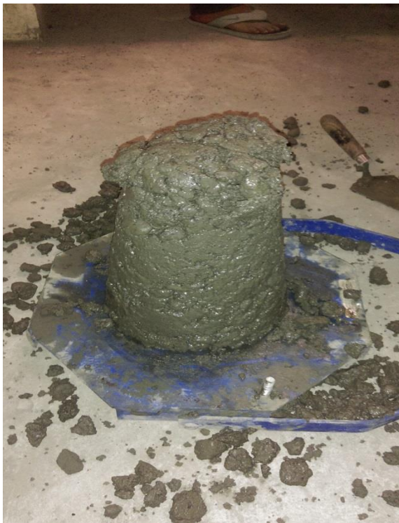
Fig 23 (a)– Slump test for different proportions
