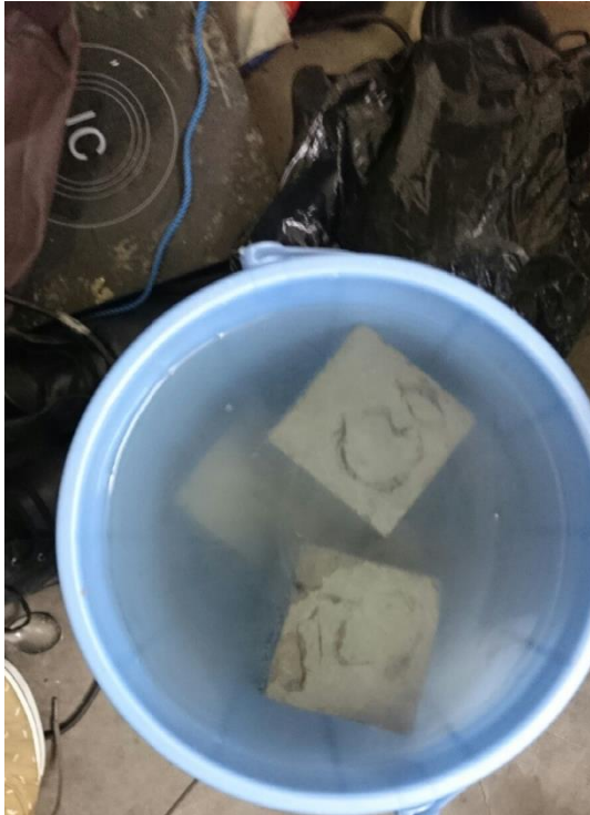
Fig17 – Chloride attack test
