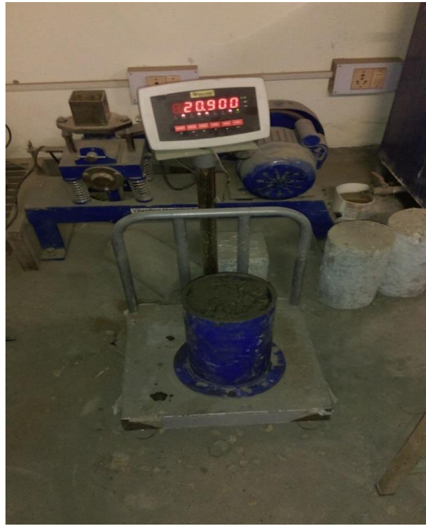
Fig11 – Compaction factor test
