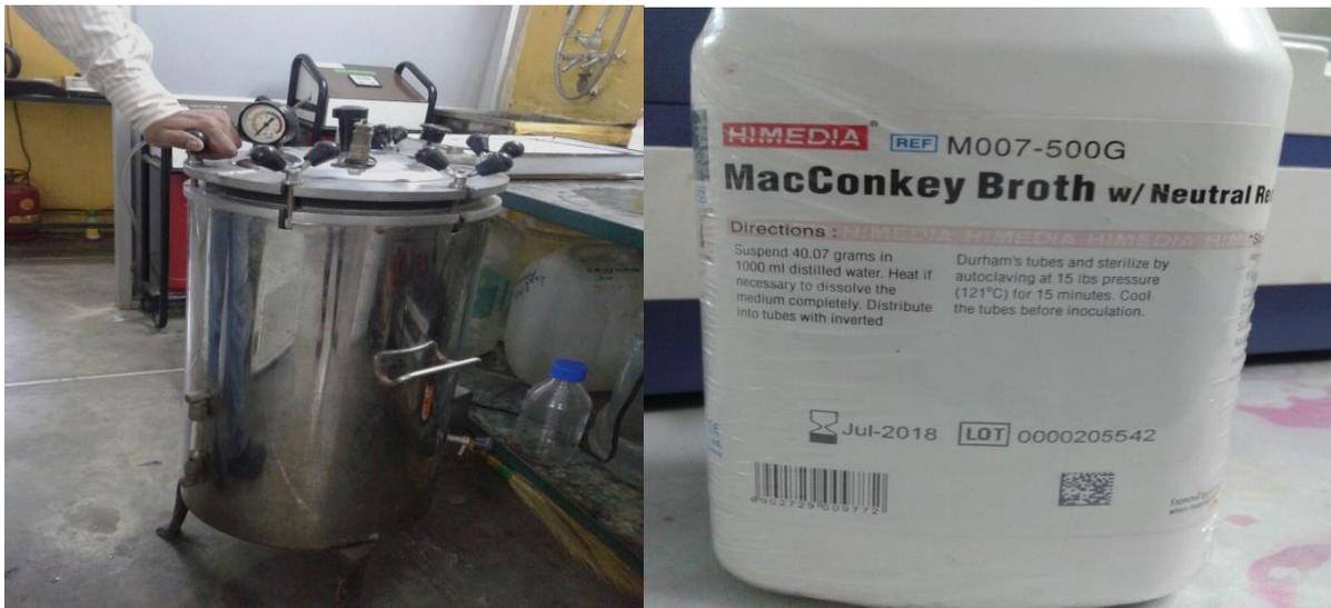
**Figure 3.3.11** Autoclave and media used for bacteriological examination
