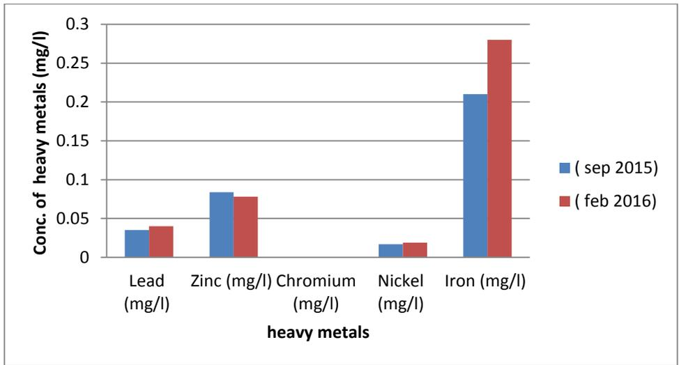
**Figure 4.4** Result of heavy metals for leachate sample
