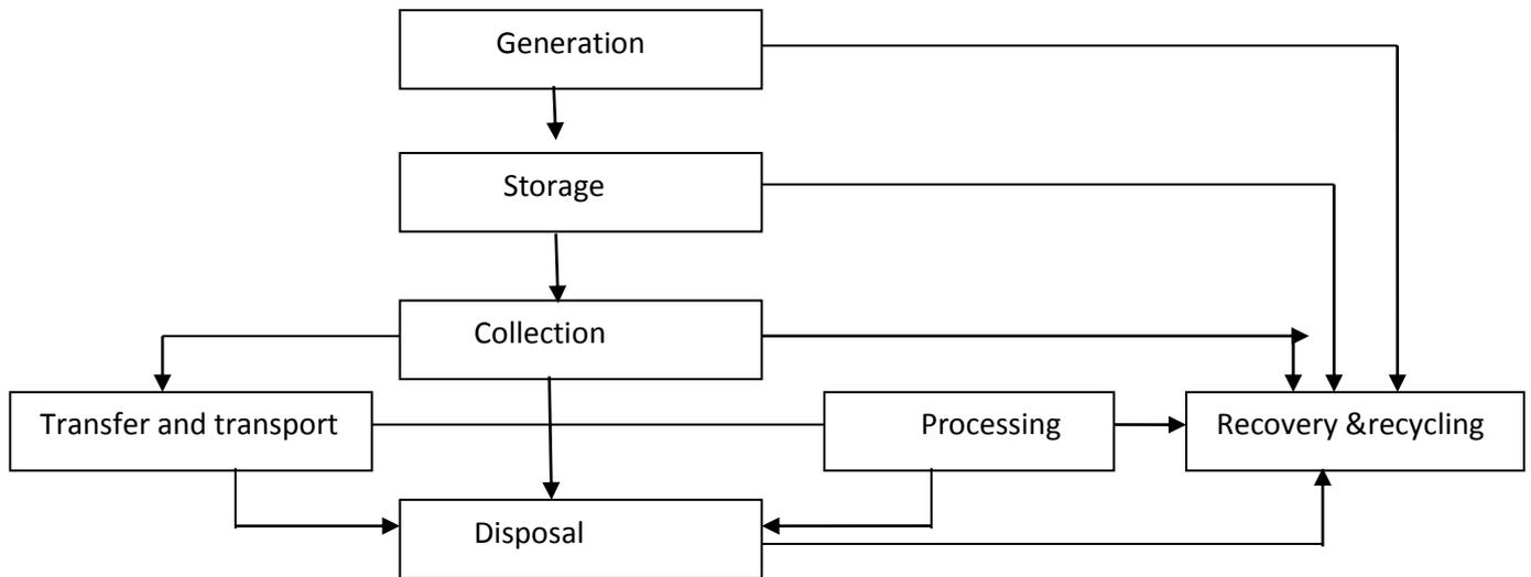
**Figure 1.1** Typical SWM Systems: Functional Elements
