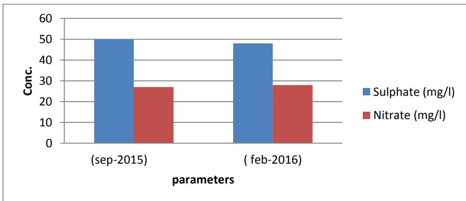
**Figure 4.2** Sulphate and Nitrate result for leachate samples
