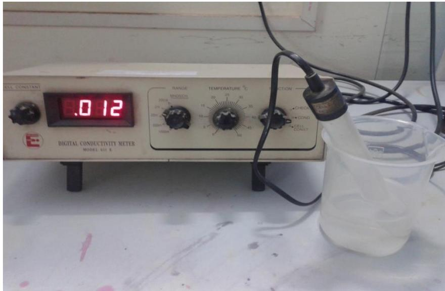
**Figure 3.3.4** Conductivity meter
