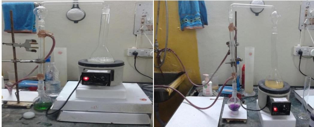
**Figure 3.3.9** Kjeldahl apparatus for total nitrogen
