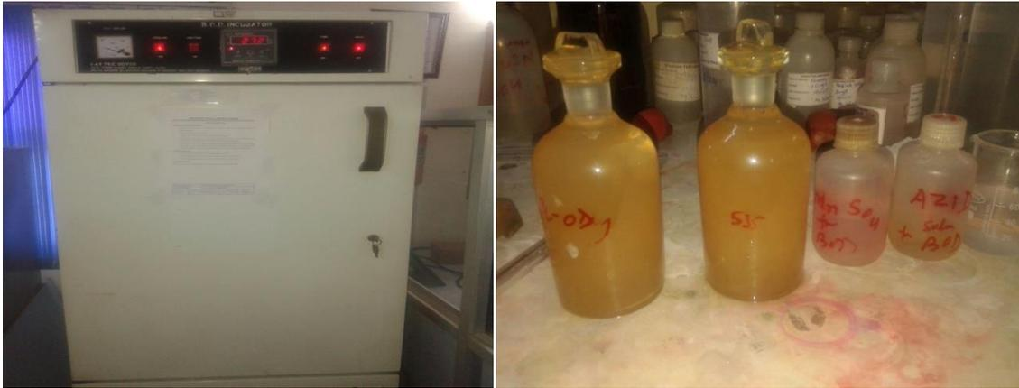
**Figure 3.3.5** BOD incubator and BOD bottles
