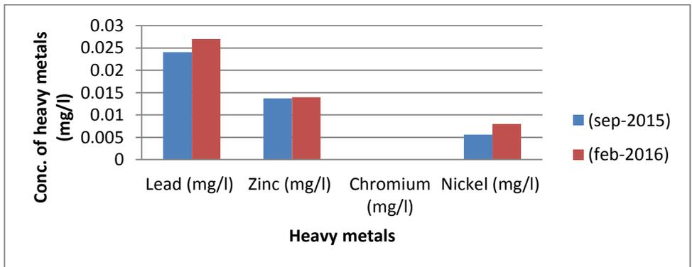
**Figure 4.6** Result of heavy metals for ground water sample
