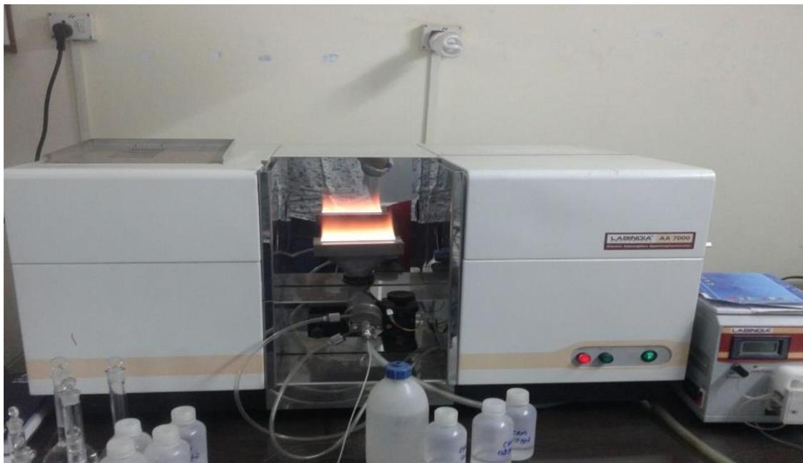
**Figure 3.3.10** Atomic absorption spectrometer
