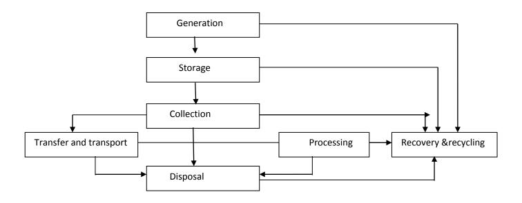
Figure 1.1 Typical SWM Systems: Functional Elements
