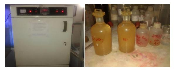
Figure 3.3.5 BOD incubator and BOD bottles
