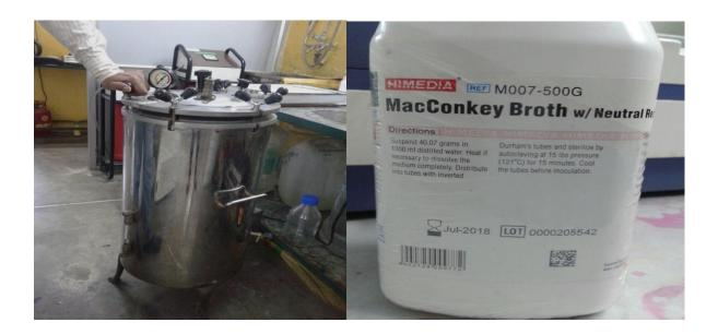
Figure 3.3.11 Autoclave and media used for bacteriological examination
