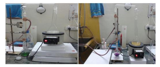
Figure 3.3.9 Kjeldahl apparatus for total nitrogen
