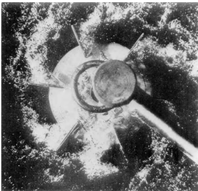
FIGURE 8.20 Gas cavities that are formed behind the blades of a 7.6-cm Rushton turbine in water. The impeller was rotated counterclockwise; the camera was located below the impeller and ring sparger.
