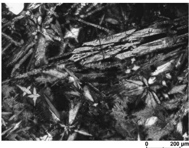
Fig. 8.1 Hedenbergite crystals in a MSWI bottom ash aggregate (Müller and Rübner, 2006)
