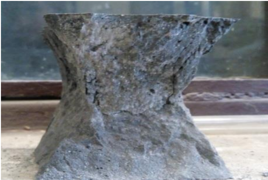
Figure 37 Brittle failure of cube 1
