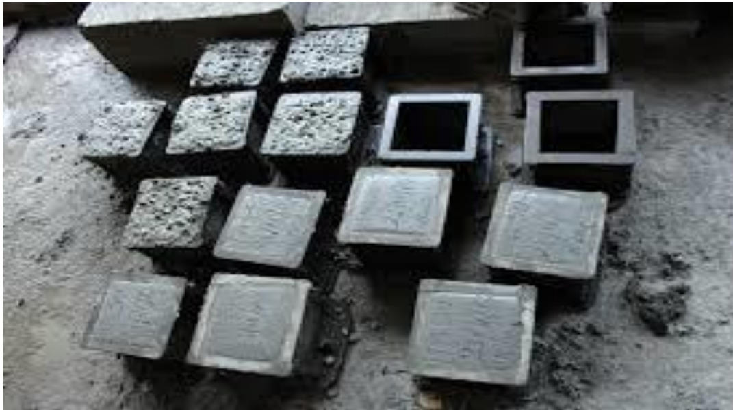
Figure 30 Casting of cubes
