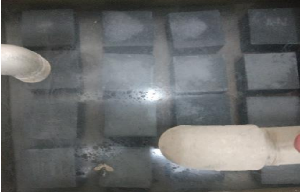
Figure 31 Curing of cubes 1
