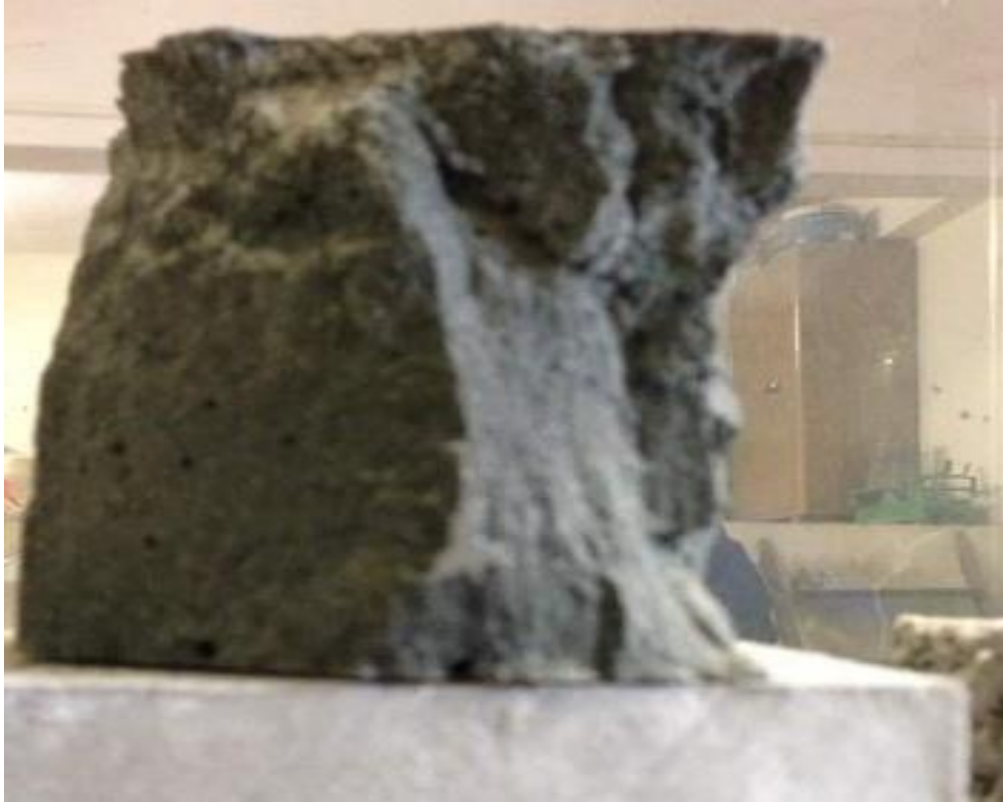
Figure 38 Brittle failure in cube2
