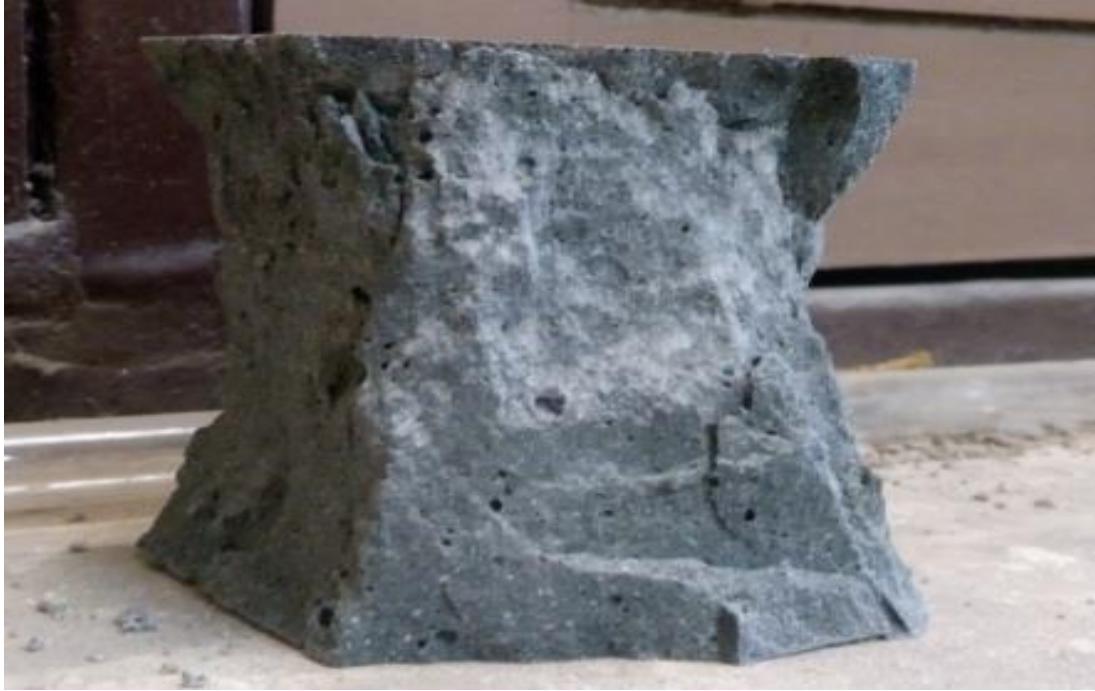
Figure 36 Pores in cube due to less compaction
