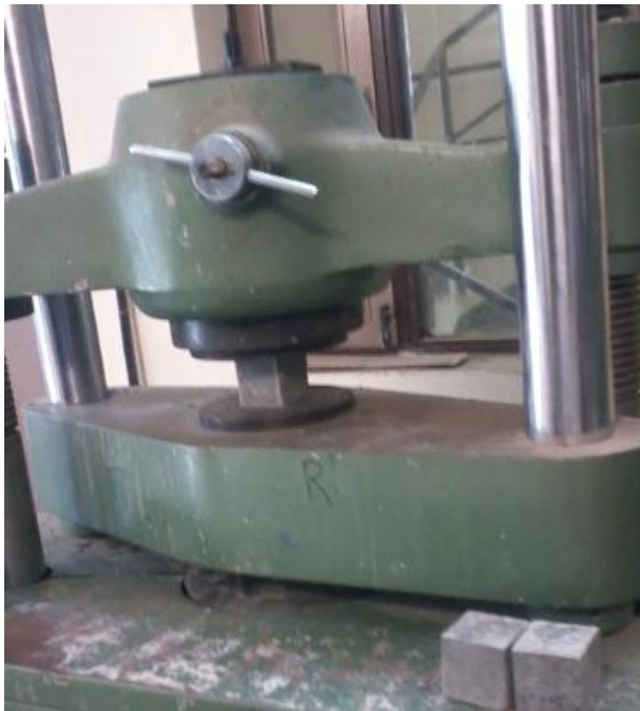
Figure 33 Testing of cubes in UTM
