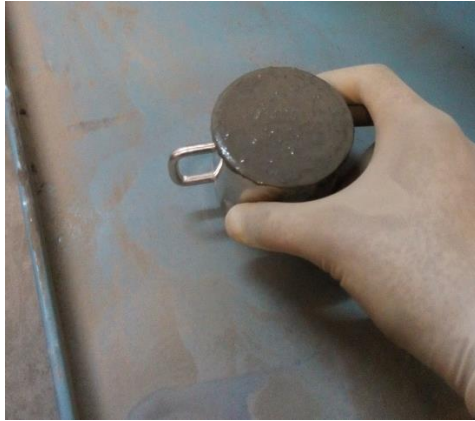
Fig. 14. Compaction on vibrating table
