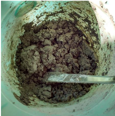
Fig. 10. Wet mix at 0.26 W/S ratio
