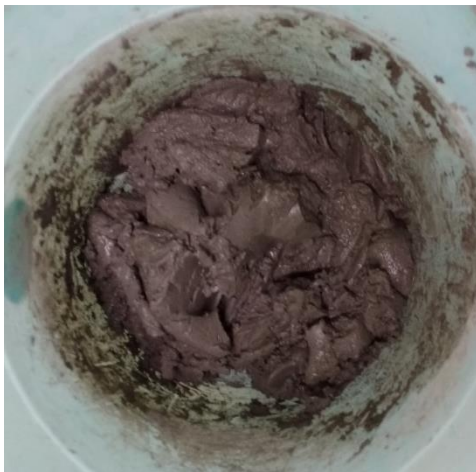
Fig. 12. Wet mix at 0.28 W/S ratio
