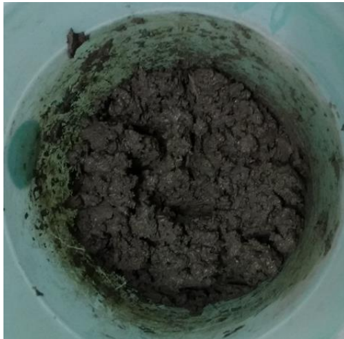
Fig. 11. Wet mix at 0.27 W/S ratio
