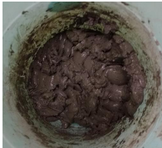
Fig. 13. Wet mix at 0.29 W/S ratio
