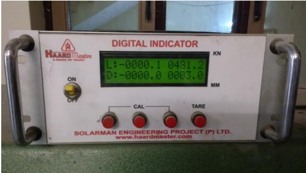
Fig. 22. Load readings on UTM
