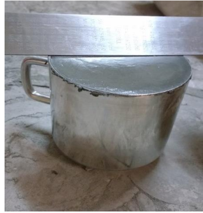
Fig. 15. Levelling of the surface
