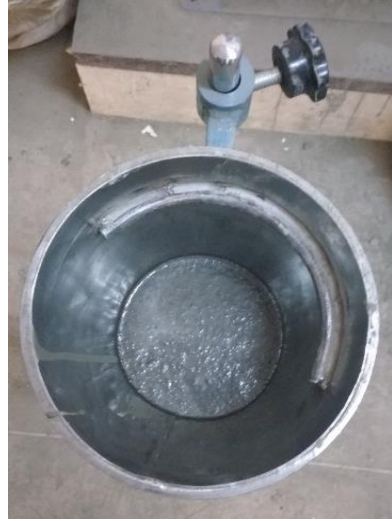
Fig. 17. Material filled in Marsh Cone
