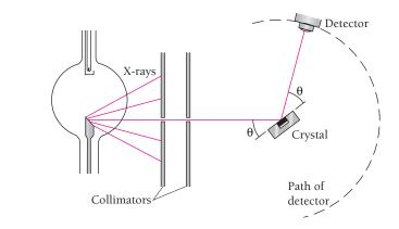
Figure 2.21 X-ray spectrometer.
