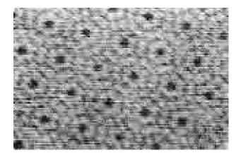
Silicon atoms on the surface of a silicon crystal form a regular, repeated pattern in this image produced by an STM.
