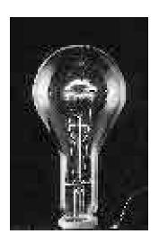
The color and brightness of an object heated until it glows, such as the filament of this light bulb, depends upon its temperature, which here is about 3000 K. An object that glows white is hotter than it is when it glows red, and it gives off more light as well.
