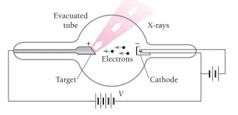
Figure 2.15 An x-ray tube. The higher the accelerating voltage *V*, the faster the electrons and the shorter the wavelengths of the x-rays.
