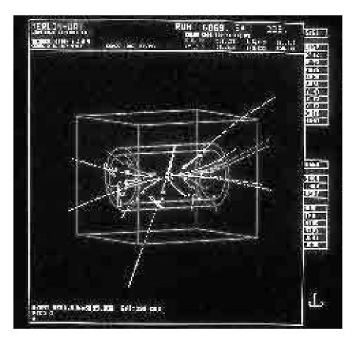
Computer reconstruction of the results of a proton-antiproton collision in which a *W* boson was created. The UAI detector is outlined in the display. The *W* boson, one of the "carriers" of the weak force, was first identified at CERN in 1983.
