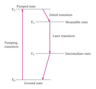
Figure 4.28 A four-level laser.
