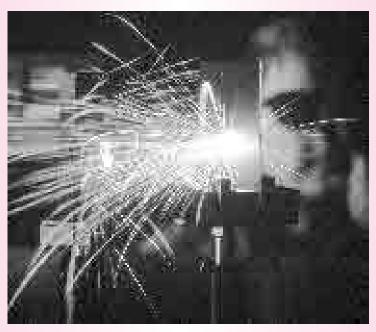
Solid-state infrared laser cutting 1.6-mm steel sheet. This laser uses an yttrium-aluminumgarnet crystal doped with neodymium. The neodymium is pumped with radiation from small semiconductor lasers, a highly efficient method.
