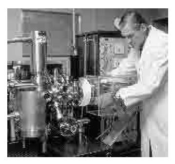
In the operation of this x-ray spectrometer, a stream of fast electrons is directed at a sample of unknown composition. Some of the electrons knock out inner electrons in the target atoms, and when outer electrons replace them, x-ray are emitted whose wavelengths are characteristic of the elements present. The identity and relative amounts of the elements in the sample can be found in this way.
