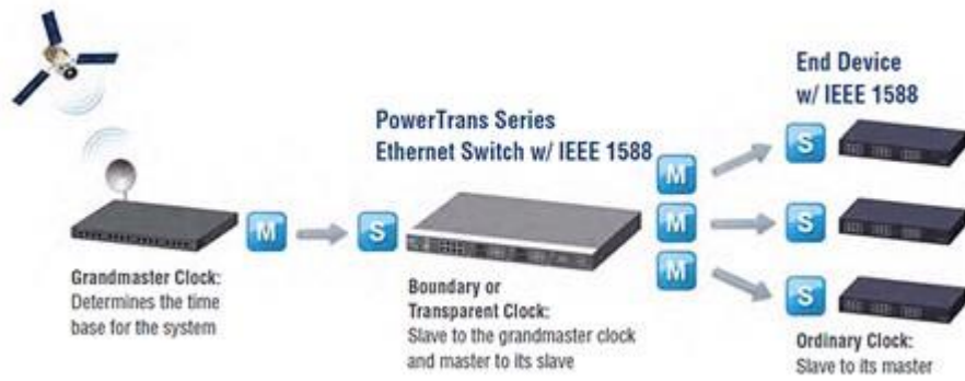
Figure 21 Precision Time Protocol (PTP) –UTC Sync
