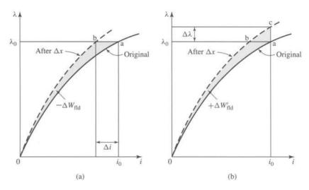
**Figure 3.11** Effect of  $\Delta x$  on the energy and coenergy of a singly-excited device: (a) change of energy with  $\lambda$  held constant; (b) change of coenergy with i held constant.
