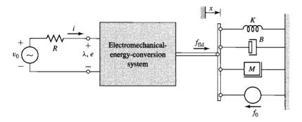
**Figure 3.23** Model of a singly-excited electromechanical system.
