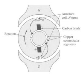
**Figure 4.17** Elementary dc machine with commutator
