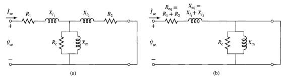
**Figure 2.15** Equivalent circuit with short-circuited secondary. (a) Complete equivalent circuit. (b) Cantilever equivalent circuit with the exciting branch at the transformer secondary.
