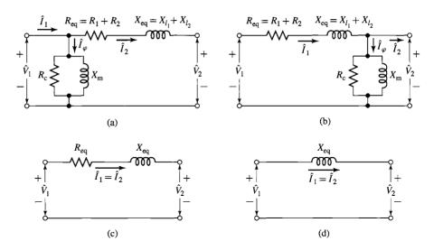
Figure 2.12 Approximate transformer equivalent circuits.
