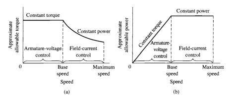
**Figure 11.6** (a) Torque and (b) power limitations of combined armature-voltage and field-current methods of speed control.
