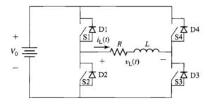
**Figure 10.45** Single-phase H-bridge inverter configuration.
