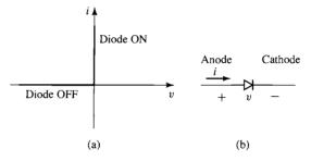
**Figure 10.2** (a) *v-i* characteristic of an ideal diode. (b) Diode symbol.
