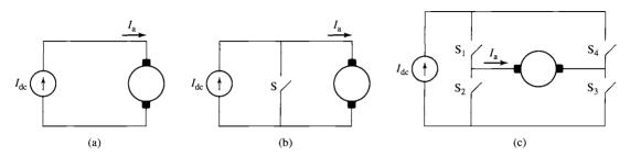
**Figure 11.9** Three typical configurations for armature-current control. (a) Variable dc-link current (produced by a phase-controlled rectifier) applied directly to the dc-motor armature terminals. (b) Constant dc-link current with single-polarity pulse-width modulation. (c) Constant dc-link current with a full H-bridge.
