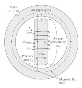
Figure 1.5 Simple synchronous machine.
