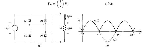
Figure 10.15 (a) Full-wave bridge rectifier. (b) Resistor voltage.
