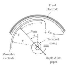
**Figure 3.35** Schematic electrostatic voltmeter (Problem 3.21).
