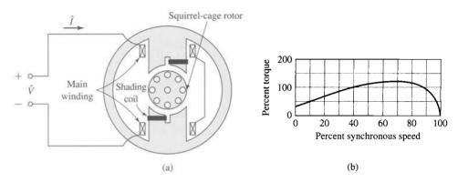
Figure 9.8 Shaded-pole induction motor and typical torque-speed characteristic.
