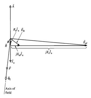
**Figure 5.8** Phasor diagram for short-circuit conditions.
