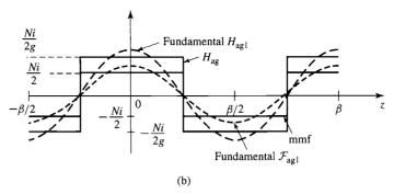
**Figure 4.36** The mmf and H field of a concentrated full-pitch linear winding.
