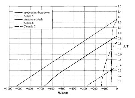
Figure 1.19 Magnetization curves for common permanent-magnet materials.
