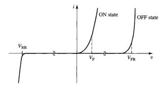
Figure 10.4 *v-i* characteristic of an SCR.
