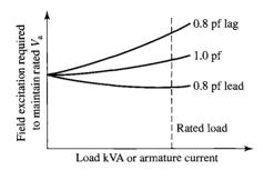
**Figure 5.15** Characteristic form of synchronous-generator compounding curves.
