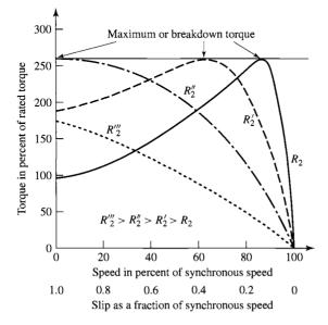
**Figure 6.16** Induction-motor torque-slip curves showing effect of changing rotor-circuit resistance.
