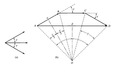
Figure B.3 (a) Coil voltage phasors and (b) phasor sum.
