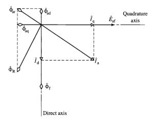
**Figure 5.22** Phasor diagram of a salient-pole synchronous generator.
