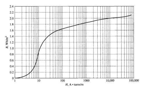
**Figure 1.10** Dc magnetization curve for M-5 grain-oriented electrical steel 0.012 in thick. (*Armco Inc.*)
