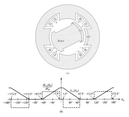
**Figure 8.12** A 4/2 VRM with 15° rotor overhang: (a) cross-sectional view and (b) plots of  $L_{11}(\theta_{\rm m})$  and  $dL_{11}(\theta_{\rm m})/d\theta_{\rm m}$  versus  $\theta_{\rm m}$ .
