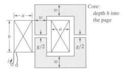
**Figure 1.31** Iron-core inductor for Problem 1.20.
