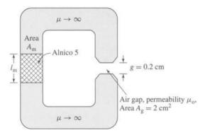
Figure 1.18 Magnetic circuit for Example 1.10.
