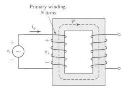
**Figure 2.4** Transformer with open secondary.
