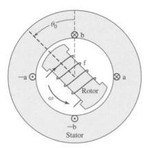
**Figure 4.46** Schematic two-phase, salient-pole synchronous machine for Problem 4.24.
