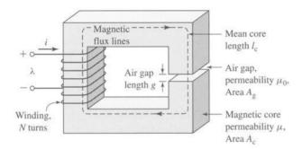
Figure 1.2 Magnetic circuit with air gap.
