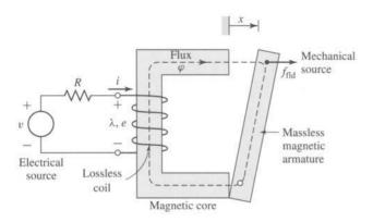
Figure 3.4 Schematic of an electromagnetic relay.
