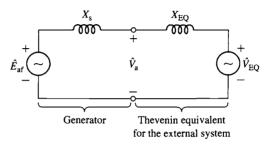
**Figure 5.12** Equivalent-circuit representation of a synchronous machine connected to an external system.
