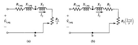
**Figure 6.13** Induction-motor equivalent circuits simplified by Thevenin's theorem.
