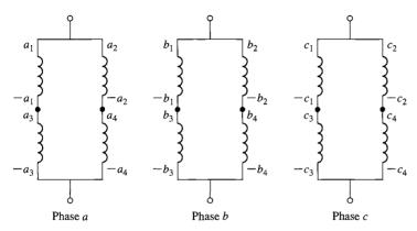
Figure B.10 Coil phase connections of Fig. B.2 for Example B.2.
