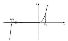
**Figure 10.1** *v-i* characteristic of a diode.
