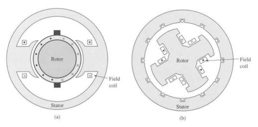
**Figure 4.26** Structure of typical salient-pole machines: (a) dc machine and (b) salient-pole synchronous machine.
