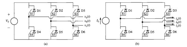
Figure 10.48 Three-phase inverter configurations. (a) Voltage-source. (b) Current-source.
