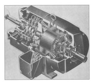
**Figure 6.1** Cutaway view of a three-phase induction motor with a wound rotor and slip rings connected to the three-phase rotor winding. (*General Electric Company*.)
