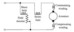
**Figure 7.24** Schematic connection diagram of a dc machine.
