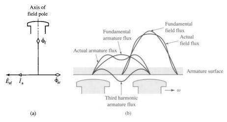
Figure 5.21 Quadrature-axis air-gap fluxes in a salient-pole synchronous machine.
