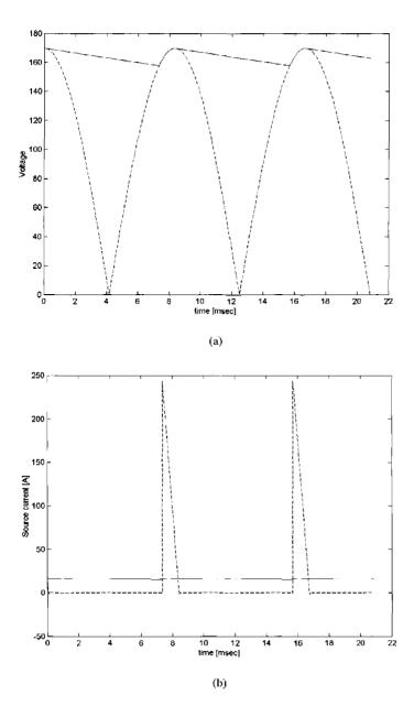
**Figure 10.17** Example 10.5. (a) Resistor voltage and rectified source voltage (dashed). (b) Resistor current and total bridge current (dashed).
