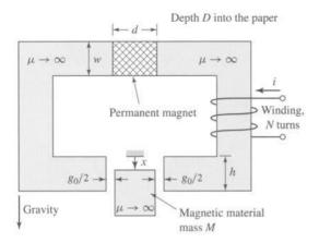
**Figure 3.38** Magnetic support system for Problem 3.27.
