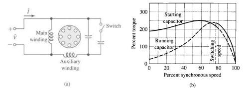
Figure 9.7 Capacitor-start, capacitor-run motor and typical torque-speed characteristic.
