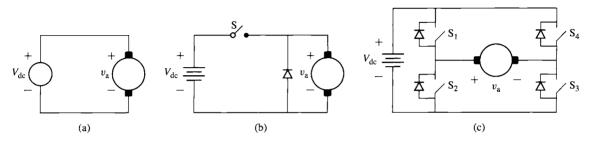
**Figure 11.4** Three typical configurations for armature-voltage control. (a) Variable dc-link voltage (produced by a phase-controlled rectifier) applied directly to the dc-motor armature terminals. (b) Constant dc-link voltage with single-polarity pulse-width modulation. (c) Constant dc-link voltage with a full H-bridge.
