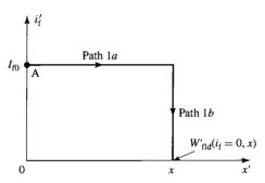
**Figure 3.18** Integration path for calculating  $W_{\text{fld}}(i_{\text{f}} = 0, x)$  in the permanent magnet system of Fig. 3.17.
