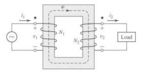
**Figure 2.6** Ideal transformer and load.
