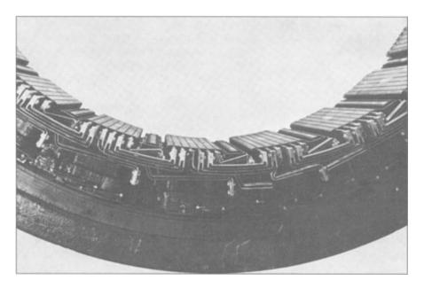
**Figure 7.23** Section of a dc motor stator showing shunt and series coils, interpoles and pole-face compensating winding. (*Westinghouse Electric Company.*)
