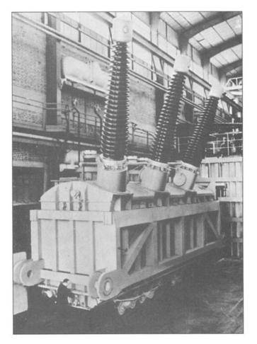
**Figure 2.3** A 660-MVA three-phase 50-Hz transformer used to step up generator voltage of 20 kV to transmission voltage of 405 kV. (*CEM Le Havre, French Member of the Brown Boveri Corporation.*)
