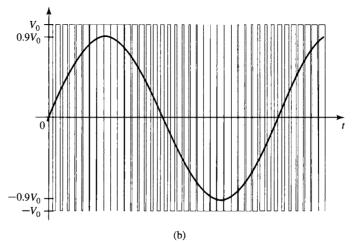
**Figure 10.47** (a) Method for producing a variable duty cycle from a reference waveform  $W_{\rm ref}(t)$ . (b) Load voltage and average load voltage for  $W_{\rm ref}(t) = 0.9 \sin \omega t$ .
