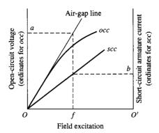
**Figure 5.7** Open- and short-circuit characteristics of a synchronous machine.
