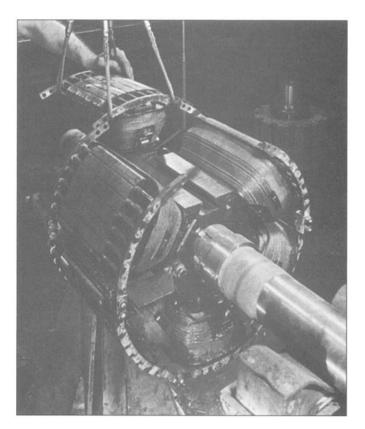
**Figure 5.31** Rotor of a six-pole 1200 r/min synchronous motor showing field coils, pole-face damper winding, and construction. (*General Electric Company*.)
