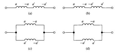
**Figure 11.17** Four possible arrangements of phase-a stator coils in a pole-changing induction motor: (a) series-connected, four-pole; (b) series-connected, two-pole; (c) parallel-connected, four-pole; (d) parallel-connected, two-pole.
