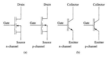
**Figure 10.11** (a) Symbols for n- and p-channel MOSFETs. (b) Symbols for n- and p-channel IGBTs.
