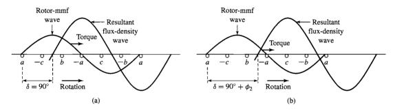
**Figure 6.5** Developed rotor winding of an induction motor with its flux-density and mmf waves in their relative positions for (a) zero and (b) nonzero rotor leakage reactance.
