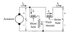
**Figure 7.13** Short-shunt compound-generator connections.
