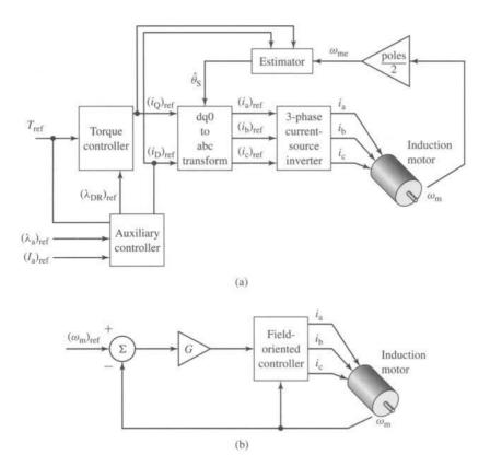
**Figure 11.21** (a) Block diagram of a field-oriented torque-control system for an induction motor. (b) Block diagram of an induction-motor speed-control loop built around a field-oriented torque control system.
