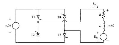
**Figure 10.35** Full-wave, phase-controlled SCR bridge with an inductive load including a dc voltage source.
