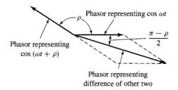
**Figure B.5** Phasor addition for fractional-pitch coil.
