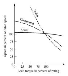
**Figure 7.6** Speed-torque characteristics of dc motors.
