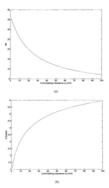
**Figure 10.30** (a) Dc current  $I_{\rm dc}$  and (b) commutation time  $t_{\rm c}$  for Example 10.6.
