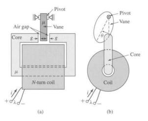
**Figure 3.26** Actuator with rotating vane for Problem 3.7. (a) Side view. (b) End view.
