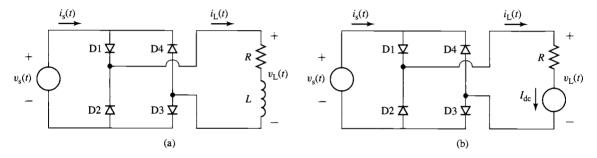
Figure 10.23 (a) Full-wave rectifier with an inductive load. (b) Full-wave rectifier with the inductor replaced by a dc current source.
