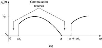
**Figure 10.28** (a) Currents through diodes D1 and D2 showing the finite commutation interval. (b) Load voltage showing the commutation notches due to the finite commutation time.
