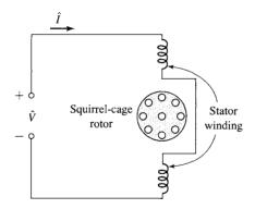
**Figure 9.1** Schematic view of a single-phase induction motor.
