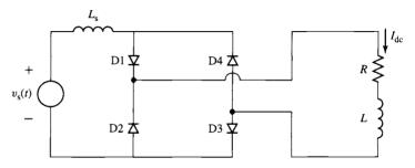
**Figure 10.29** Full-wave bridge rectifier with source inductance for Example 10.6.
