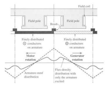
**Figure 7.9** Armature-mmf and flux-density distribution with brushes on neutral and only the armature excited.
