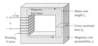
Figure 1.1 Simple magnetic circuit.
