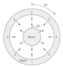
**Figure 8.7** Schematic view of a four-phase 8/6 VRM. Pole locations are indicated by arrows.
