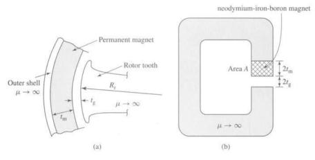
**Figure 7.18** (a) Dimension definitions for the motor of Fig. 7.17, (b) approximate magnetic equivalent circuit.
