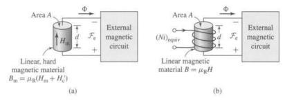
**Figure 3.21** (a) Generic magnetic circuit containing a section of linear, permanent-magnet material. (b) Generic magnetic circuit in which the permanent-magnet material has been replaced by a section of linear magnetic material and a fictitious winding.
