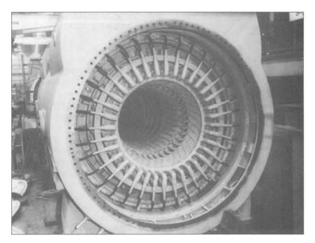
**Figure 4.42** End view of the stator of a 26-kV 908-MVA 3600 r/min turbine generator with water-cooled windings. Hydraulic connections for coolant flow are provided for each winding end turn. (*General Electric Company.*)
