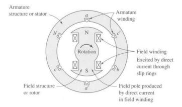
Figure A.1 Elementary two-pole, three-phase generator.
