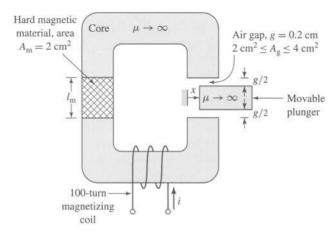
**Figure 1.22** Magnetic circuit for Example 1.11.
