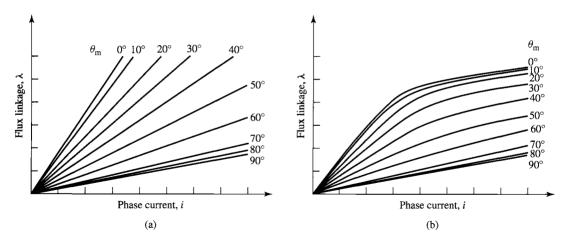
**Figure 8.13** Plots of  $\lambda$  versus *i* for a VRM with (a) linear and (b) nonlinear magnetics.
