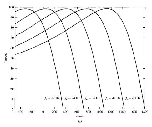
**Figure 11.18** A family of typical induction-motor speed-torque curves for a four-pole motor for various values of the electrical supply frequency. (a)  $R_1$  sufficiently small so that its effects are negligible. (b)  $R_1$  not negligible.
