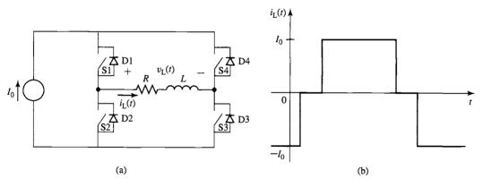
Figure 10.43 (a) H-bridge inverter configuration fed by a current source. (b) Typical stepped load-current waveform
