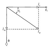
**Figure 2.5** No-load phasor diagram.
