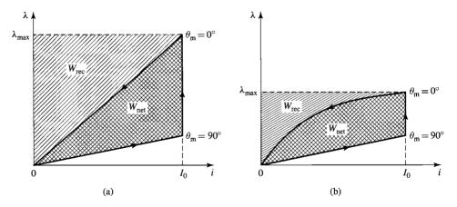
**Figure 8.14** (a) Flux-linkage-current trajectory for the (a) linear and (b) nonlinear machines of Fig. 8.13.
