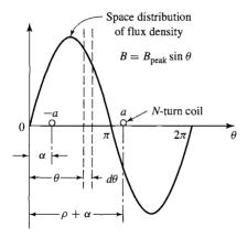
**Figure B.4** Fractional-pitch coil in sinusoidal field.
