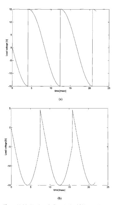
**Figure 10.34** Waveforms for Example 10.7. (a) Magnet-voltage for  $\alpha_{\rm d}=87.4^{\circ}$ ,  $V_{\rm dc}=0.438$  V. (b) Magnet-voltage for  $\alpha_{\rm d}=162^{\circ}$ ,  $V_{\rm dc}=-9.1$  V.
