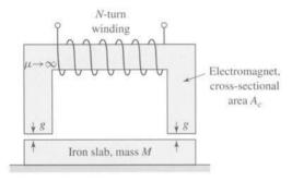
**Figure 3.30** Electromagnet lifting an iron slab (Problem 3.14).
