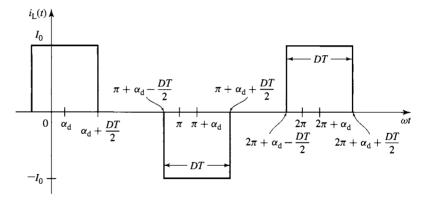
Figure 10.58 Stepped current waveform for Problem 10.20.
