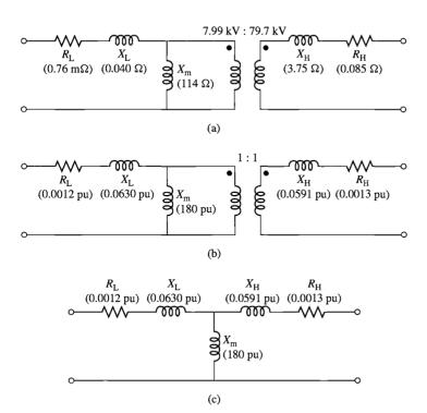
**Figure 2.22** Transformer equivalent circuits for Example 2.12. (a) Equivalent circuit in actual units. (b) Per-unit equivalent circuit with 1:1 ideal transformer. (c) Per-unit equivalent circuit following elimination of the ideal transformer.
