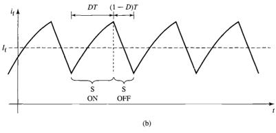
**Figure 11.2** (a) Pulse-width modulation system for a dc-machine field winding. (b) Field-current waveform.
