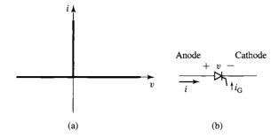
**Figure 10.5** (a) Idealized SCR *v-i* characteristic. (b) SCR symbol.
