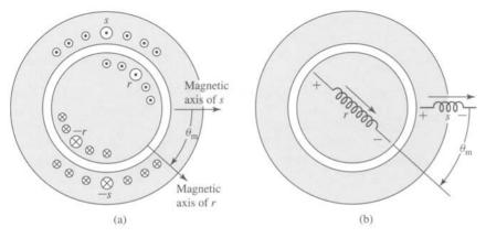
**Figure 4.34** Elementary two-pole machine with smooth air gap: (a) winding distribution and (b) schematic representation.
