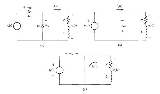
**Figure 10.21** (a) Half-wave rectifier with an inductive load and a free-wheeling diode. (b) Equivalent circuit when  $v_s(t) > 0$  and diode D1 is conducting. (c) Equivalent circuit when  $v_s(t) < 0$  and the free-wheeling diode D2 is conducting.
