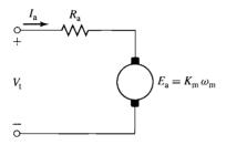
**Figure 7.20** Equivalent circuit of a permanent-magnet dc motor.
