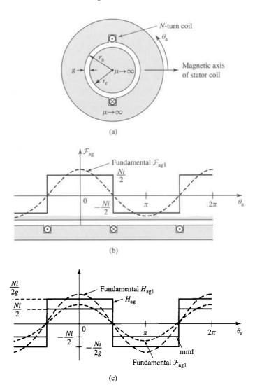
**Figure 4.25** The air-gap mmf and radial component of  $H_{ag}$  for a concentrated full-pitch winding.
