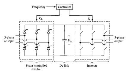
Figure 11.11 Three-phase voltage-source inverter.
