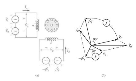
**Figure 9.13** Synthesis of an unbalanced two-phase system from the sum of two balanced systems of opposite phase sequence.
