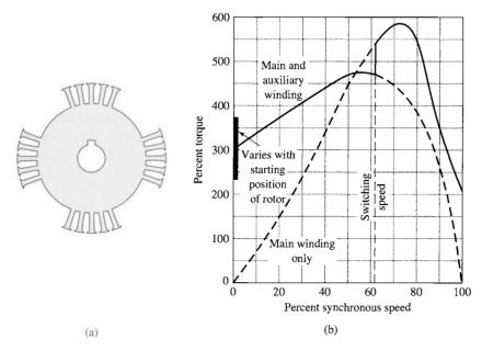
**Figure 9.9** Rotor punching for four-pole synchronous-reluctance motor and typical torque-speed characteristic.
