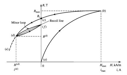
**Figure 1.21** Portion of a *B-H* characteristic showing a minor loop and a recoil line.
