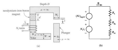
**Figure 3.22** (a) Actuator for Example 3.9. (b) Equivalent circuit for the actuator with the permanent magnet replaced by linear material and an equivalent winding carrying (Ni)<sub>equiv</sub> ampere-turns.
