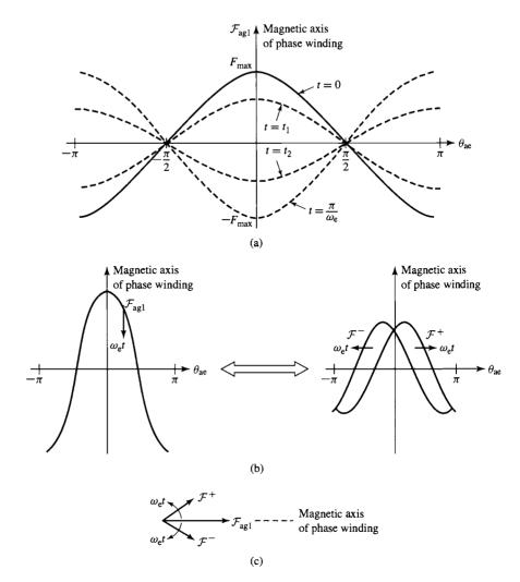
**Figure 4.28** Single-phase-winding space-fundamental air-gap mmf: (a) mmf distribution of a single-phase winding at various times; (b) total mmf  $\mathcal{F}_{ag1}$  decomposed into two traveling waves  $\mathcal{F}^-$  and  $\mathcal{F}^+$ ; (c) phasor decomposition of  $\mathcal{F}_{ag1}$ .
