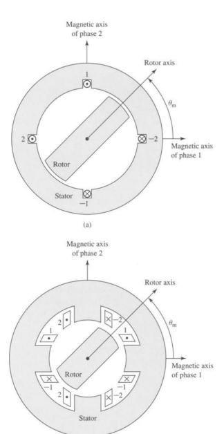
**Figure 8.1** Basic two-phase VRMs: (a) singly-salient and (b) doubly-salient.
