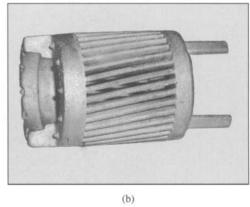
**Figure 6.3** (a) The rotor of a small squirrel-cage motor. (b) The squirrel-cage structure after the rotor laminations have been chemically etched away. (*Athens Products*.)
