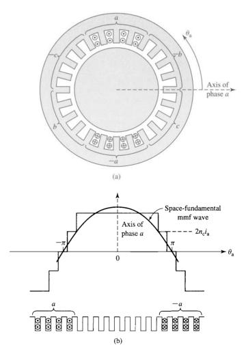
**Figure 4.20** The mmf of one phase of a distributed two-pole, three-phase winding with full-pitch coils.
