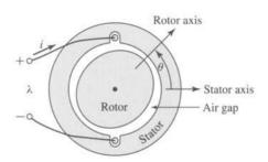
**Figure 3.9** Magnetic circuit for Example 3.4.
