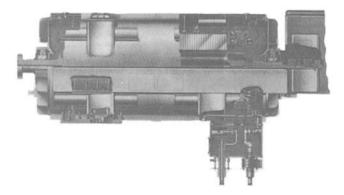
**Figure D.2** Cutaway view of a two-pole 3600 r/min turbine rated at 500 MVA, 0.90 power factor, 22 kV, 60 Hz, 45 psig H<sub>2</sub> pressure. Stator winding is water-cooled; rotor winding is hydrogen-cooled. (*General Electric Company.*)
