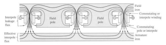
Figure 7.21 Interpoles and their associated component flux.
