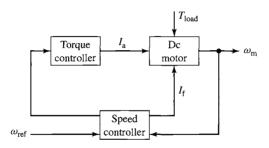
**Figure 11.10** Block diagram of a dc-motor speed-control system using direct-control of motor torque.
