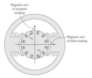
Figure 4.22 Cross section of a two-pole dc machine.
