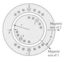
**Figure B.9** Two distributed windings separated by electrical angle  $\alpha$ .
