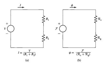
**Figure 1.3** Analogy between electric and magnetic circuits. (a) Electric circuit, (b) magnetic circuit.
