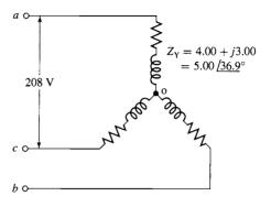
Figure A.13 Circuit for Example A.2.
