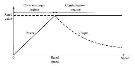
Figure 11.12 Variable-speed operating regimes for a synchronous motor.
