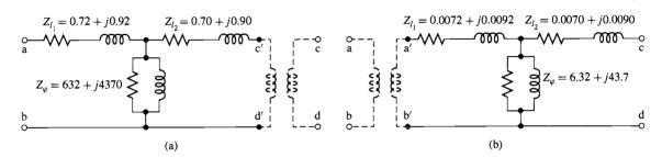
**Figure 2.11** Equivalent circuits for transformer of Example 2.3 referred to (a) the high-voltage side and (b) the low-voltage side.
