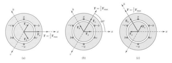
**Figure 4.31** The production of a rotating magnetic field by means of three-phase currents.
