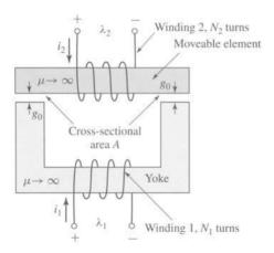
**Figure 3.36** Two-winding magnetic circuit for Problem 3.22.
