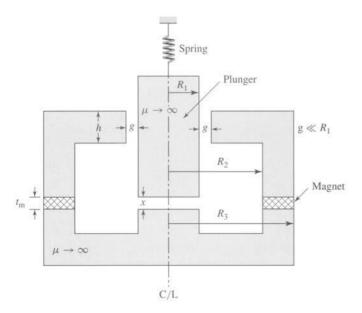
Figure 3.40 Permanent-magnet system for Problem 3.29.
