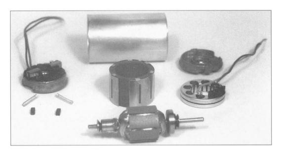
**Figure 7.16** Disassembled permanent-magnet dc motor. A permanent-magnet ac tachometer is also included in the same housing for speed control. (*Buehler Products Inc.*)
