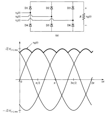
**Figure 10.36** (a) Three-phase, six-pulse diode bridge with resistive load. (b) Line-to-line voltages and resistor voltage.
