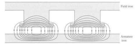
Figure 7.10 Flux with only the armature excited and brushes on neutral.
