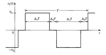
**Figure 10.42** Typical output-voltage waveform for the H-bridge of Fig. 10.40.
