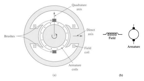
Figure 7.1 Schematic representations of a dc machine.
