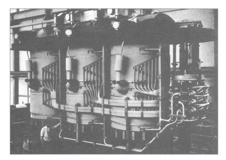
**Figure 2.20** A 200-MVA, three-phase, 50-Hz, three-winding, 210/80/10.2-kV transformer removed from its tank. The 210-kV winding has an on-load tap changer for adjustment of the voltage. (*Brown Boveri Corporation*.)
