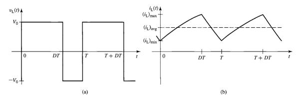
Figure 10.46 Typical (a) voltage and (b) current waveform under PWM operation.
