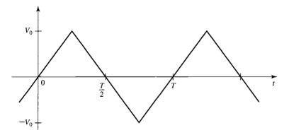
Figure 10.50 Triangular voltage waveform.
