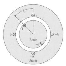
**Figure 4.45** Elementary cylindrical-rotor, two-phase synchronous machine for Problem 4.22.
