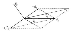
**Figure 9.14** Resolution of unbalanced two-phase voltages into symmetrical components.
