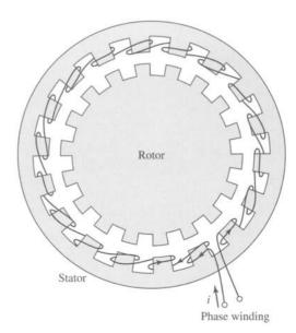
**Figure 8.17** Diagram of one stack and phase of a multiphase, multistack variable-reluctance stepping motor, such as that in Fig. 8.16. For an  $n_s$ -stack motor, the rotor or stator (but not both) on each stack is displaced by  $1/n_s$  times the pole pitch.
