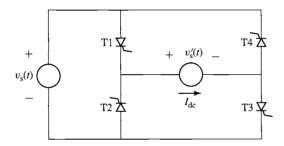
**Figure 10.55** Full-wave, phase-controlled rectifier for Problem 10.11.
