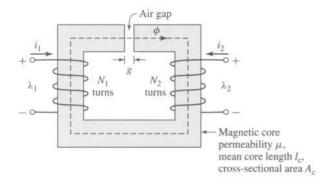
Figure 1.8 Magnetic circuit with two windings.
