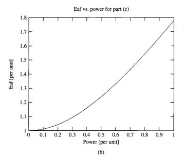
**Figure 5.13** Example 5.6. (a) MATLAB plot of terminal voltage vs.  $\delta$  for part (b). (b) MATLAB plot of  $E_{\rm af}$  vs. power for part (c).
