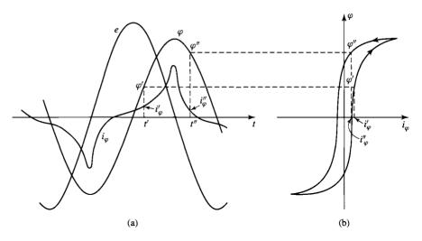
**Figure 1.11** Excitation phenomena. (a) Voltage, flux, and exciting current; (b) corresponding hysteresis loop.
