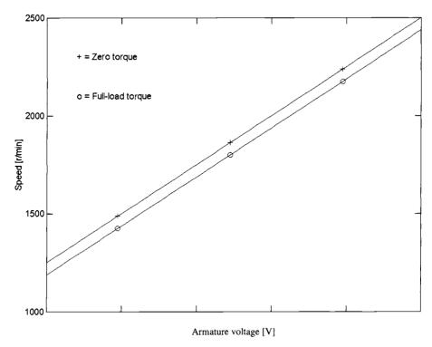
Figure 11.5 A plot of speed versus armature voltage for the dc motor of Example 11.3.
