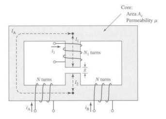
Figure 1.33 Symmetric magnetic circuit for Problem 1.23.
