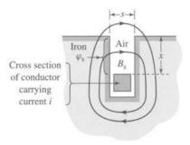
**Figure 3.31** Conductor in a slot (Problem 3.17).
