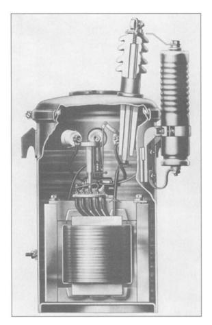
**Figure 2.2** Cutaway view of self-protected distribution transformer typical of sizes 2 to 25 kVA, 7200:240/120 V. Only one high-voltage insulator and lightning arrester is needed because one side of the 7200-V line and one side of the primary are grounded. (*General Electric Company.*)
