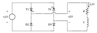
**Figure 10.54** Full-wave, phase-controlled rectifier system for Problem 10.10.
