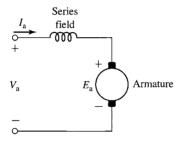
**Figure 7.25** Series-connected universal machine.
