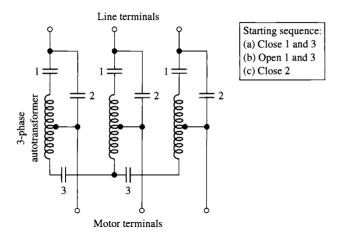
**Figure 6.22** Connections of a one-step starting autotransformer
