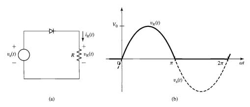
Figure 10.3 (a) Half-wave rectifier circuit for Example 10.1. (b) Resistor voltage.
