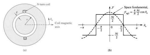
Figure B.8 (a) N-turn concentrated coil and (b) resultant mmf.
