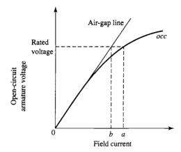
**Figure 5.5** Open-circuit characteristic of a synchronous machine.
