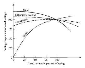
Figure 7.5 Volt-ampere characteristics of dc generators.
