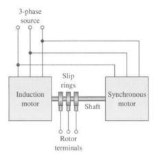
**Figure 6.23** Interconnected induction and synchronous machines (Problems 6.7 and 6.8).
