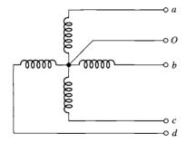
**Figure A.16** A five-wire, four-phase system.
