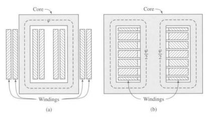
**Figure 2.1** Schematic views of (a) core-type and (b) shell-type transformers.
