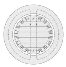
**Figure 4.8** Elementary two-pole cylindrical-rotor field winding.
