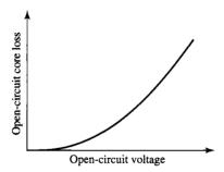
**Figure 5.6** Typical form of an open-circuit core-loss curve.
