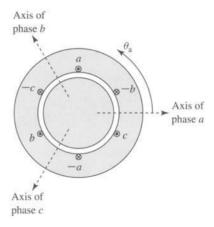
**Figure 4.29** Simplified two-pole three-phase stator winding.
