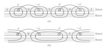
Figure 11.16 Principles of the pole-changing winding.
