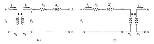
**Figure 2.8** Equivalent circuits for Example 2.2. (a) Impedance in series with the secondary. (b) Impedance referred to the primary.
