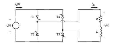
Figure 10.31 Full-wave, phase-controlled SCR bridge.
