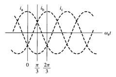
**Figure 4.30** Instantaneous phase currents under balanced three-phase conditions.
