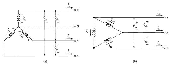
**Figure A.5** Three-phase connections: (a) Y connection and (b)  $\Delta$  connection.
