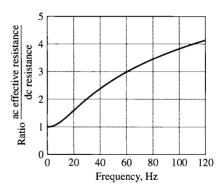
**Figure 6.19** Skin effect in a copper rotor bar 2.5 cm deep.
