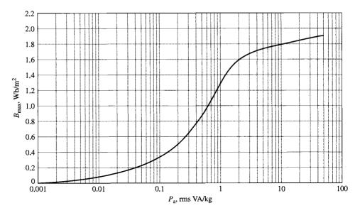
**Figure 1.12** Exciting rms voltamperes per kilogram at 60 Hz for M-5 grain-oriented electrical steel 0.012 in thick. (*Armco Inc.*)
