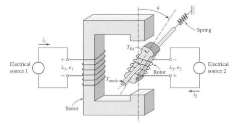
Figure 3.15 Multiply-excited magnetic system for Example 3.7.
