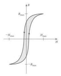
**Figure 1.13** Hysteresis loop; hysteresis loss is proportional to the loop area (shaded).
