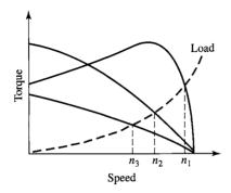
**Figure 11.20** Speed control by means of rotor resistance.
