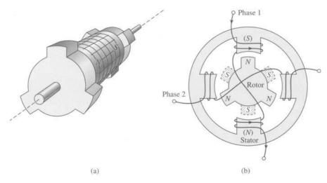
**Figure 8.21** Schematic view of a hybrid stepping motor. (a) Two-stack rotor showing the axially-directed permanent magnet and the pole pieces displaced by one-half the pole pitch. (b) End view from the rotor north poles and showing the rotor south poles at the far end (shown crosshatched). Phase 1 of the stator is energized to align the rotor as shown.
