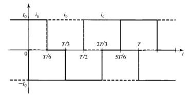
**Figure 10.49** Three-phase stepped current waveform for Example 10.14.
