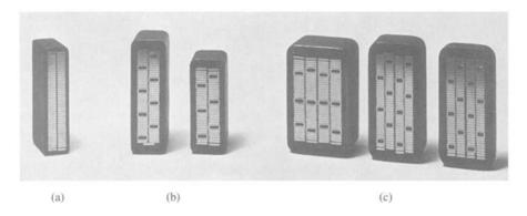
**Figure D.1** Cross sections of bars for two-layer stator windings of turbine-generators. Insulation system consists of synthetic resin with vacuum impregnation. (a) Indirectly cooled bar with tubular strands; (b) water-cooled bars, two-wire-wide mixed strands, (c) water-cooled bars, four-wire-wide mixed strands. (*Brown Boveri Corporation*.)
