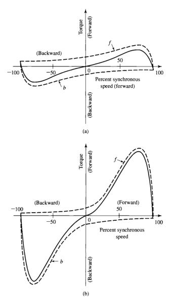
**Figure 9.2** Torque-speed characteristic of a single-phase induction motor (a) on the basis of constant forward and backward flux waves, (b) taking into account changes in the flux waves.
