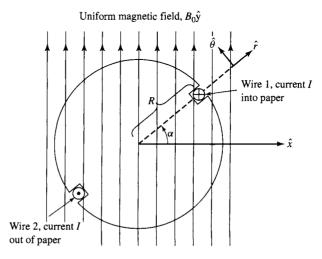
Figure 3.2 Single-coil rotor for Example 3.1.
