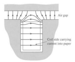
**Figure 4.41** Flux created by a single coil side in a slot.
