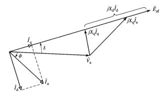
Figure 5.25 Generator phasor diagram for Example 5.9.
