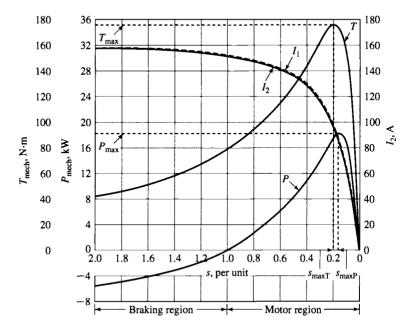
**Figure 6.15** Computed torque, power, and current curves for the 7.5-kW motor in Examples 6.2 and 6.3.
