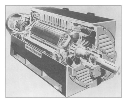
**Figure 4.13** Cutaway view of a high-speed synchronous motor. The excitor shown on the left end of the rotor is a small ac generator with a rotating semiconductor rectifier assembly. (*General Electric Company*.)
