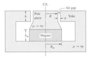
**Figure 1.37** Magnetic circuit for the loudspeaker of Problem 1.34 (voice coil not shown).
