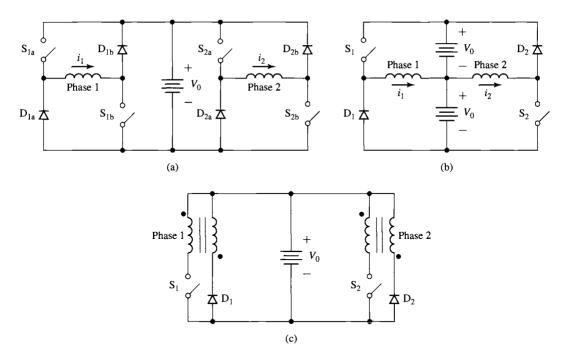
**Figure 11.23** Inverter configurations. (a) Two-phase inverter which uses two switches per phase. (b) Two-phase inverter which uses a split supply and one switch per phase. (c) Two-phase inverter with bifilar phase windings and one switch per phase.
