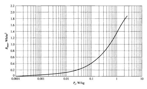
**Figure 1.14** Core loss at 60 Hz in watts per kilogram for M-5 grain-oriented electrical steel 0.012 in thick. (*Armco Inc.*)
