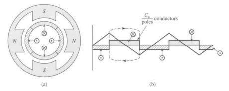
Figure 4.24 (a) Cross section of a four-pole dc machine; (b) development of current sheet and mmf wave.
