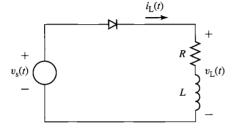
**Figure 10.19** Half-wave rectifier with an inductive load.
