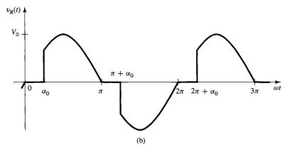
**Figure 10.10** (a) Gate pulses for Example 10.3. (b) Resistor voltage.
