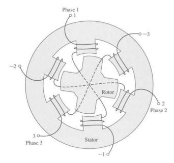
Figure 8.5 Cross-sectional view of a 6/4 three-phase VRM.
