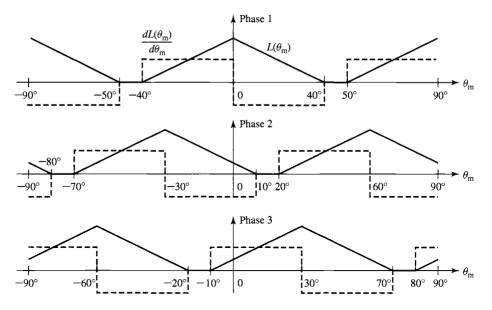
**Figure 8.9** Idealized inductance and  $dL/d\theta_{\rm m}$  curves for a three-phase 6/4 VRM with 40° rotor and stator poles.
