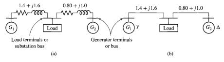
Figure A.15 Examples of single-line diagrams.
