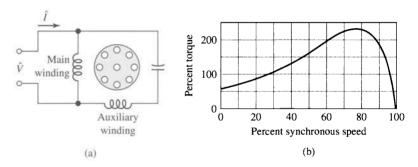
**Figure 9.6** Permanent-split-capacitor motor and typical torque-speed characteristic.
