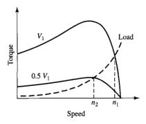
**Figure 11.19** Speed control by means of line voltage.
