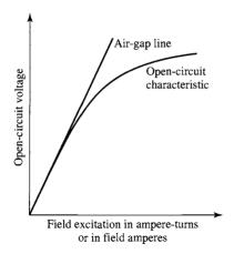
**Figure 4.37** Typical open-circuit characteristic and air-gap line.
