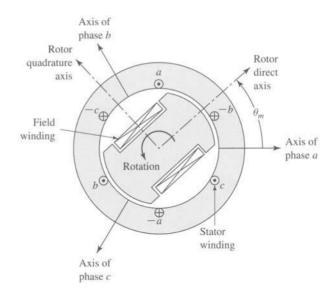
Figure C.1 Idealized synchronous machine
