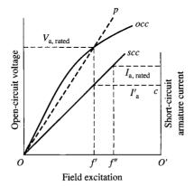
**Figure 5.9** Open- and short-circuit characteristics showing equivalent magnetization line for saturated operating conditions.
