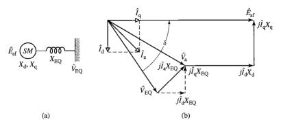
**Figure 5.26** Salient-pole synchronous machine and series impedance: (a) single-line diagram and (b) phasor diagram.
