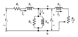
**Figure 6.9** Single-phase equivalent circuit for a polyphase induction motor.
