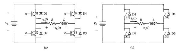
**Figure 10.40** Single-phase H-bridge inverter configuration. (a) Typical configuration using IGBTs. (b) Generic configuration using ideal switches.
