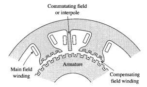
**Figure 7.22** Section of dc machine showing compensating winding.
