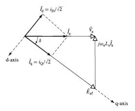
**Figure 11.14** Phasor diagram for unity-power-factor field-oriented-control algorithm.
