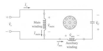
**Figure 9.17** Permanent-split-capacitor induction-motor connections for Example 9.5.
