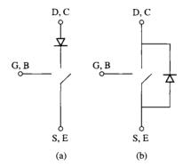
**Figure 10.13** (a) Ideal-switch model for a MOSFET or an IGBT showing the series ideal diode which represents the unidirectional-current device characteristic. (b) Ideal-switch model for devices which include a reverse-biased protection diode. The symbols G, D, and S apply to the MOSFET while the symbols B, C, and E apply to the IBGT.
