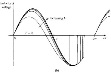
**Figure 10.20** Effect of increasing the series inductance in the circuit of Fig. 10.19 on (a) the load current and (b) the inductor voltage.
