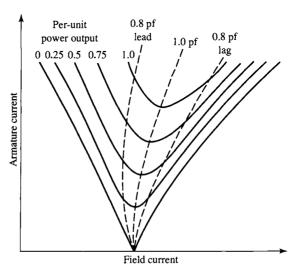
**Figure 5.18** Typical form of synchronous-generator V curves.
