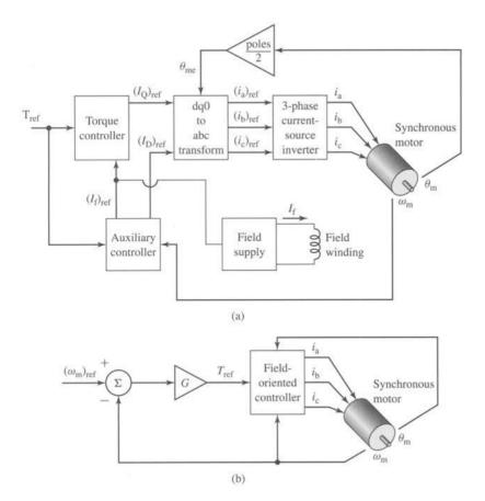
**Figure 11.13** (a) Block diagram of a field-oriented torque-control system for a synchronous motor. (b) Block diagram of a synchronous-motor speed-control loop built around a field-oriented torque control system.
