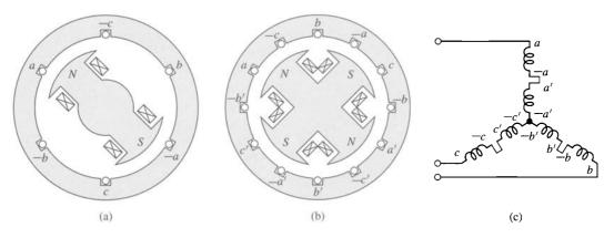
**Figure 4.12** Schematic views of three-phase generators: (a) two-pole, (b) four-pole, and (c) *Y* connection of the windings.
