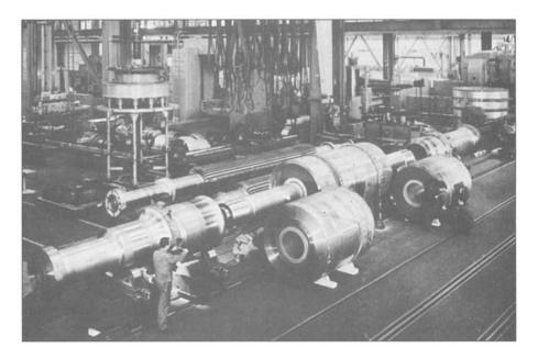
**Figure 4.11** Parts of multipiece rotor for a 1333-MVA three-phase 1800 r/min turbine generator. The separate forgings will be shrunk on the shaft before final machining and milling slots for the windings. The total weight of the rotor is 435,000 lb. (*Brown Boveri Corporation.*)
