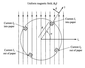
Figure 3.25 Two-coil rotor for Problem 3.1.
