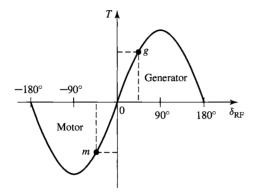
**Figure 5.1** Torque-angle characteristic.
