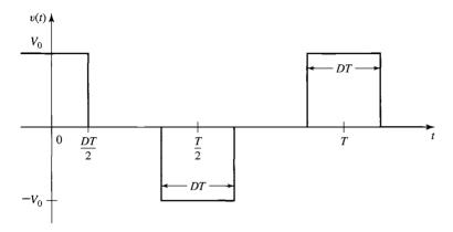
Figure 10.57 Stepped voltage waveform for Problem 10.18.
