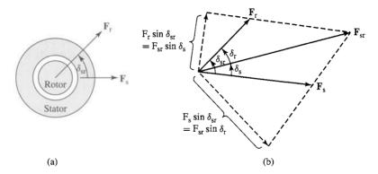
**Figure 4.35** Simplified two-pole machine: (a) elementary model and (b) vector diagram of mmf waves. Torque is produced by the tendency of the rotor and stator magnetic fields to align. Note that these figures are drawn with  $\delta_{sr}$  positive, i.e., with the rotor mmf wave  $\mathbf{F}_r$  leading that of the stator  $\mathbf{F}_s$ .
