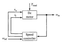
**Figure 11.7** Block diagram for a speed-control system for a separately excited or shunt-connected do motor.
