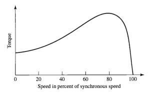
**Figure 4.15** Typical induction-motor speed-torque characteristic
