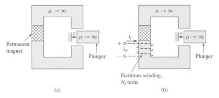
**Figure 3.17** (a) Magnetic circuit with permanent magnet and movable plunger; (b) fictitious winding added.
