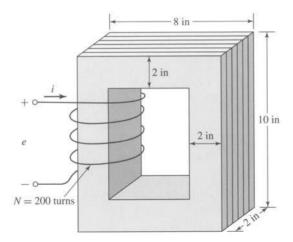
**Figure 1.15** Laminated steel core with winding for Example 1.8.
