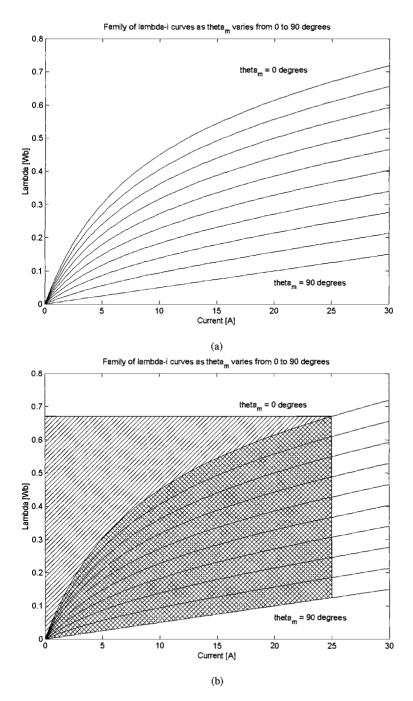
**Figure 8.15** (a)  $\lambda_1$ - $i_1$  curves for Example 8.4. (b) Areas used in the calculation of part (b).
