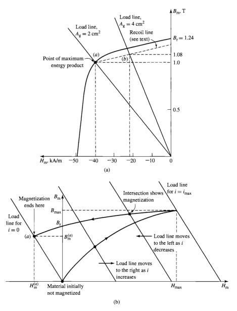
**Figure 1.23** (a) Magnetization curve for Alnico 5 for Example 1.11; (b) series of load lines for  $A_{\rm g}=2~{\rm cm^2}$  and varying values of i showing the magnetization procedure for Example 1.11.
