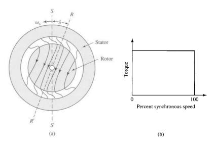
**Figure 9.10** (a) General nature of the magnetic field in the air gap and rotor of a hysteresis motor; (b) idealized torque-speed characteristic.
