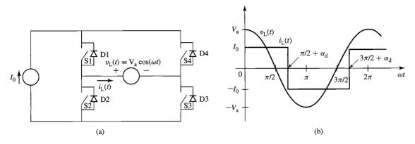
Figure 10.44 (a) Current-source inverter for Example 10.12. (b) Load-current waveform.
