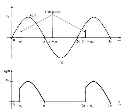
Figure 10.7 (a) Gate pulses for Example 10.2. (b) Resistor voltage.
