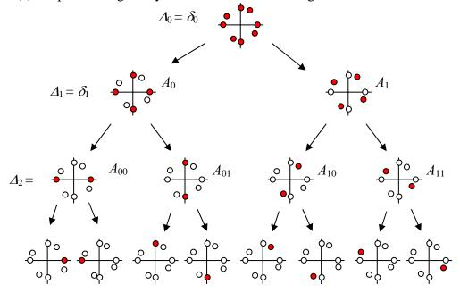
(b) If the minimum Euclidean distance between parallel transitions is given by  $\Delta_{\tilde{m}+1}$  and the minimum Euclidean distance between non-parallel paths of the trellis is given by  $d_{free}(\tilde{m})$ , the free Euclidean distance of the TCM encoder is
