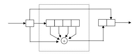
(i) There are  $2^4 = 16$  states for this encoder. The state transitions and the output is given in the table below.
