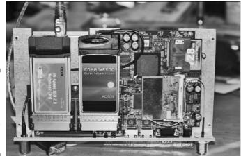
Figure 11-7: The insides of a completed Stompbox EV-D0/Wi-Fi router.
