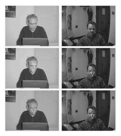
**Figure 8.6** (Top) Detections from step I. (Middle) Detections from step II. (Bottom) Detections remaining after final classifier. Detection triangles—mapping of the reference points into the image by *a*.
