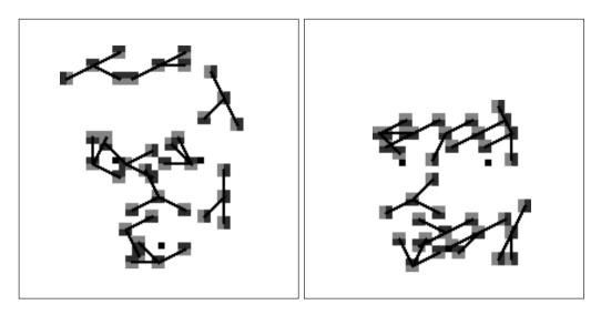
**Figure 6.9** The graphs representing local features identified for the sparse face model. Each local feature has a center edge and three other edges around it. The two adjacent rectangles describe the orientation and polarity of each edge.
