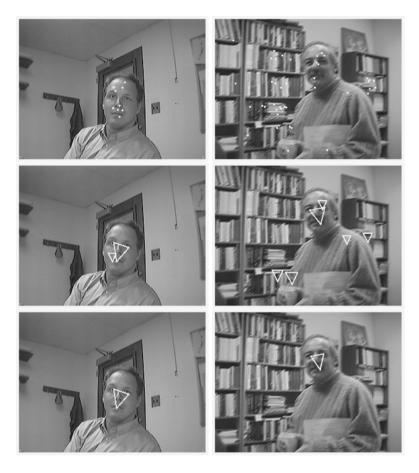
**Figure 8.5** (Top) Detections from step I. (Middle) Detections from step II. (Bottom) Detections remaining after final classifier. Detection triangles—mapping of the reference points into the image by *a*.
