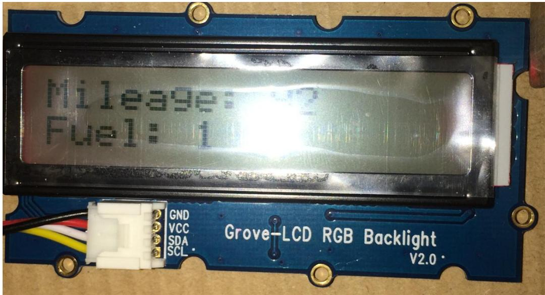
**Figure 13** LCD interfaced with Arduino
