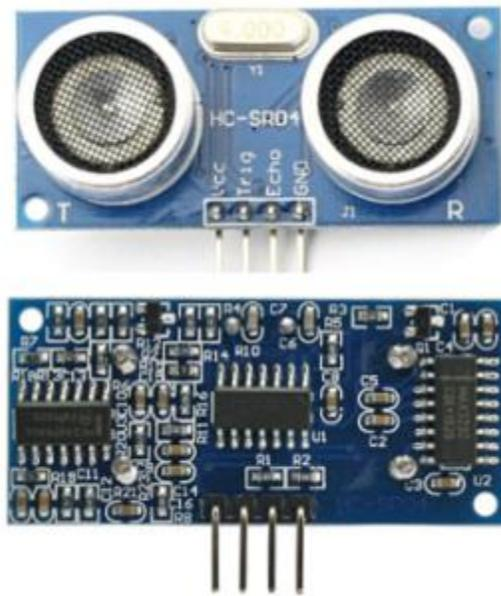
Figure 11 HC-SR04 Ultrasonic Sensor
