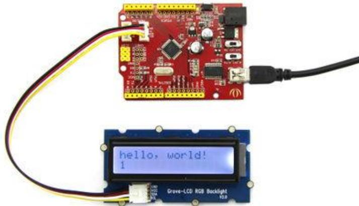
Figure 20 Connections from LCD to Arduino board
