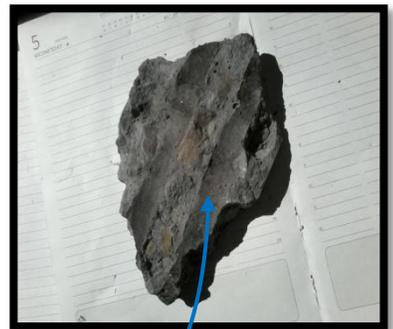
Smooth concrete surface indicating poor bond between reinforcement & concrete.
