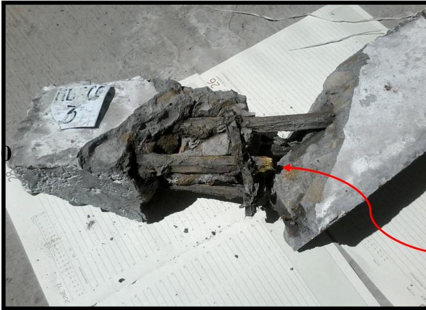
Breaking of tensile reinforcement at node, indicates ductile failure of beam
