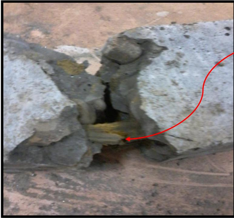
Splitting of tensile reinforcement at node, indicates ductile failure of beam-BSRCC:3
