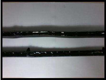
Bamboo Splints coated with bitumen & sand mixture
