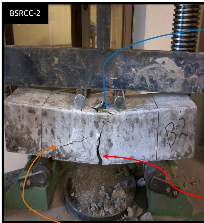
Crushing of concrete
