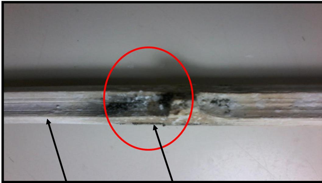
Deposition of Calcium layer on the surface
