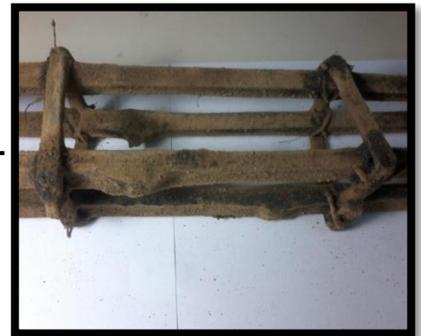
Steel wires used for connecting stirrups
