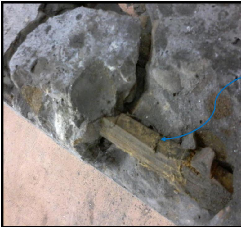
Making grooves on the inner surface of bamboo splint helped in maintaining the structural integrity and enhanced the concrete-bamboo bond to a fair amount.
