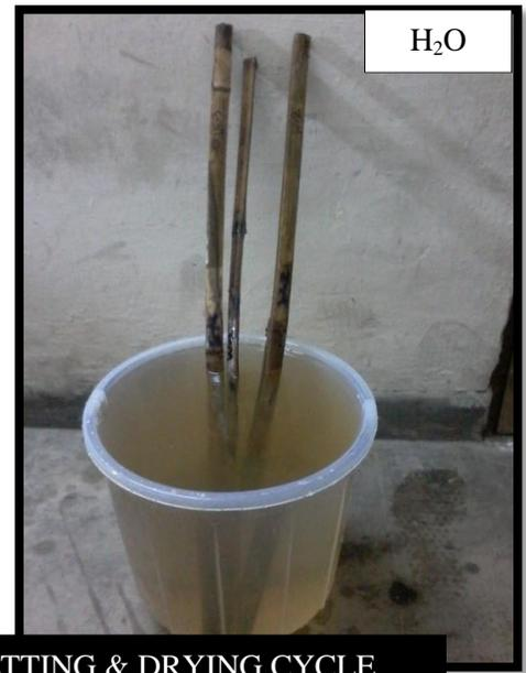
SAMPLES AFTER UNDERGOING 60 DAYS OF ALTERNATE WETTING & DRYING CYCLE
