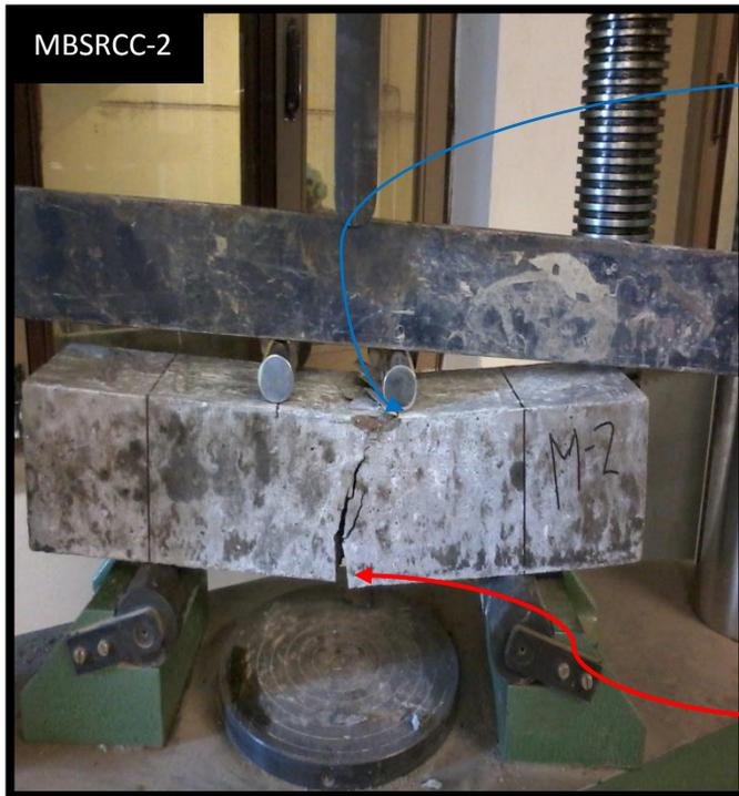
Crushing of concrete
