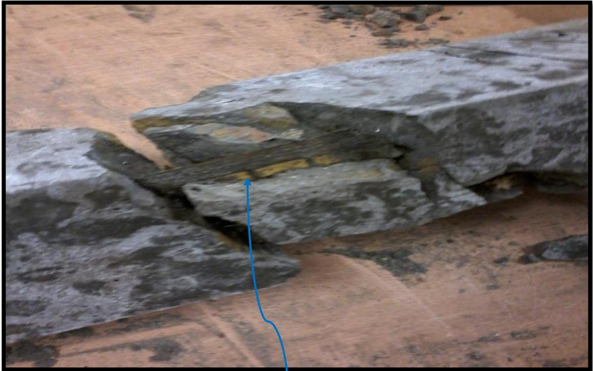
In case of MBRCC beams the grooves got filled up by bitumen+sand mixture making them ineffective in enhancing the concrete bamboo bond resulting in poor transfer of stresses between the two, because of this, splitting of bamboo did not occurred in any of the MBRCC beams.
