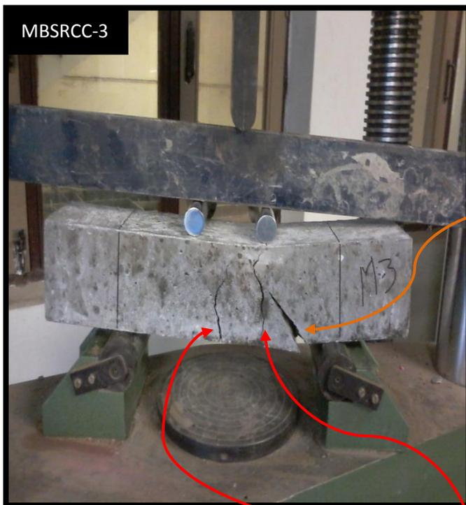
Web Shear crack
