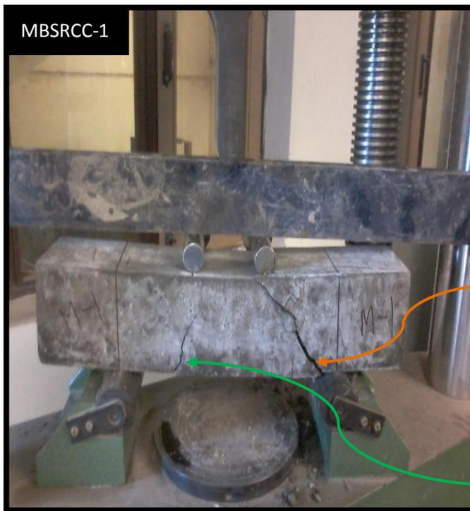
Web Shear crack
