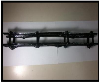
Bamboo Splints coated with bitumen & sand mixture
