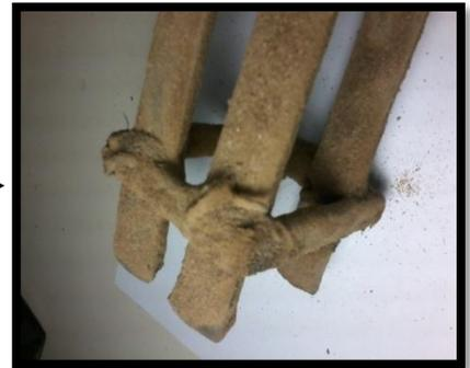
Sand being applied over wet bitumen & sand mixture
