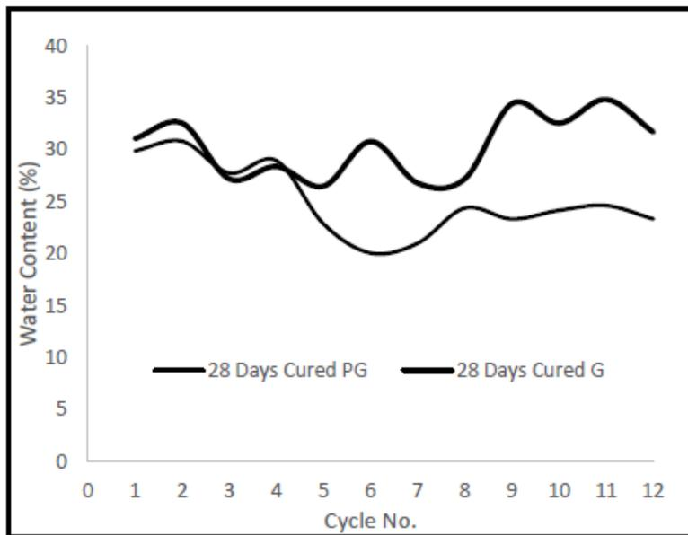
Figure 4.19 (c) – Water content plots for durability cycles with G and PG (28 days)
