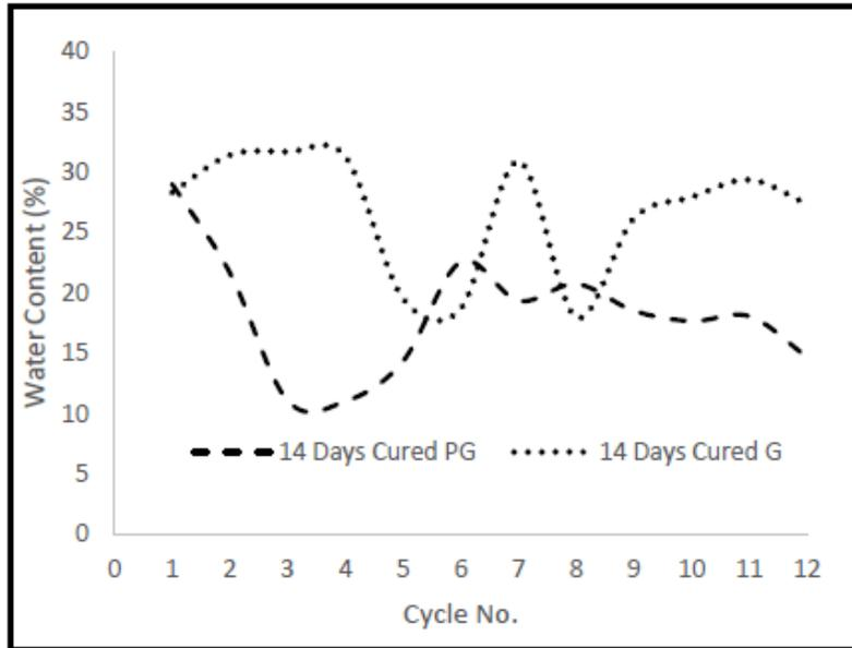
Figure 4.19 (b) – Water content plots for durability cycles with G and PG (14 days)
