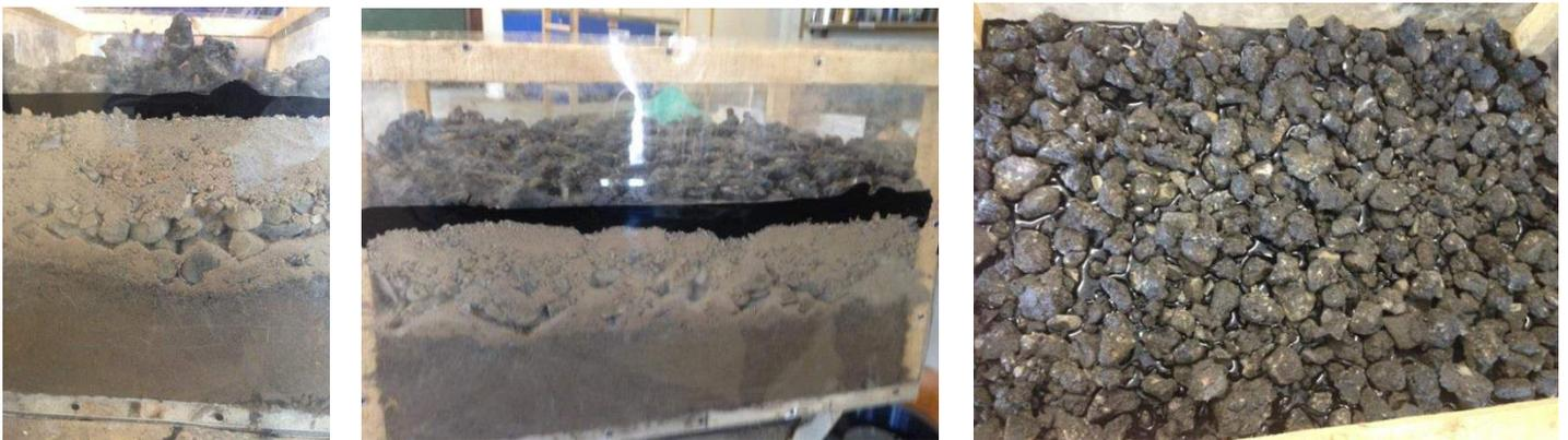
*Figure 3.20 – Laying of first layer of surface course consisting of bigger aggregates mixed with hot bitumen*
