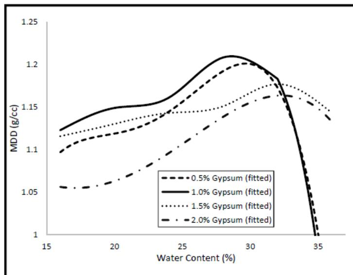
Figure 4.1 - Measurement of OMC and MDD of Fly ash + 8% Lime and varying Gypsum Content for Reference mix Preparation
