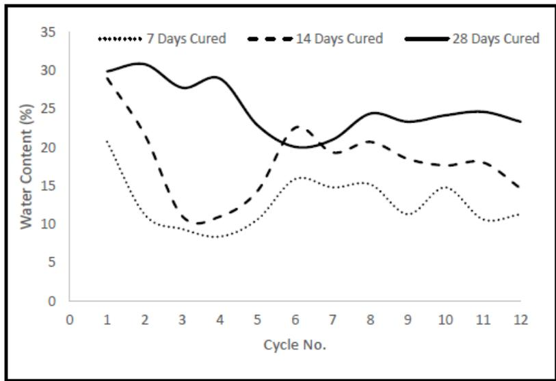
Figure 4.11 – Variation of water content with durability cycle for Phosphogypsum (PG)
