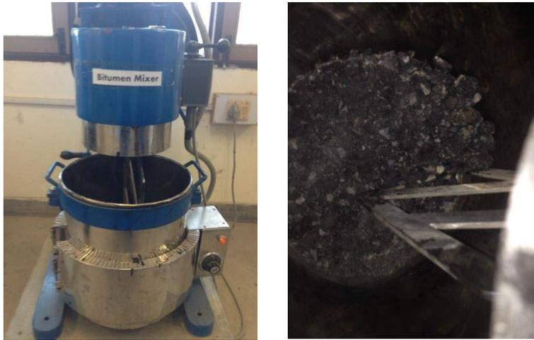
*Figure 3.19 – Mixing of aggregates with hot bitumen*
