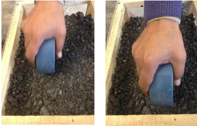
*Figure 3.22 – Compaction of surface course*
