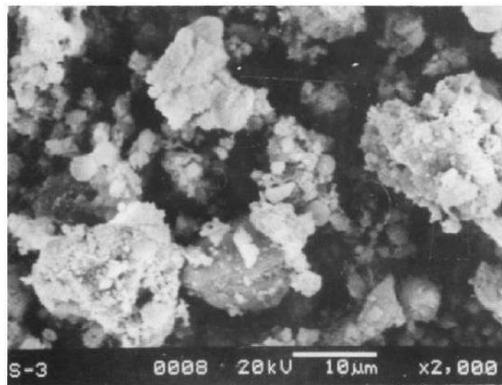
*Figure 4.22 – SEM photograph of Fly Ash + Lime (8%) + Gypsum (1%) cured sample at 28 days (illustrative purpose only)*
