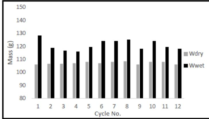
Figure 4.8 – Data of 7 days cured sample for durability cycles for Phosphogypsum (PG)
