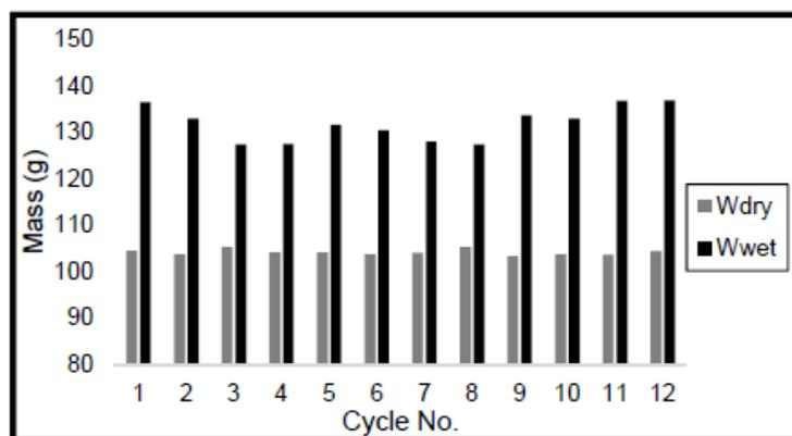
Figure 4.7 - Data of 28 Days Cured sample for Durability Cycles for Gypsum (G)
