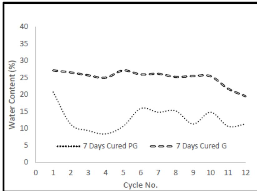
*Figure 4.19 (a) – Water content plot for durability cycles with G and PG (7 days)*
