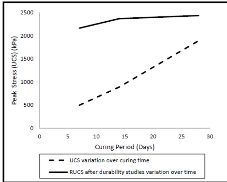
Figure 4.14 – Variation of Unconfined Compressive Strength over curing time for Gypsum (G)
