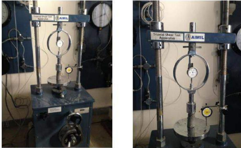
*Figure 3.3 – Setup for Unconfined Compressive Strength (UCS) measurement*
