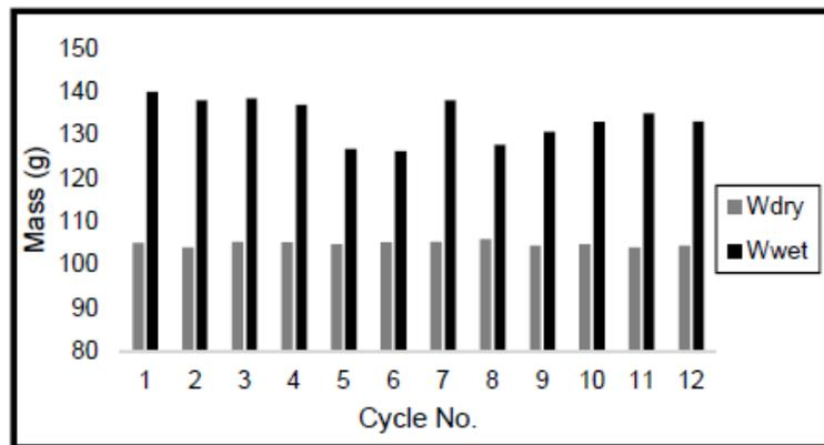
Figure 4.6 - Data of 14 Days Cured sample for Durability Cycles for Gypsum (G)
