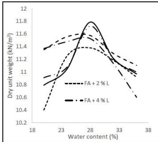
Figure 4.2 (a) – Compaction test plots for fly ash and varying lime (L) content
