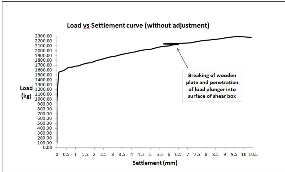
Figure 4.25 (a) – Load v/s settlement curve (without adjustment) for PM 1
