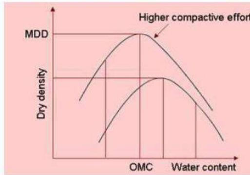
Figure 3.2 - Dry Density v/s Water Content with increasing Compactive effort
