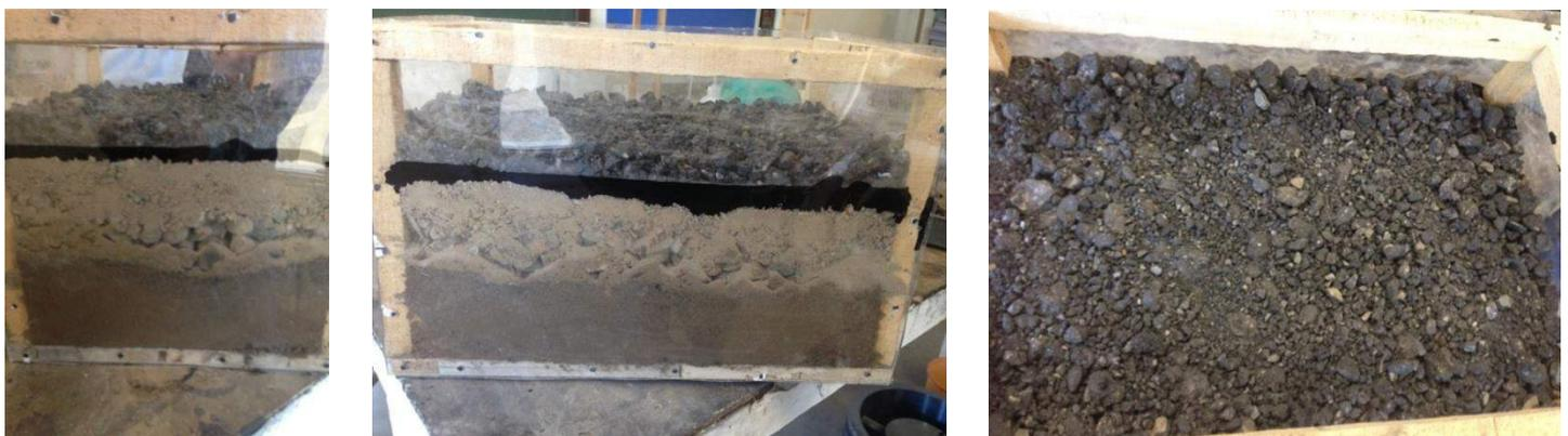
*Figure 3.21 – Laying of second layer of surface course consisting of smaller aggregates mixed with hot bitumen*
