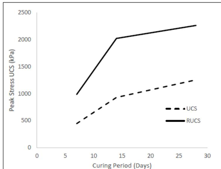
Figure 4.15 – Variation of Unconfined Compressive Strength over curing time for Phosphogypsum (PG)
