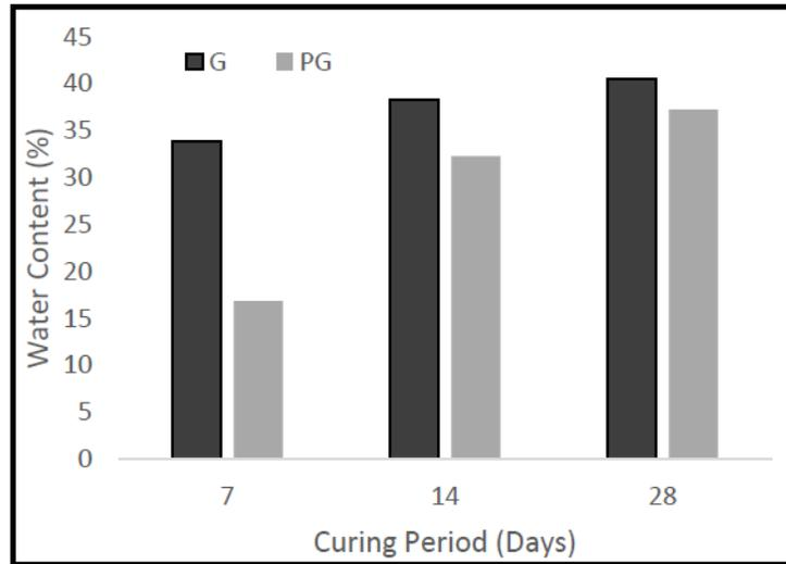
Figure 4.17 – Water content measurement just after curing
