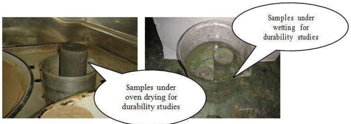
*Figure 3.7 – Setup for drying-wetting cycles*
