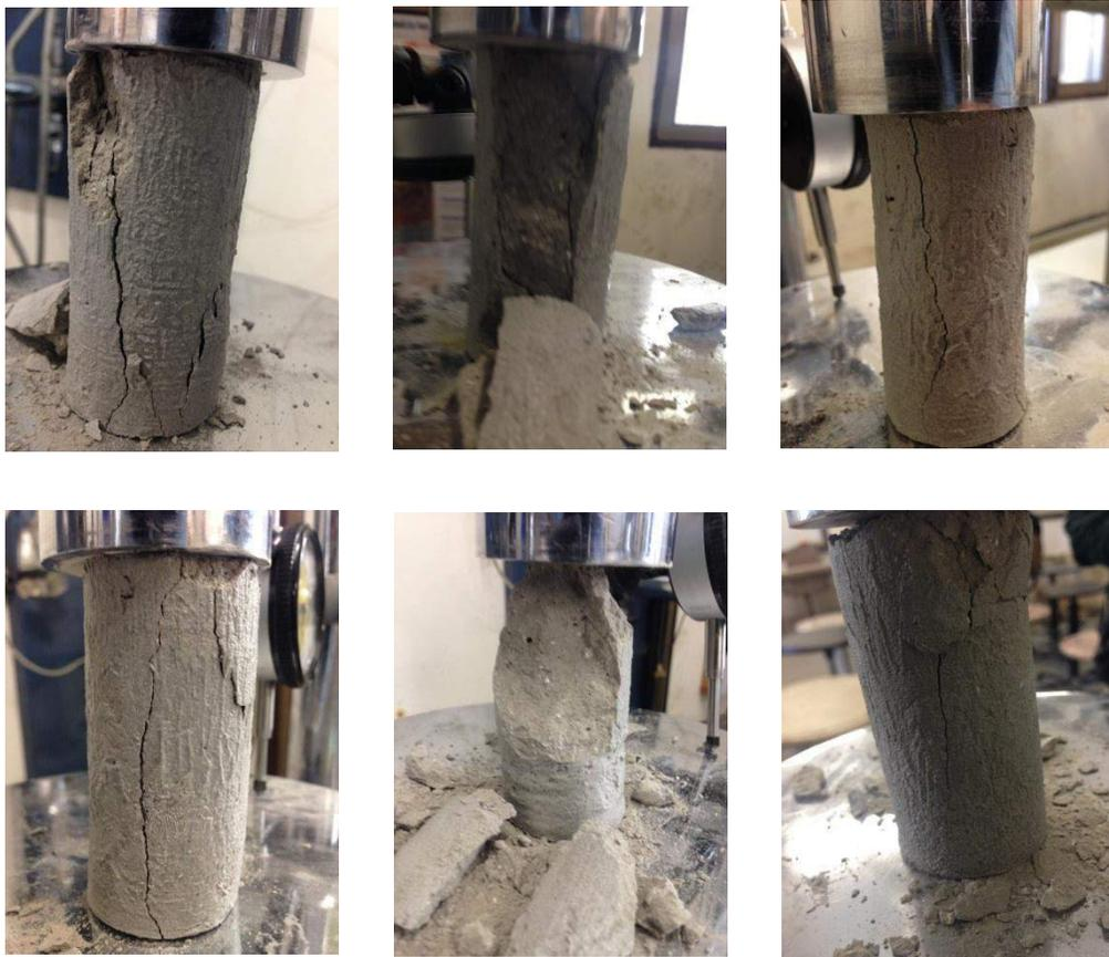
*Figure 4.20 (b) – Samples under UCS (top) and RUCS (bottom) for Posphogypsum (PG) modifier*
