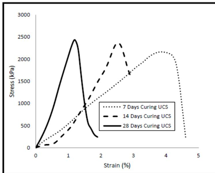
Figure 4.12 - UCS Plots of 7, 14 and 28 days cured samples for Gypsum (G)
