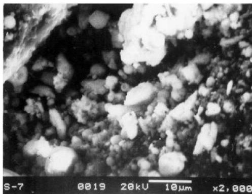
*Figure 4.23 – SEM photograph of Fly Ash + Lime (8%) + Phosphogypsum (2%) cured sample at 28 days (illustrative purpose only)*
