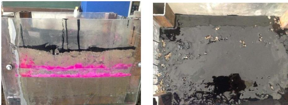
*Figure 3.31 – Tack coat on binder layer*
