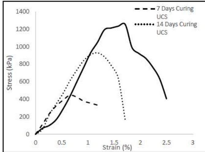
Figure 4.4 – UCS plots of 7, 14 and 28 days cured samples for Phosphogypsum (PG)
