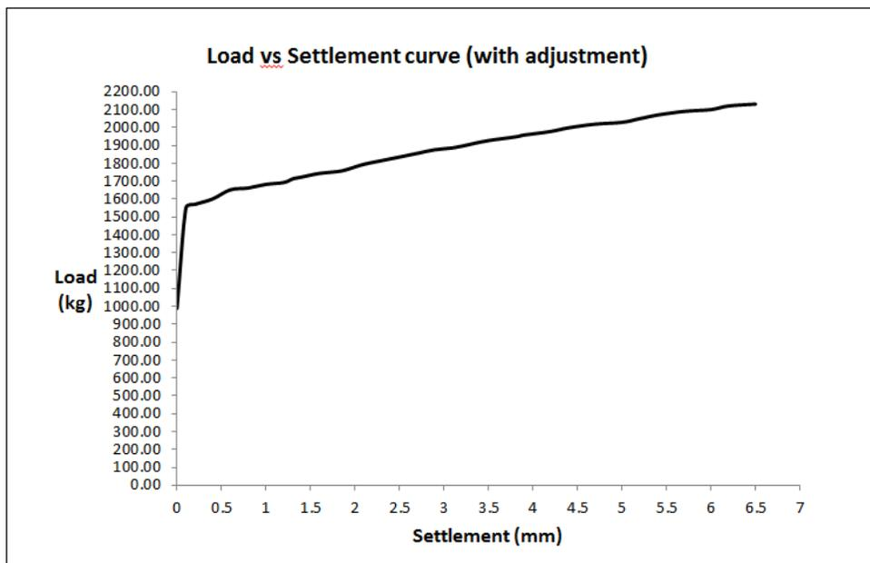
Figure 4.25 (b) – Load v/s settlement curve (with adjustment) for PM 1
