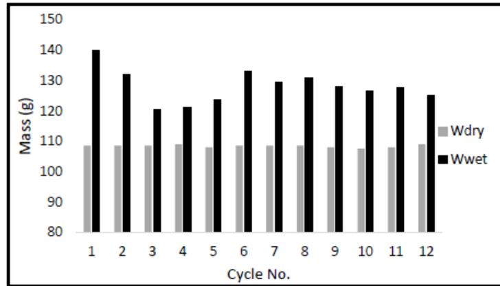
Figure 4.9 – Data of 14 days cured sample for durability cycles for Phosphogypsum (PG)
