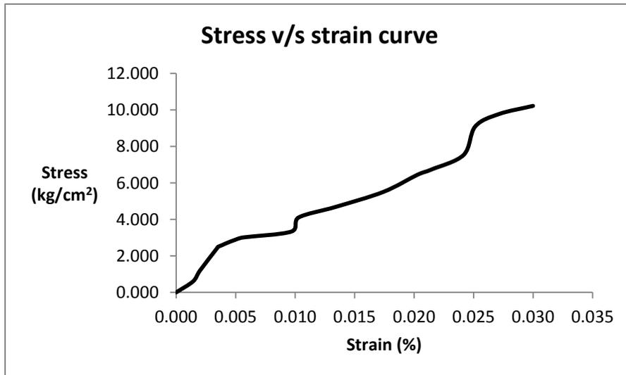
Figure 4.29 - Stress ( $\text{kg/cm}^2$ ) vs strain (%) curve for PM 2
