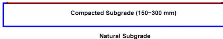
*Figure 3.14 – Layer 1 – Compacted Subgrade course*
