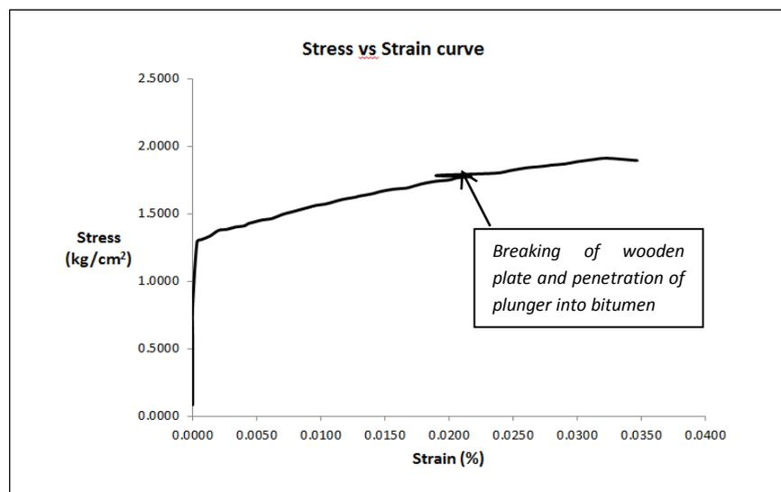
Figure 4.26 – Stress (kg/cm<sup>2</sup>) v/s strain (%) curve for PM 1
