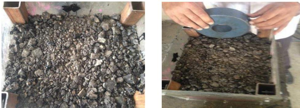
*Figure 3.37 – Surface course and its compaction*
