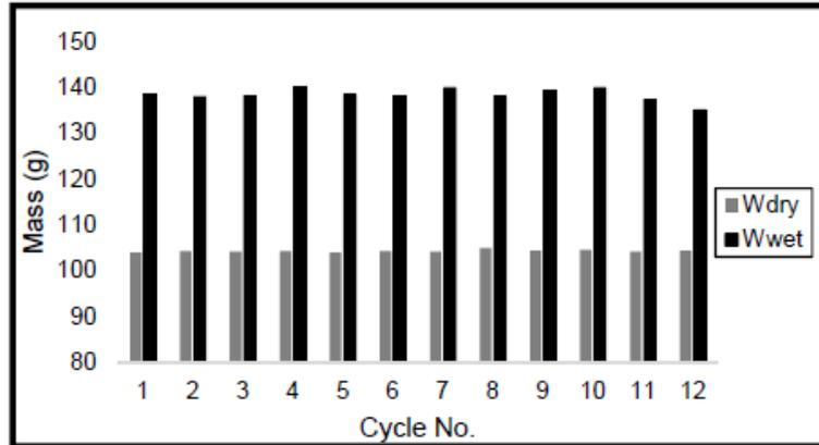
Figure 4.5 - Data of 7 Days Cured sample for Durability Cycles for Gypsum (G)
