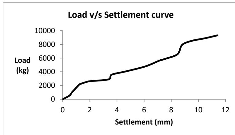
Figure 4.28 – Load v/s settlement curve for PM 2
