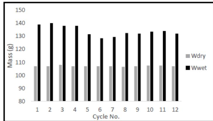
Figure 4.10 – Data of 28 days cured sample for durability cycles for Phosphogypsum (PG)
