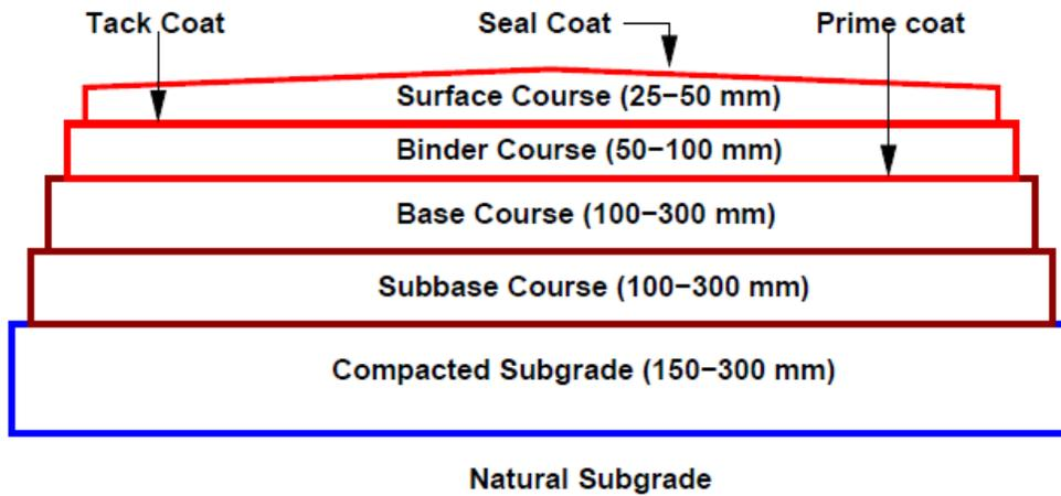
Typical cross section of a flexible pavement
