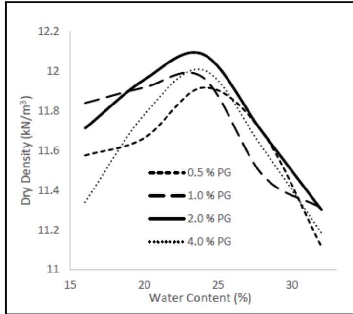
Figure 4.2 (b) – Compaction test plots for fly ash + 8% lime and varying phosphogypsum content
