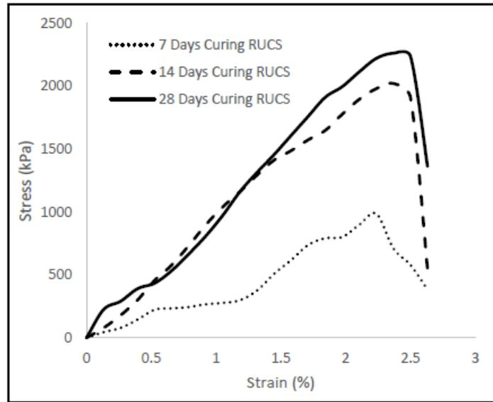
Figure 4.13 – RUCS plots of 7, 14 and 28 days cured samples for Phosphogypsum (PG)
