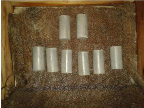
*Figure 3.6 – Burlap curing method for 7, 14 and 28 days sample curing*
