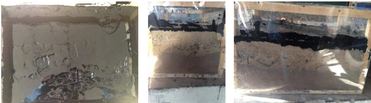
*Figure 3.24 – Seal coat on Layer 5 - Surface course*
