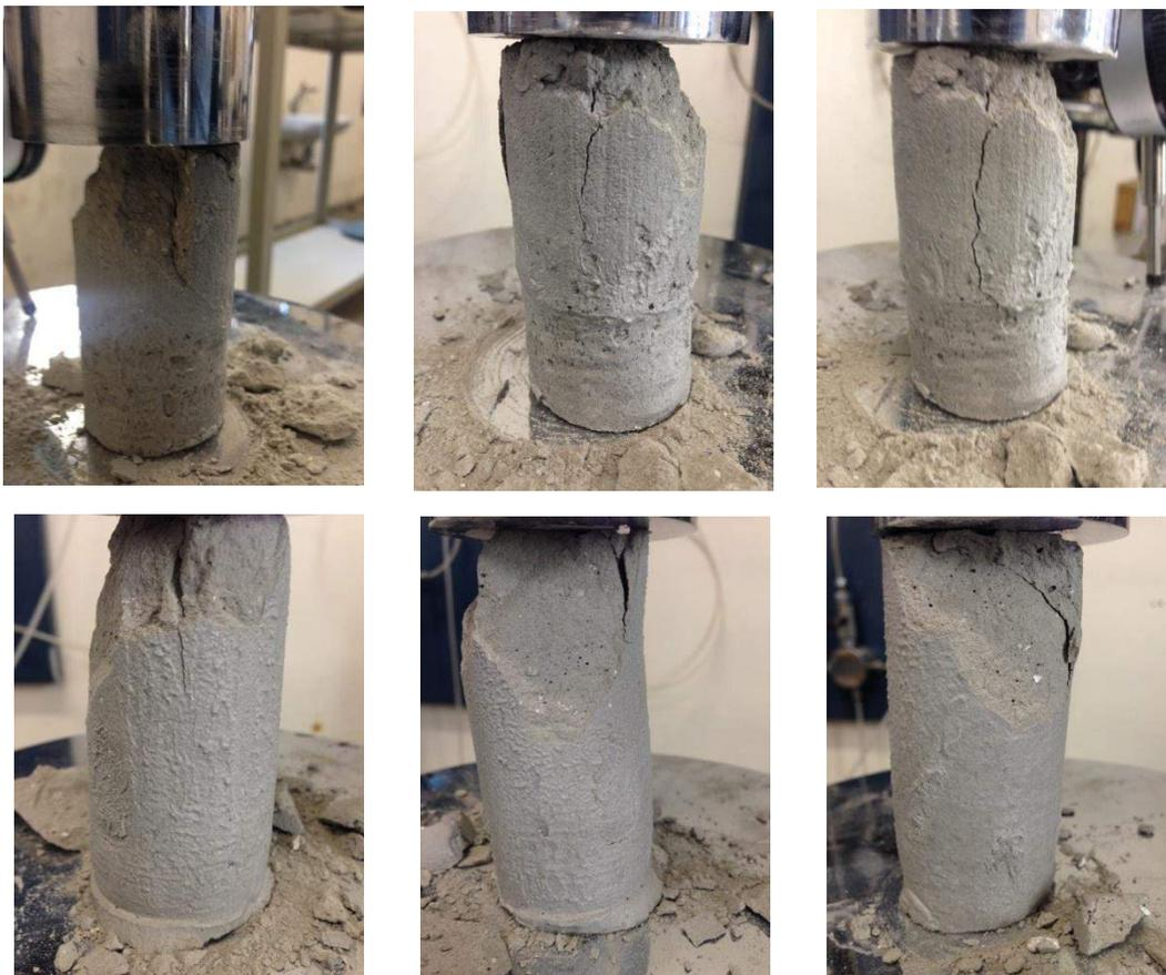
Figure 4.20 (a) – Samples under UCS (top) and RUCS (bottom) for Gypsum (G) modifier
