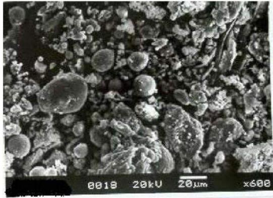
*Figure 4.21 – SEM photograph of Class F Fly Ash (illustrative purpose only)*
