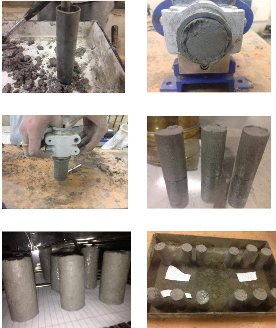
*Figure 3.5 – Sample preparation using compaction mould and sample extractor*
