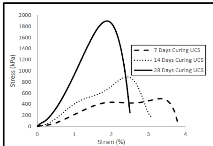
Figure 4.3 – UCS plots of 7, 14 and 28 days cured samples for Gypsum (G)
