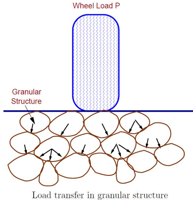
*Figure 3.12 – Grain to grain load transfer/Layer to layer load transfer*
