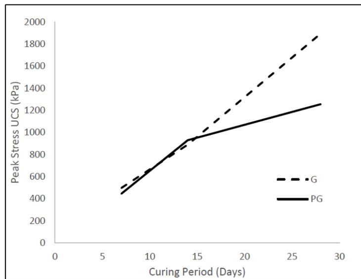
Figure 4.16 – Comparison of UCS over curing time with G and PG
