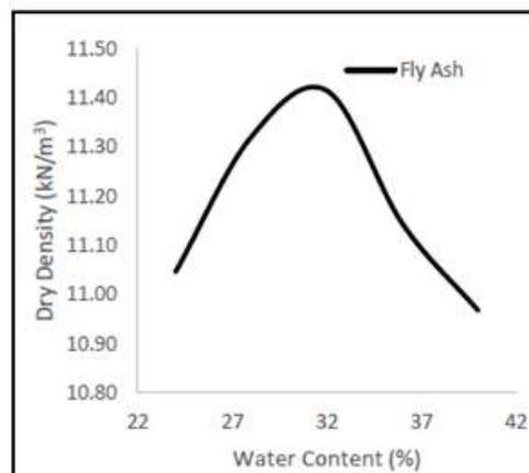
Figure 3.1 – Standard Proctor compaction test results for fly ash
